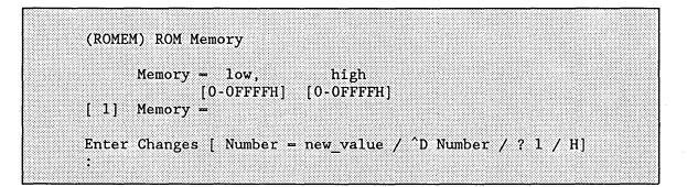
If your application system includes any code burned into ROM, you need to specify the ROM addresses for this code. However, until you are ready to test a PROM-based system in RAM (explained in the *Guide to the iRMX® I Interactive Configuration Utility*) you do not need to use the "ROM" prompt. An example is given in the *Guide to the iRMX® I Interactive Configuration Utility*, you do not need to use the "ROM" prompt.
