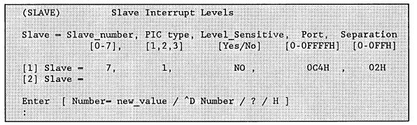
If you need to add an additional interrupt level to those you already specified, enter a new line on the screen using the rules for editing repetitive screens defined in the *Guide to the iRMX® I Interactive Configuration Utility*. See the *Component Data Catalog* for more information on PICs and edge- and level-triggered modes.
