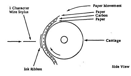
Figure 2-6. Stylus Printer
