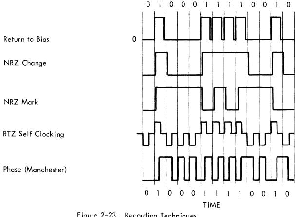
Figure 2-23. Recording Techniques V-2-66
