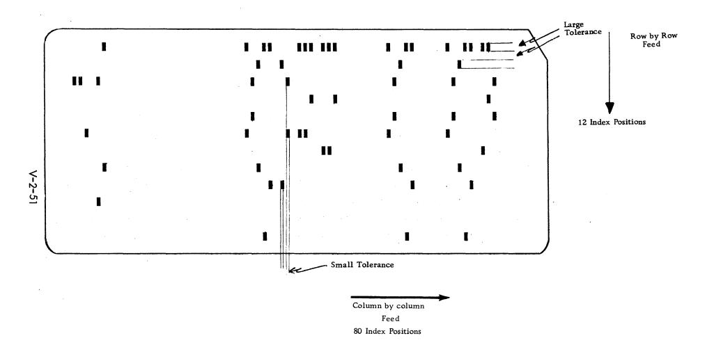
Figure 2-16. Index Positions and Tolerances of Different Feeds
