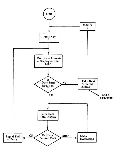
Figure 2–2. Typical Series of Operator Steps in Using Function Keys
