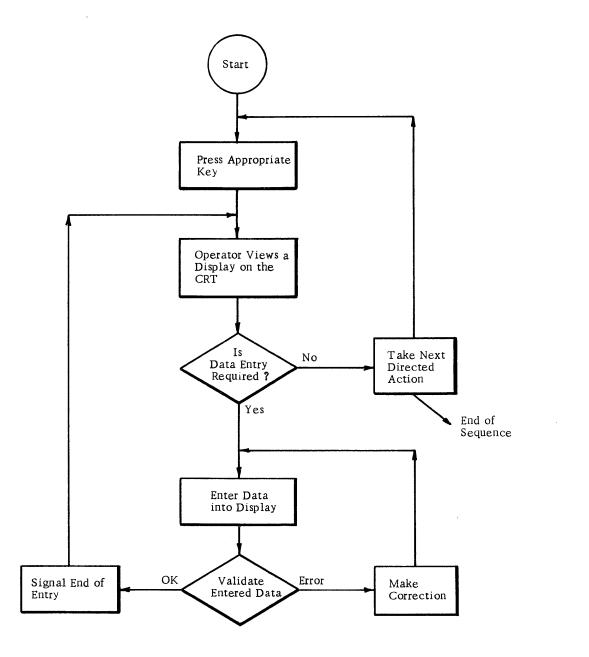
Figure 3-4. Typical On-Line Display Console Operator Procedure
