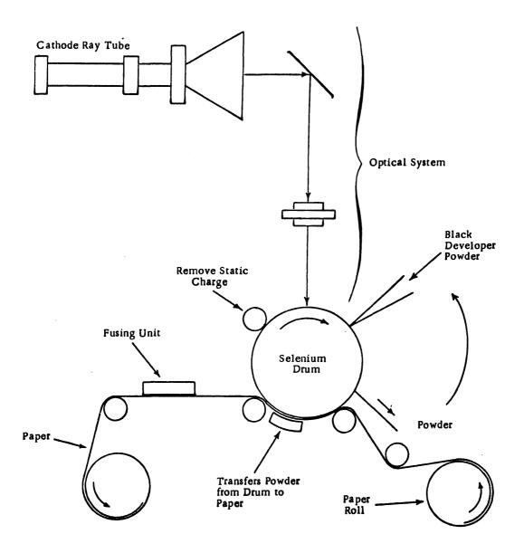
Figure 2-9. Electro-Optical Printer
