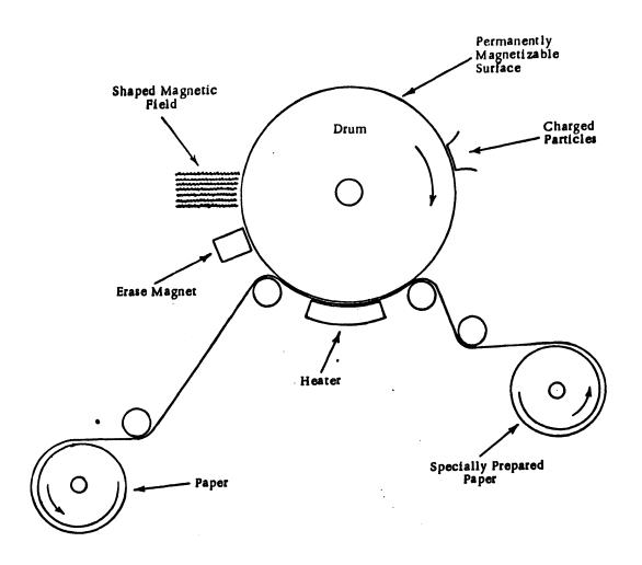
Figure 2-11. Magnetic Printer
