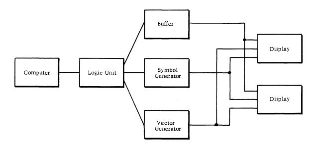
Figure 3-6. Multiple Console with Shared Components
