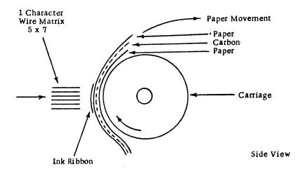
Figure 2-5. Matrix Printer
