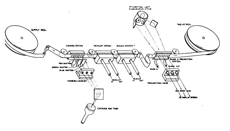
Figure 4-4. Multicolor Film Projection Display System
