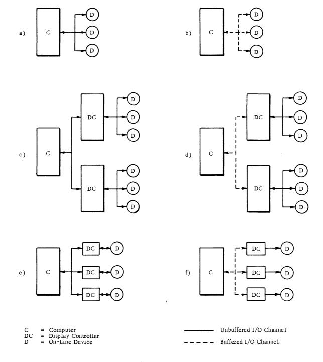
Figure 3-5. Computer/On-Line Device Configurations
