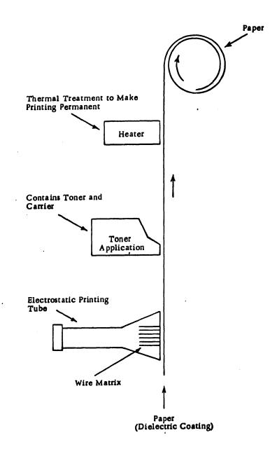
Figure 2-10. Electrographic Printer
