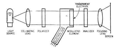
Light path through electro-optic light modulator. Modulating element is between polarizer and analyzer, and is scanned by electron gun at bottom.
