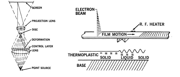
Figure 4–6. A Typical Light Valve Projection System (right) The Principle of Thermoplastic Recording
