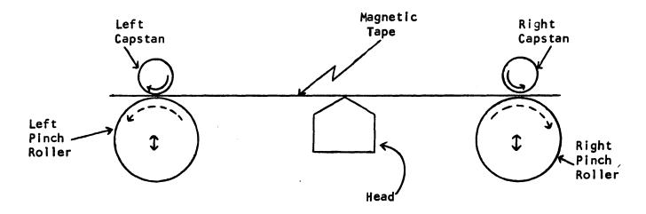
Figure 2-17. Typical Pinch Roller Drive
