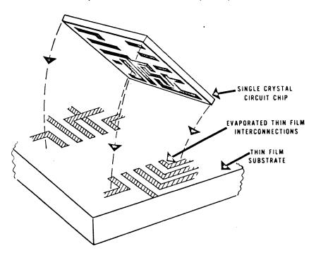
Figure 5-2. Flip-Chip Technique
