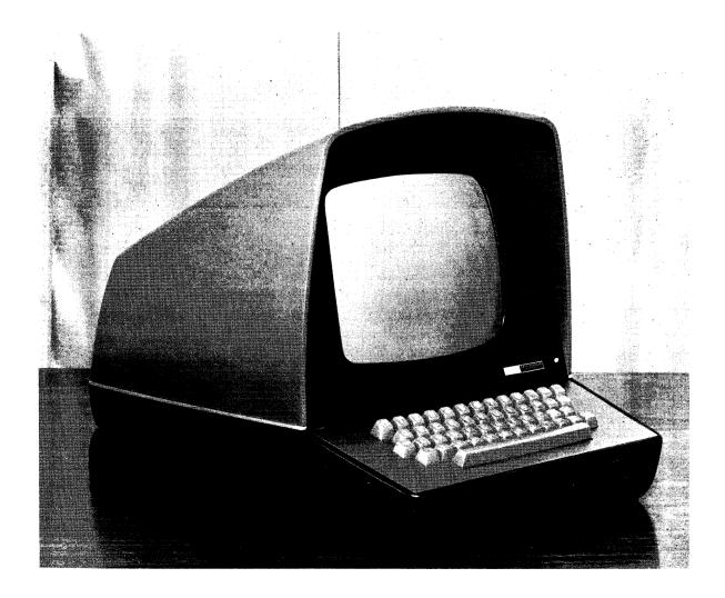
Figure 3–16. Data Display Inc's dd 10 Data Entry and Retrieval Device  User Console - operates like the input console for viewing radar video, IFF and/or computer readouts and is used for command evaluation and decision action entry.
