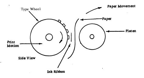
Figure 2-4. Impact Wheel Printer
