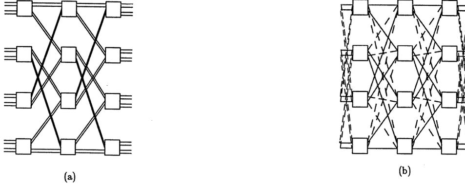
Fig. 2: a) a 2-dilated  $2^3 \times 2^3$  delta network. b) a 2-augmented  $2^3 \times 2^3$  delta network. (Delta networks [22] are a subclass of banyan networks [8]).
