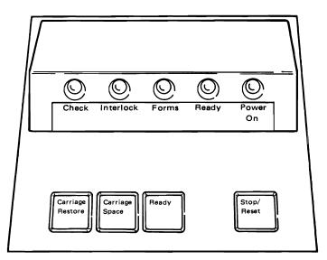
Figure 5-1. 3262 Printer Operator Panel
