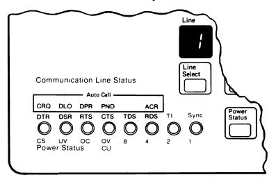
Figure 2-2. Communication Line Status and Power Status Indicators
