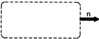
This block shows a procedure passing control for the purposes stated in process n.
