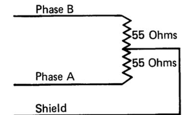
6. Connect the alligator clips **D** to the end of the cable for each combination below. Look at the oscilloscope signal for each combination to determine if a cable failure is present. Use the tables that follow and the sample oscilloscope signals on 70-320 to find any problems that are present.
