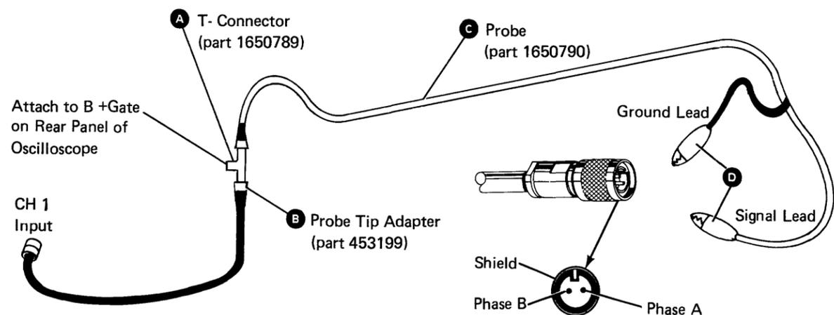
6. Disconnect the cable at the system port. Connect the alligator clips **D** to the end of the cable for each combination below. Look at the oscilloscope signal for each combination to determine if a cable failure is present. Use the tables on the following page and the cabling system sample oscilloscope signals on 70-340 to find any problems that are present.
