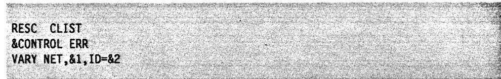
Figure 41. RESC Command List with Parameter Values
