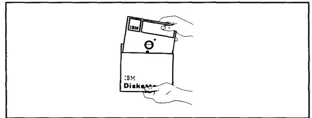
3. Insert the diskette squarely into the diskette unit opening as shown. Make sure that the diskette is completely in the slot, but do not force or bend it. On the 4965 Diskette Storage Unit the label on the diskette faces to the left, and on the 4964 and 4966 diskette units it faces to the right.
