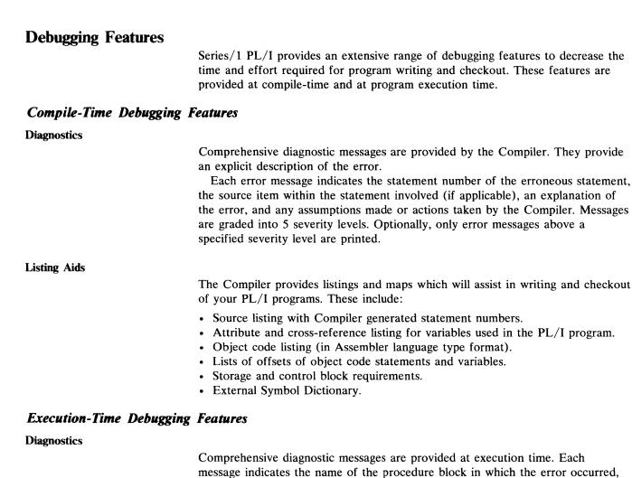
Comprehensive diagnostic messages are provided at execution time. Each message indicates the name of the procedure block in which the error occurred, the offset of the instruction in error, and an explanation of the error. The offset, together with the statement offset list generated by the Compiler allows you to determine the PL/I source statement associated with the error.
