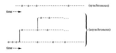
In an asynchronous operation, once a new line has been started, the statements on that line are executed in sequence and independently of the statements on any other line.
