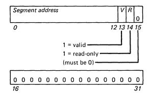
The segment address (bits 0-12) contains the high-order bits of the physical address, which is used by the translator to select a 2K-byte block of main storage.
