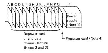
Figure 1-2. IBM Series/1 4956 Model K00 Plugging Assignments
