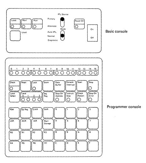
The basic console is intended primarily for those systems that are totally dedicated to a particular application, where operator intervention is not needed during the execution of the application.
