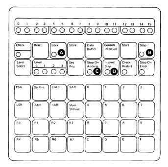
A Lock: Pressing the Lock key first, then pressing four hex keys and the Store key locks the console. A locked console is indicated by an illuminated indicator on the Lock key. The data LEDs are automatically set to the previous value. Displays or alterations cannot be performed with the programmer console keys while in the lock mode. The console remains locked until the same sequence of hex keys that locked the console is repeated and then followed by pressing the Store key.
