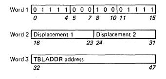
The instruction uses the values of displacement 1, displacement 2, and the address of the first word of the branch table TBLADDR for loading the ARIB instruction work registers, where:
