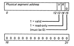
The segment address (bits 0-12) contains the high-order bits of the physical address.
