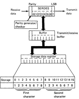
**Note:** The attachment transmits by sending out the low order bit of the byte first. The received characters are stored in the same manner; that is, the first bit received is the low order bit of the byte. If the character is less than 8 bits, it must be right justified. If the data address (DCB word 7) is odd, only one character is moved in or out of storage on the first data transfer.
