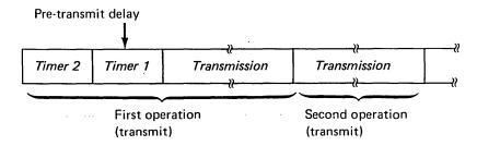
Timer 1 should be set for a pretransmit delay of approximately 9 milliseconds when the receiving station is a program controlled device and is directly connected or is connected through a duplex modem. Timers 1 and 2 should always be activated to prevent excessive turnaround and noise.
