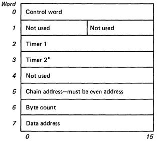
\*Dual function word. In transmit, it contains Timer 2 and PCI information. In receive, it contains only PCI information.
