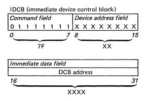
This command does not allow a chaining operation. The byte count in word 6 must be set to 6 and the data address (word 7) must be on a word boundary (bit 15 is set to 0) or an exception interrupt (CC2) occurs with DCB bit 3 (specification check) in the interrupt status byte set to 1.
