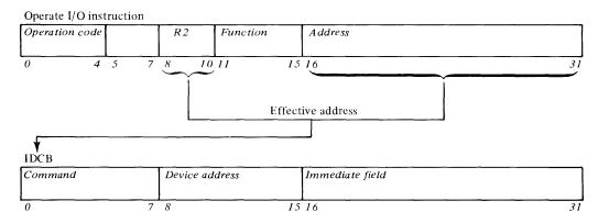
Figure 2-1. Operate I/O instruction and IDCB format
