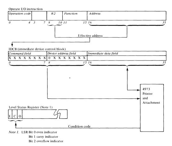
Figure 2-4. Direct Program Control I/O Operation
