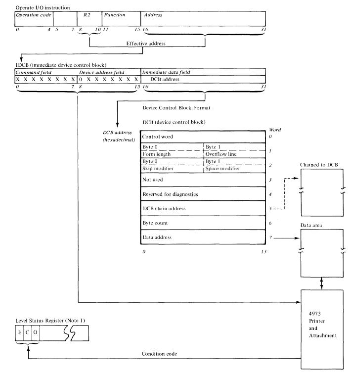
Note 1. LSR Bit 0 even indicator Bit 1 carry indicator Bit 2 overflow indicator
