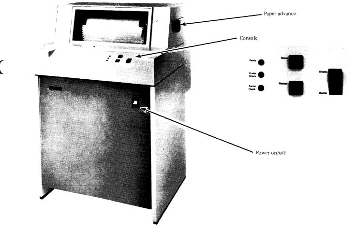
Figure 1-3. Printer Console
