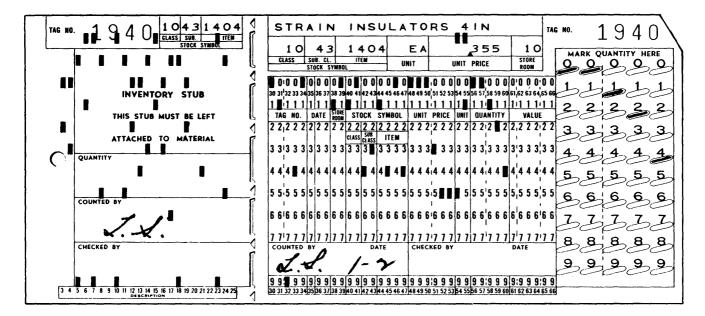
Figure 11. Mark-Sensed Punched Card
