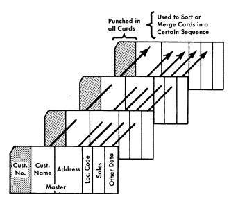
Figure 5. Coding by Gangpunching
