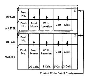
Figure 38. Automatic Coding by Gangpunching
