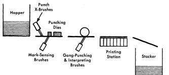
Figure 21. Sketch of Punch Feed with Printing Station
