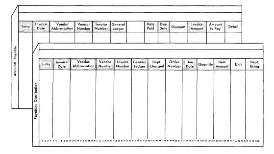
Figure 33. Interspersed-Gangpunching Application
