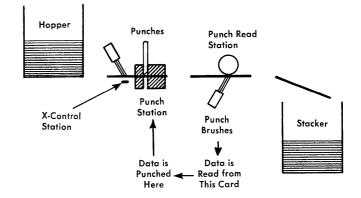
Figure 29. Schematic of Gangpunching
