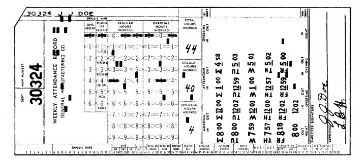
Figure 2. Mark-Sense Punched Card
