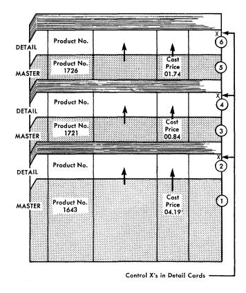
Figure 37. Automatic Pricing by Gangpunching
