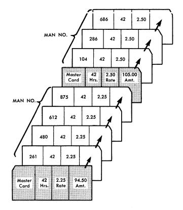
Figure 39. Automatic Extending by Gangpunching
