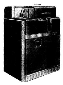
Figure 55. IBM 521 Punching Unit
