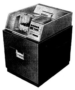
Figure 58. IBM 542 Card Read Punch
