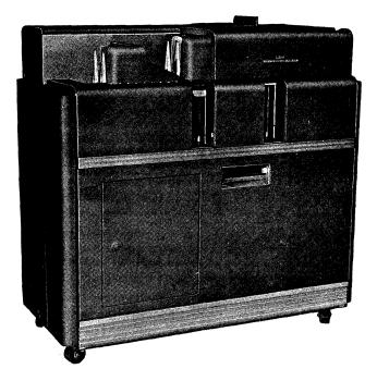
Figure 46. IBM 514 Reproducing Punch
