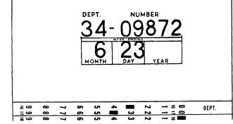
Figure 23. End-Printed Card
