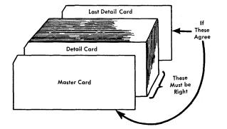
Figure 31. Verification of Gangpunching.
