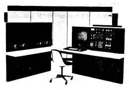
Model 165 ... Large scale scientific and commercial users can achieve substantial throughput gains using IBM's new System/370 Model 165. With an internal power 2 to 5 times that of the System/360 Model 65, it provides fast access through buffered storage using highly efficient algorithms, and concurrent operation. The 165 provides integrated emulation of the 7070, 7080 and 7090.
