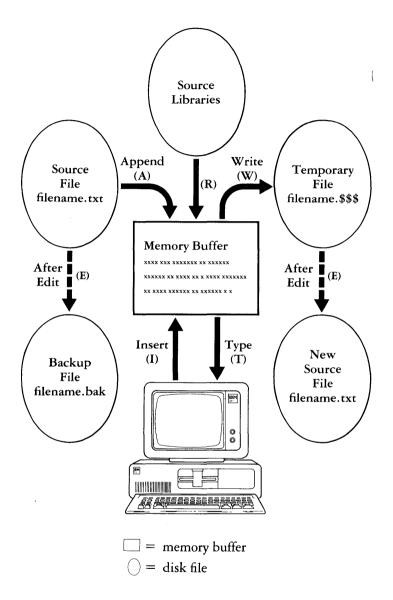
In the figure above, the memory buffer is logically between the source file and the temporary work file. ED supports several commands that transfer lines of text between the source file, the memory buffer and the temporary, and eventually final, file. The following table lists the three basic text transfer commands that allow you to easily enter the editor, write text to the temporary file, and exit the editor.
