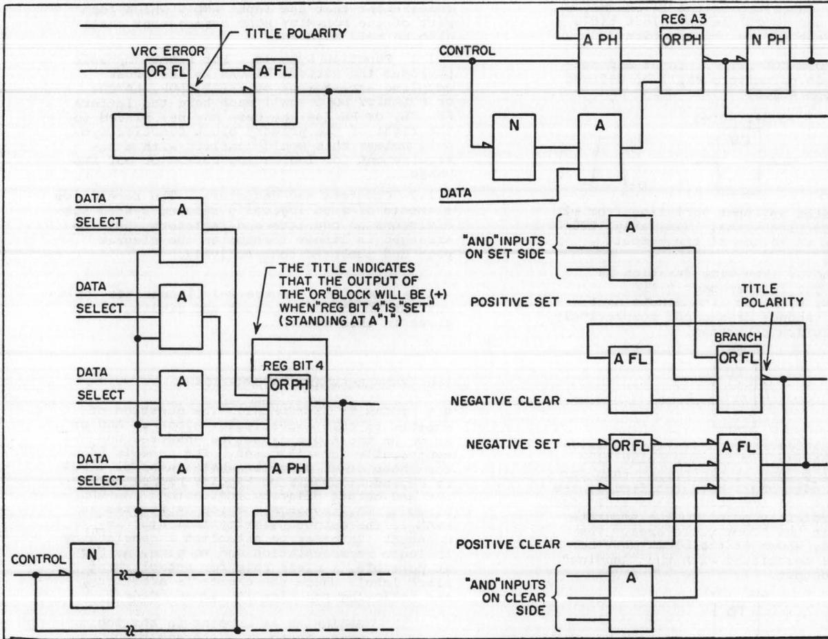
FIGURE 2-2. EXAMPLES OF MULTIPLE BLOCK STORAGE ELEMENTS
