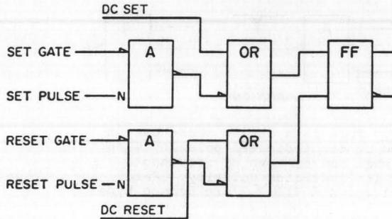
**FLIP FLOP WITH INPUT AND'S AND OR'S**
