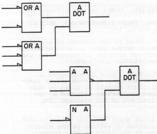
4.1.17.1 **Wired Logic.** When the output of a block enters into both a DOT OR and a DOT AND operation the letters WL (for WIRED LOGIC) shall be placed to the right of the primary block function symbol.
