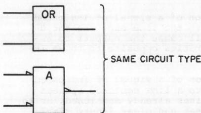
4.1.2.2 **Positive OR INVERT.** The output of the positive OR INVERT is in its more negative condition when and only when one or more of the inputs are in their more positive condition.
