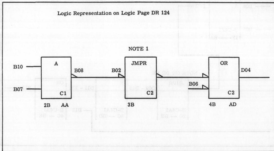
FIGURE 2-8. JUMPER NOT ASSOCIATED WITH EXTERNAL PINS
