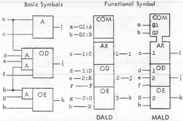
Common Section: A line common to all logic elements shall be drawn to the common section of the logic symbol and shall be identified as described in the paragraph under FLIP-FLOPS as applicable. Gating lines common to one or more storage elements should also be drawn to the Common Section. The top line of the common section may contain the letters "REG".
