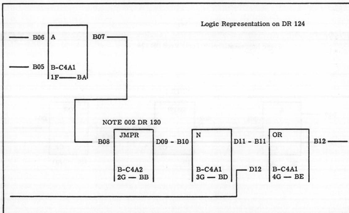
FIGURE 2-6. FEATURE INCORPORATED WITH JUMPER
