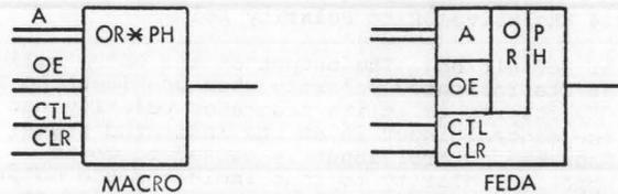
NOTE: In this representation it is necessary to establish the control (CTL) input, and if used the clear (CLR) input.
