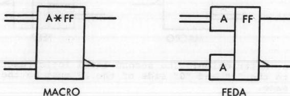
2.2.3 Suffixes: DOT, FL, PH or others as specified in CES 0-1046-3 shall be used where ever possible. When the number of characters in the Macro function prohibits this, due to space requirements, the suffix will be omitted from the logic block. However, where ever possible the omitted suffix shall be carried in the block title as follows.
