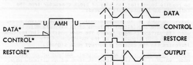
5.3 ANALOG OR. The amplitude of the output signal will stand at a value corresponding to that of the input signal having the greatest amplitude in the direction shown by the line input edge of block character, which must be the same for all inputs. The inputs must be in the same signal mode as the output. The output mode may be indicated by the suffix, I or V (see Paragraph 4.1).
