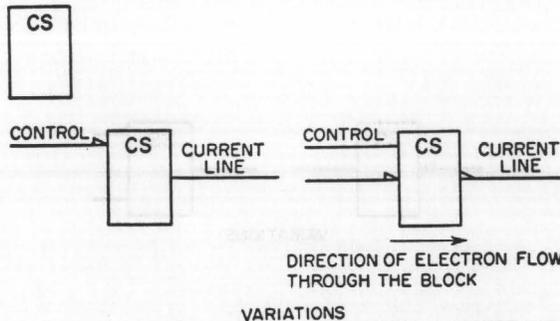
4.1.18.1 **Example of Use.** The illustration (Figure 2-1) shows the use of the SERIES CURRENT SWITCH (CS) to control a series flow of current through more than one circuit.
