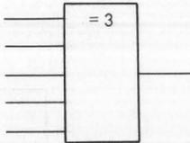
FIGURE 2-21. TYPICAL M AND ONLY M SYMBOL
