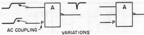
4.1.2 **OR.** This is a device whose output will stand at its indicated polarity when and only when one or more of its inputs stands at its indicated polarity. Paragraphs 4.1.2.1 and 4.1.2.2 are common types.
