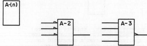
**4.1.12 ODD COUNT.** This is a device whose output will be at its indicated polarity when and only when an odd number (1-3-5-7, etc.) of its inputs are at their indicated polarity. An ODD may be shown as an EVEN through proper change in polarity indication.
