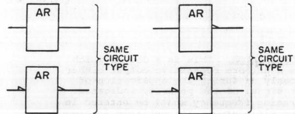
4.1.4.1 **Non-Standard Logic Signal Voltage.** An AMPLIFIER having input or output of other than standard logic signal voltage shall be made recognizable through labeling at the block.
