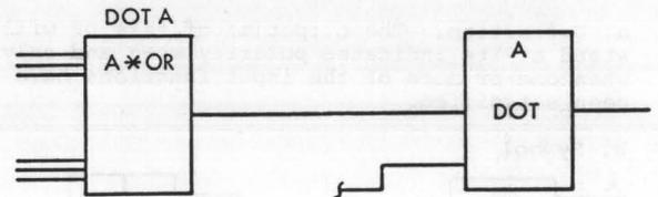
CAUTION: When the DOT suffix is not in line one of the logic block, the DA program will not check the suffix and will produce suffix errata, however, DOT wiring rules are checked.
