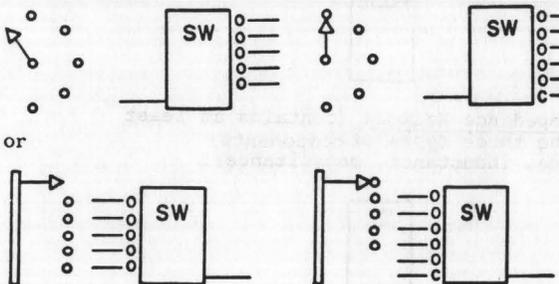
(e) When a pole is to make electrical connection with more than one other point at a time, the pole is to be shown as contacting each of the other points.
