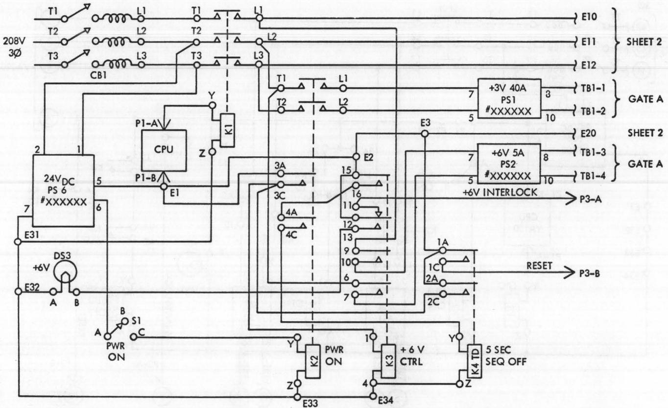
FIGURE 4-3. WIRING DIAGRAM, POWER SYSTEM
