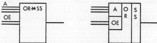
2.3.4 Delineator; Shall be used with two level symmetrical macros. When the Advanced D.A. program is operational an "\*" asterisk will be inserted in the space reserved between functional groupings automatically. The asterisk shall also be used to separate the "1" and "0" areas of a two and three level FF, also the Data, control, and clear inputs to the two level PH.
