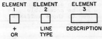
5.1.1 Element 1. The + or - symbol in element 1 refers solely to the relative level of the signal line with respect to its title. For example, the + symbol indicates that for the title condition, the line will stand at the more positive of its two possible states. The + or - symbol should generally match the output polarity indication shown on the source block.
