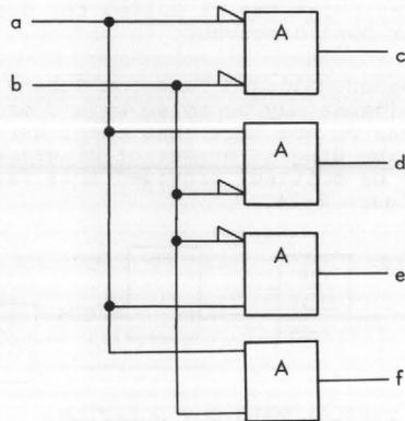
B. DECODER WITH BINARY CODED OUTPUTS
