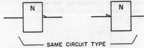
4.1.4 **AMPLIFIER.** This is a device whose fundamental purpose is to provide adequate driving energy and appropriate impedance matching to other devices. Its output will be at its indicated polarity when and only when its input is at its indicated polarity.
