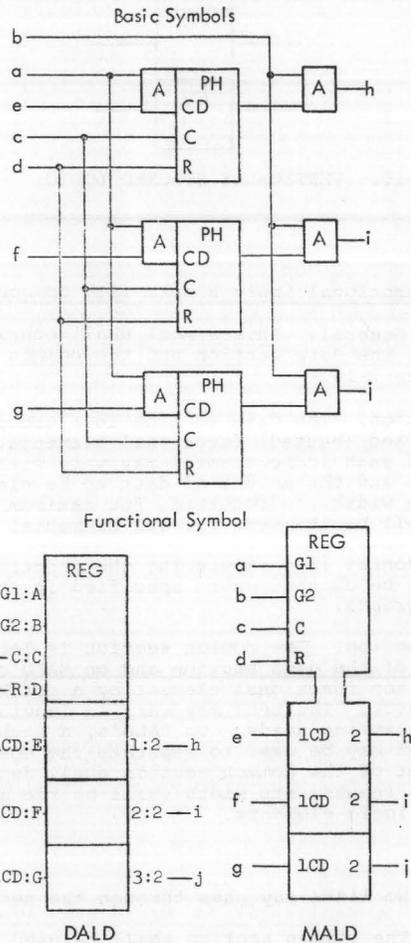
FIGURE 2-19. REGISTER FUNCTIONAL SYMBOL.
