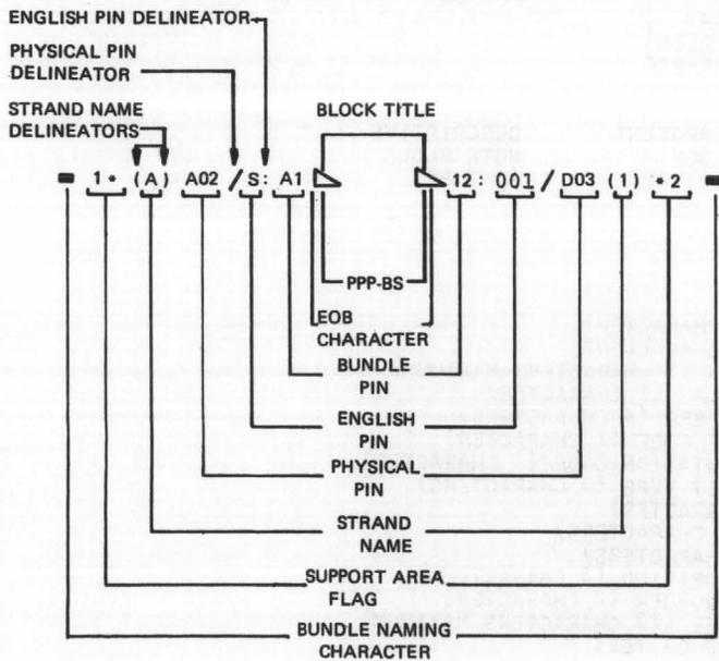
FIGURE 2-27. BLOCK PERIPHERARY NOTATION
