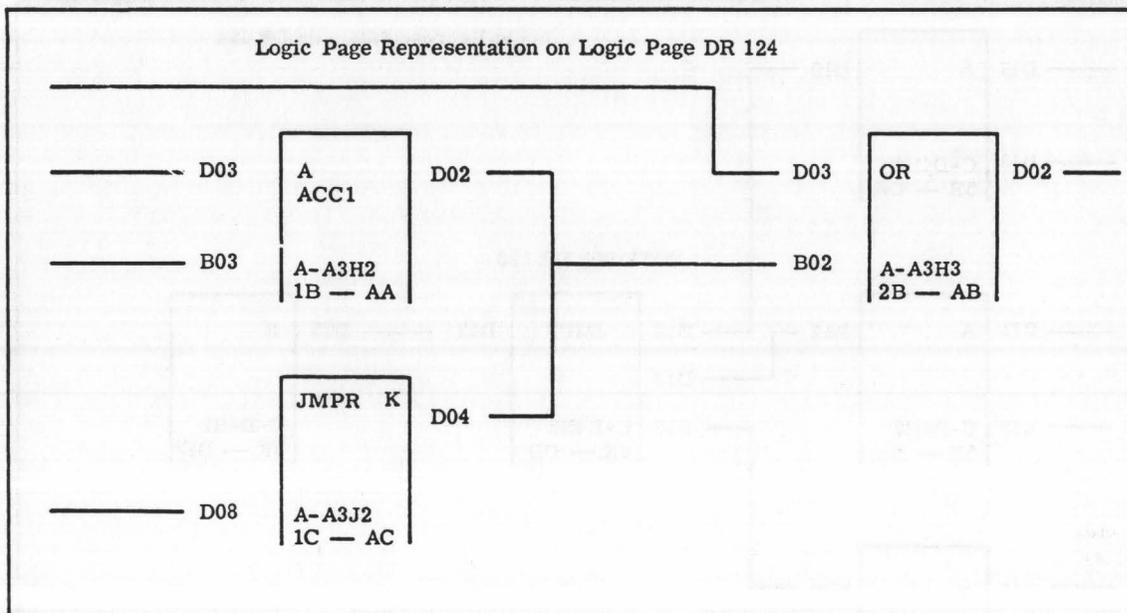
FIGURE 2-5. JUMPER USED TO STABILIZE FUNCTIONS
