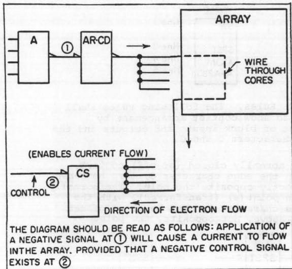
FIGURE 2-1. USE OF SERIES CURRENT SWITCH
