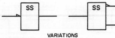
**4.1.11 THRESHOLD.** This is a device whose output will be at its indicated polarity when and only when the number of its inputs which stand at their indicated polarity reaches or exceeds the number specified in the function symbol. This symbol shall also be used where an input may have greater
