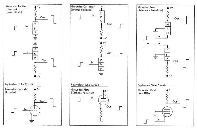
Figure 2. Transistor Circuit Configurations
