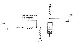
Figure 20. Logical Low Power Inverter
