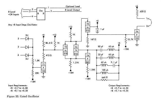
the R-C-L network. When T2 cut off, however, the T4 base went negative, causing T4 to reduce its conduction. The reduced current of T4 was a sudden current decrease through the R-C-L network. This network responds by providing a negative voltage shift to the T3 base after a time interval determined by the components of the network.
