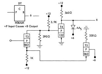
Figure 62. Current Switching to DDTL Converters
