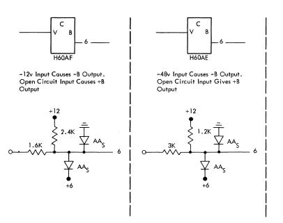
Figure 64. V to B Converters
