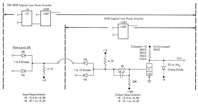
Figure 30. AND Logical Low Power Inverter
