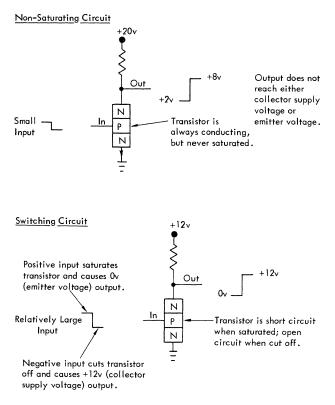
Figure 4. Transistor Operating Modes
