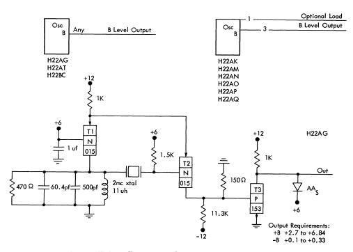
Figure 53. Crystal-Controlled Oscillator, Example 1
