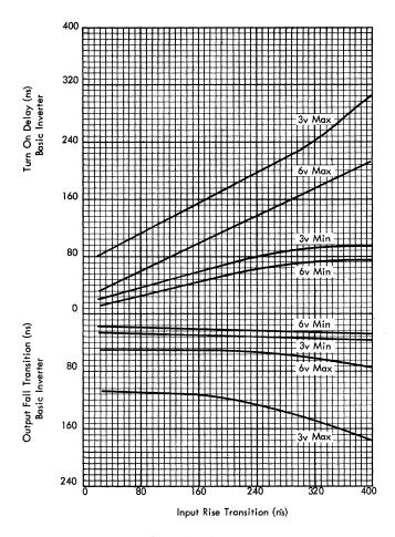
Figure 82. Turn-On Delay and Fall Transition of Basic Inverter
