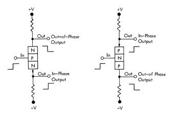
Figure 3. Split-Load Configuration
