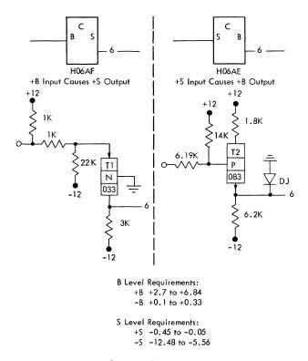
Figure 63. B to S and S to B Converters
