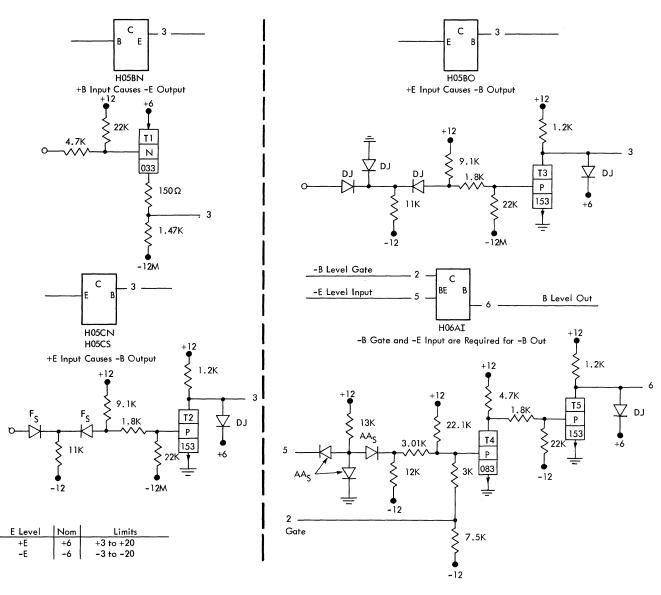
Figure 60. B to E and E to B Converters
