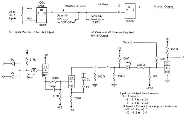
Figure 56. Line Driver and Line Terminator
