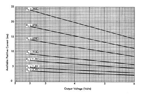
Figure 95. Available Positive Current from a Basic Inverter
