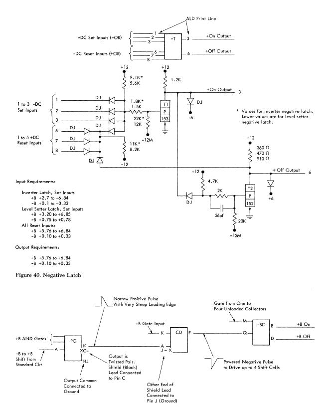
Figure 41. Shift Cell Circuits
