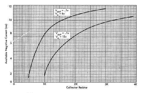
Figure 94. Available Negative Current from a Basic Inverter
