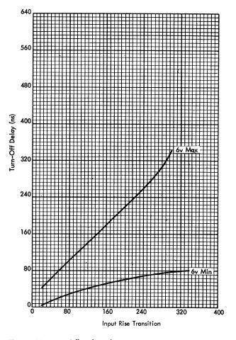
Figure 99. Turn-Off Delay of AND LLPI
