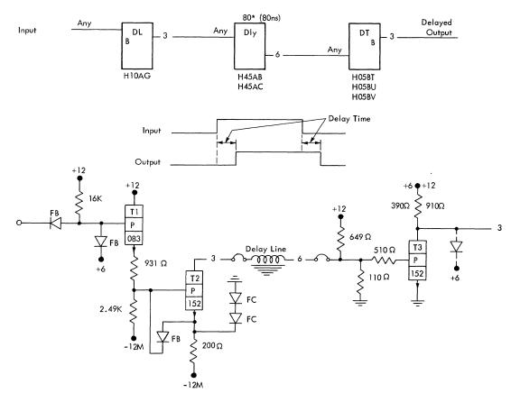
Figure 57. Delay Line Driver and Terminator
