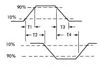
T1 = Rise Transition (Turn – On) T2 = Turn – On Delay T3 = Fall Transition (Turn – Off) T4 = Turn – Off Delay
