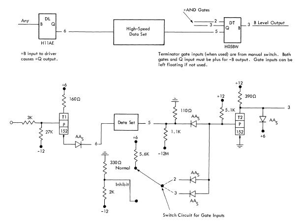
Figure 59. V or Q Level Data Set Driver and Terminator
