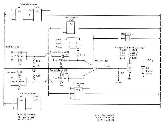
Figure 28. Basic Inverter with Diode Logic
