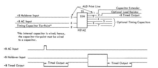
If holdover input is +B, output is -B. When the holdover input goes to -B, output remains minus for time duration of SS. Only if the holdover input is -B, can the AC input fire the SS.
