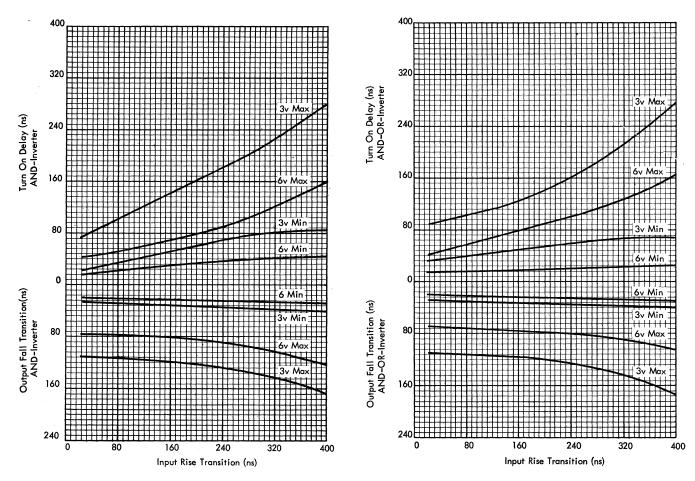
Figure 84. Turn-On Delay and Fall Transition of AND Inverter
