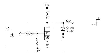
Figure 17. Basic Inverter with Clamped Output
