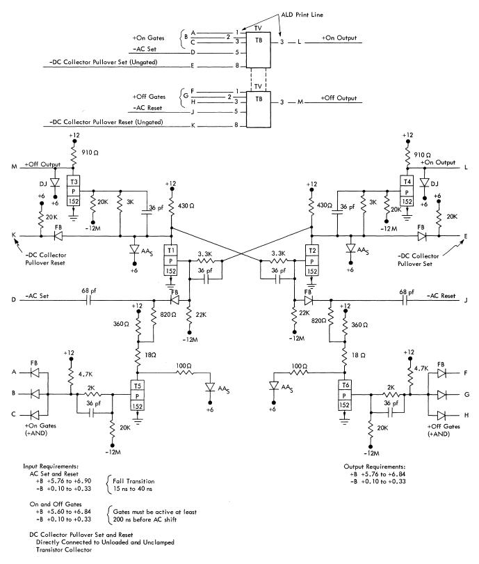
Figure 39. AC Trigger
