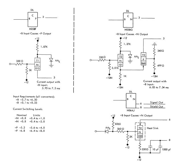
Figure 61. DDTL to Current Switching Converters
