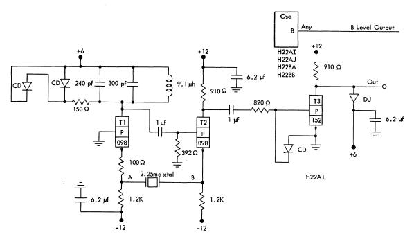
Figure 54. Crystal-Controlled Oscillator, Example 2
