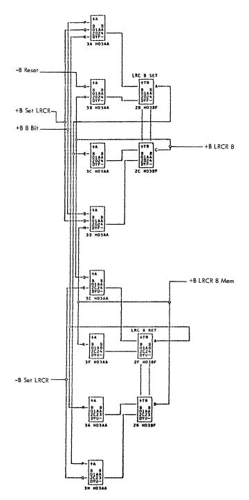
Figure 75. Latch Configuration for Binary Operation
