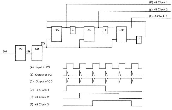
Figure 42. Shift Cell Clock Ring
