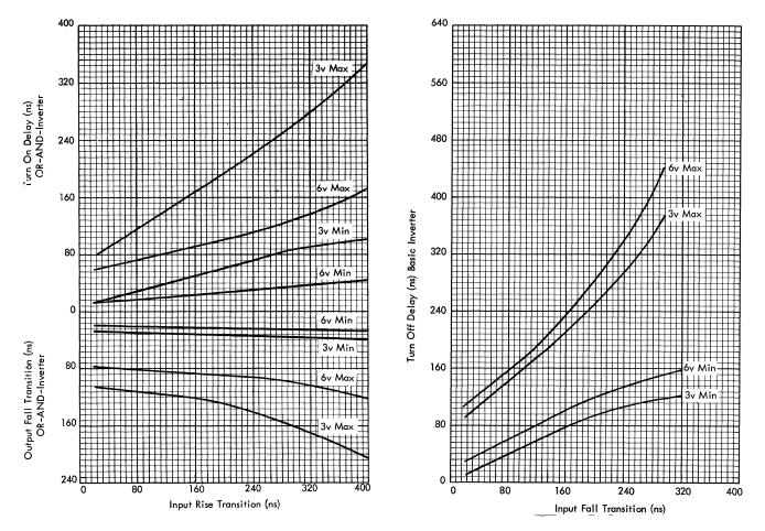
Figure 86. Turn-On Delay and Fall Transition of OR-AND Inverter Figure 87. Turn-Off Delay of Basic Inverter
