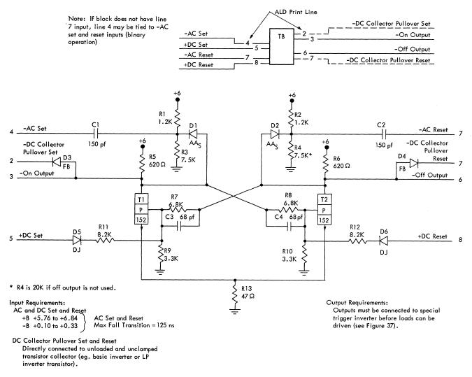
Figure 36. Binary Trigger
