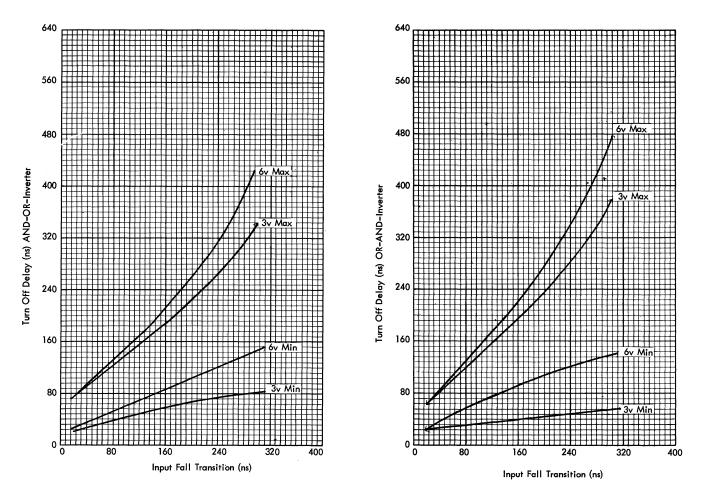
Figure 90. Turn-Off Delay of AND-OR Inverter
