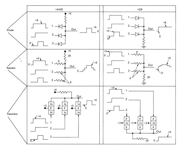
Figure 5. Logic-Performing Circuits
