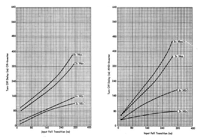
Figure 88. Turn-Off Delay of OR Inverter
