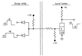
Figure 23. Level Setting Circuit
