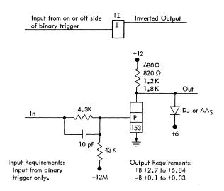
Figure 37. Binary Trigger Inverter
