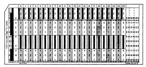
Figure 17. IBM card - column binary
