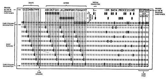
Figure 15. IBM card - standard card code
