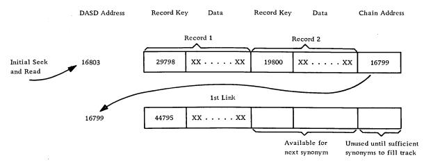
Figure 12. Example of chaining, blocked records
