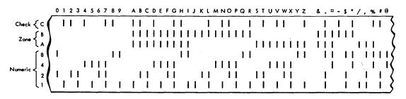
Figure 18. Magnetic tape - six-bit alphameric code
