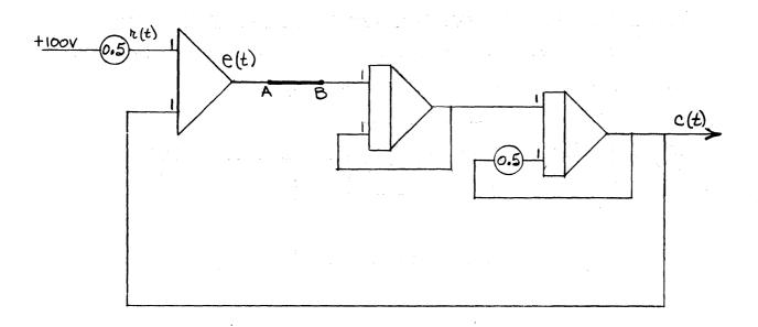
Figure 6. Analog model of a Type 0 system.
