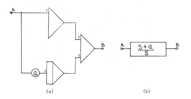
Figure 9. Analog model of integral-error compensation.
