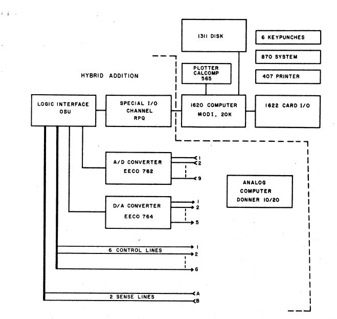
Figure 1. Block diagram of OSU computing system.
