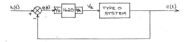
Figure 10. The analog system with the digital computer in the loop.
