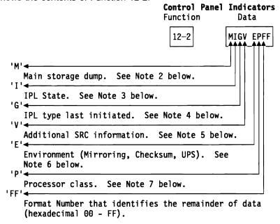
Figure 4-11. Structure of Fixed Data in Function 12-2 Notes:
