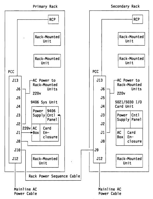
Figure 7-9. Stage 1 Power Distribution. The 9406 Stage 1 system uses the distributed power concept.
