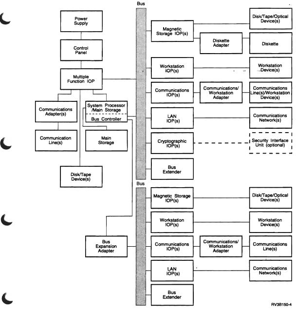
Figure 7-11. Example - 9406 Model F95 logic diagram
