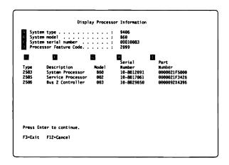
Figure 1-32. Example of Display Processor Information Display
