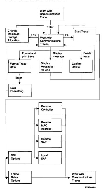
Figure 1-21. Work with Communications Trace Menu Flow
