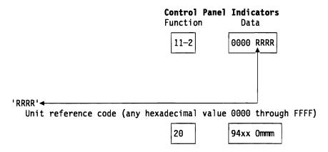
Figure 4-8. Example of Stage 2 Control Panel SRC records
