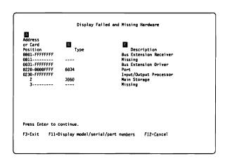
Figure 1-33. Example of Display Failed and Missing Hardware Display
