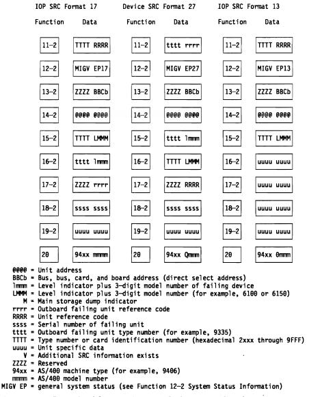
Figure 4-7. Example of Stage 2 Hardware SRC records. This figure represents three SRC record formats; other formats exist.
