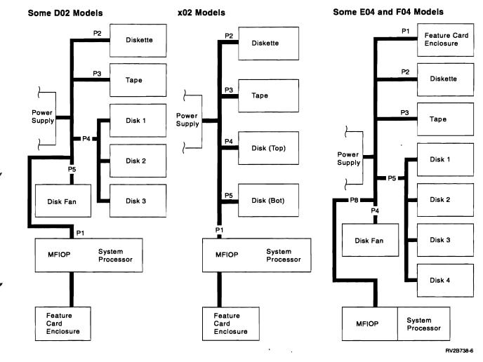
Figure 7-6. 9402 System Power Distribution (2 of 3). The 9402 Power Distribution Diagram shows the FRUs that receive dc voltages from the central power supply.
