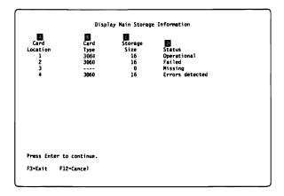
Figure 1-31. Example of Display Main Storage Information Display
