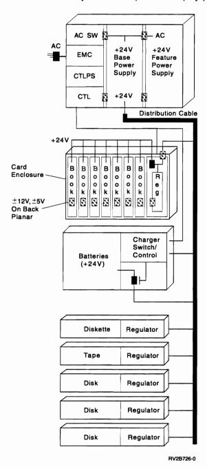
Figure 7-8. 9404 System Power Distribution
