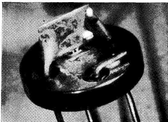
Figure 3 Two views of the microwave oscillator mounted on conventional header. (Unit at left magnified 6.6\times .)
