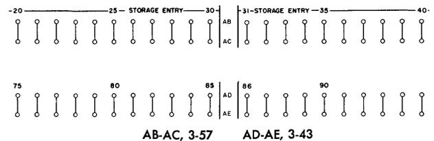
These 96 pairs of hubs are normally wired from the third reading brushes to enter data. They correspond to the 96 positions in the row buffer, which is a special synchronizer used for temporary storage. The words to be entered (as indicated by word size wiring) must be wired to these hubs in numerical sequence by word number.
