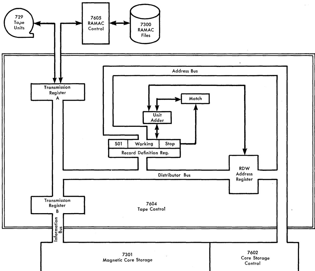
FIGURE 104. CHANNEL CONTROLS 1 AND 2 SCHEMATIC
