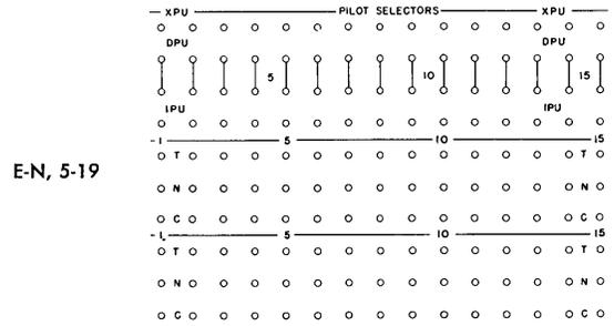
PILOT SELECTOR PICKUPS. Three types of pilot selector pickups are provided.
