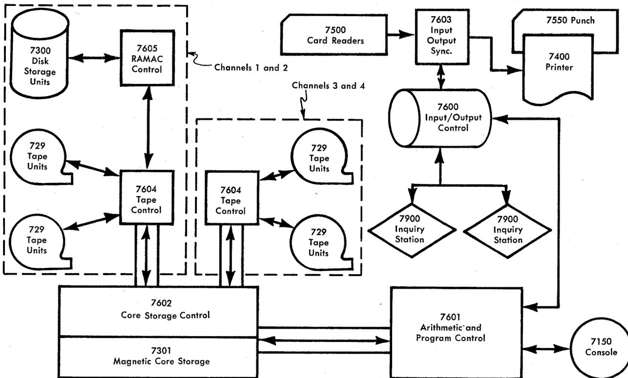
FIGURE 4. SCHEMATIC OF 7070 COMPONENTS
