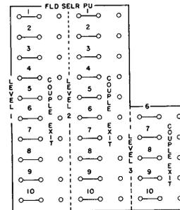
**FIELD SELECTOR PICKUP LEVELS 1, 2, AND 3:** These hubs are used to impulse the corresponding level of a field selector to transfer on the following read feed cycle. They are entries for any read-timed digit impulses (9-12) and are wired from first reading to cause the selector to transfer when that card passes second reading, or from second reading to transfer the selector for third reading.
