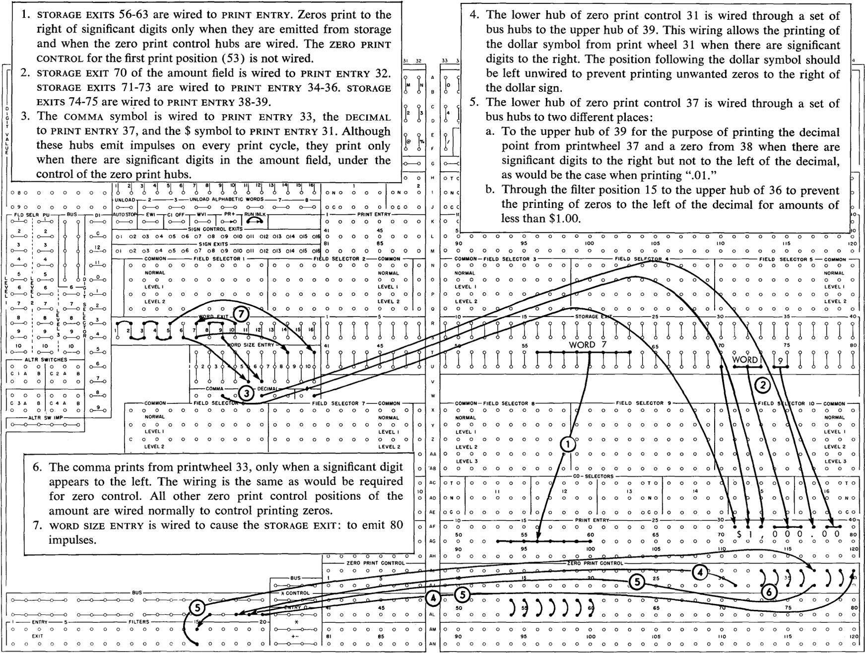
1. STORAGE EXITS 56-63 are wired to PRINT ENTRY. Zeros print to the right of significant digits only when they are emitted from storage and when the zero print control hubs are wired. The ZERO PRINT CONTROL for the first print position (53) is not wired.
