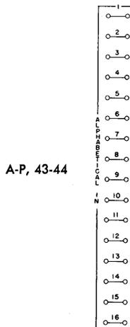
**ALPHABETICAL IN:** These hubs are normally wired from the CAI hubs to activate the necessary translating circuitry for alphabetic conversion in the 7070. The combination zone and digit punches in the card are converted to the 2-digit representation used to store alphabetic information. Impulsing this hub also causes an alphabetic sign to be entered into the sign position of the designated word.
