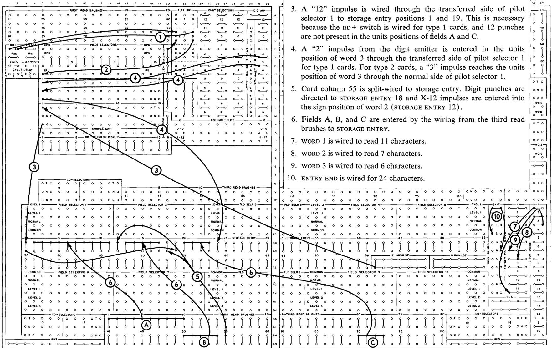
1. The RD+ switch is connected for type 1 cards through the B side of alteration switch selector 2. For type 2 cards the switch is unwired.
