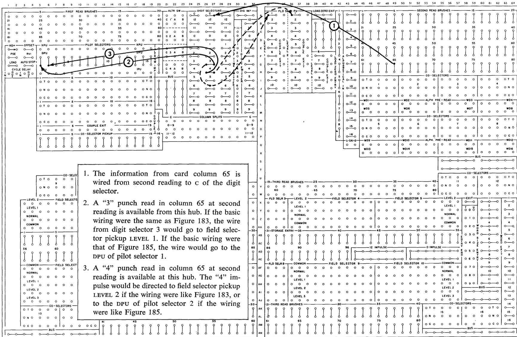
1. The information from card column 65 is wired from second reading to c of the digit selector.
