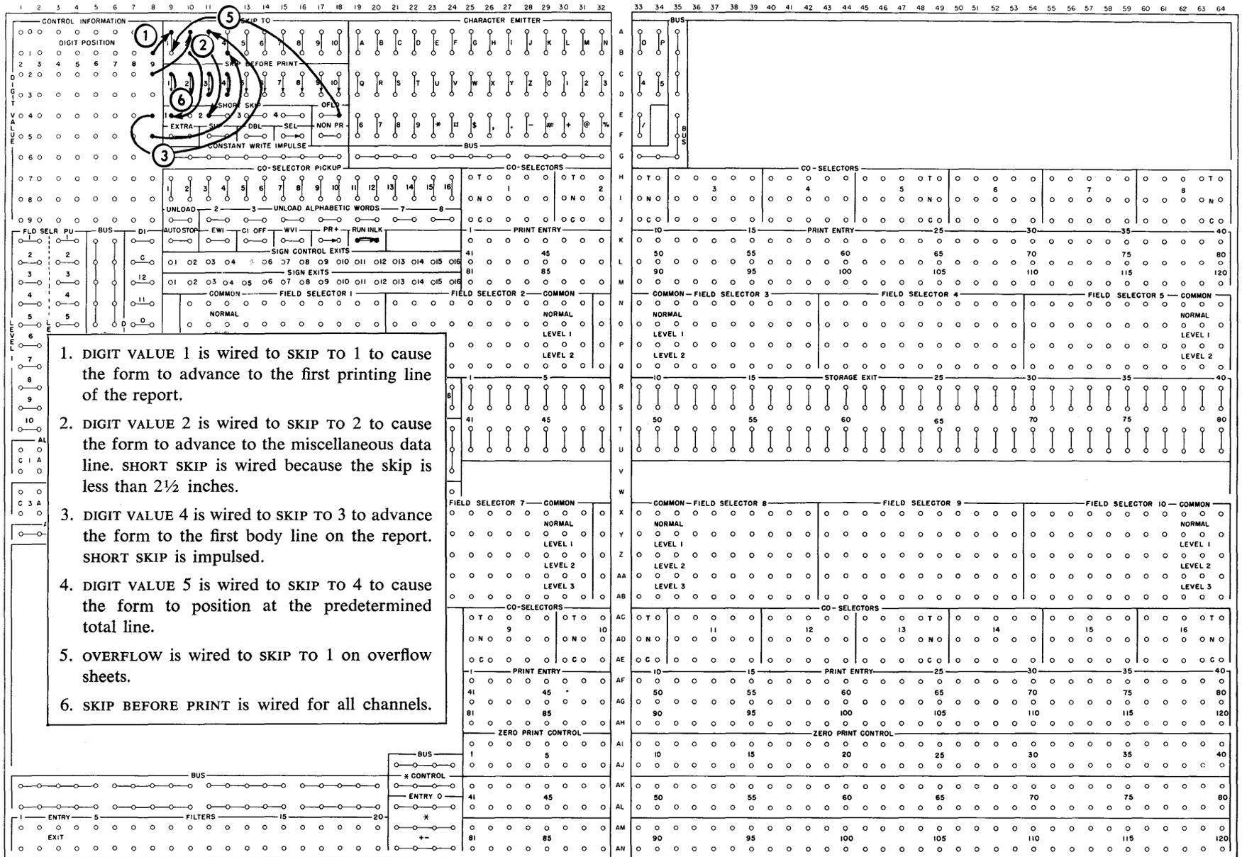
1. DIGIT VALUE 1 is wired to SKIP TO 1 to cause the form to advance to the first printing line of the report.
