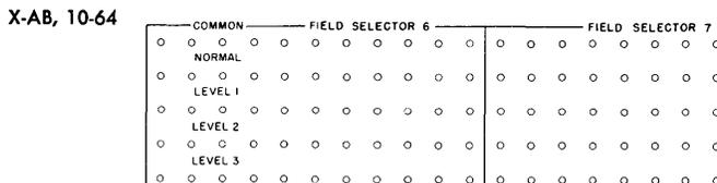
FIELD SELECTOR LEVELS 1, 2, AND 3—NORMAL AND COMMON: There are ten 11-position field selectors provided. Field selectors 1-5 have three levels each (*normal, level 1 and level 2*); selectors 6-10 have 4 levels each (*normal, level 1, level 2, and level 3*). *Note:* The vertical arrangement of the four level field selectors 6-10 is the same as that of the three level field selectors 1-5.
