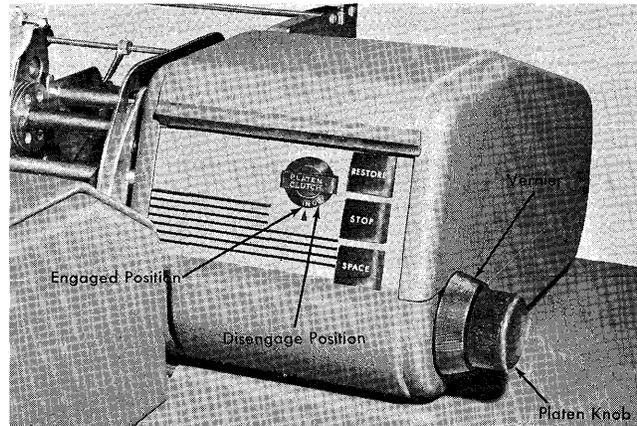
FIGURE 235. PLATEN CLUTCH
