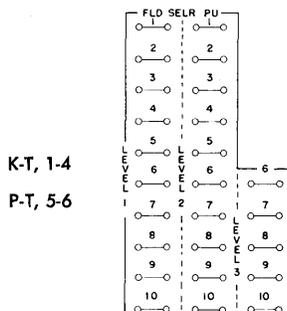
FIELD SELECTORS PICKUP LEVELS 1, 2, AND 3: These hubs, when impulsed, cause the corresponding level of a field selector to transfer on the same print cycle. They are normally wired from CONTROL INFORMATION. An impulse to these hubs causes the field selectors to transfer immediately and remain transferred for the duration of that print cycle.
