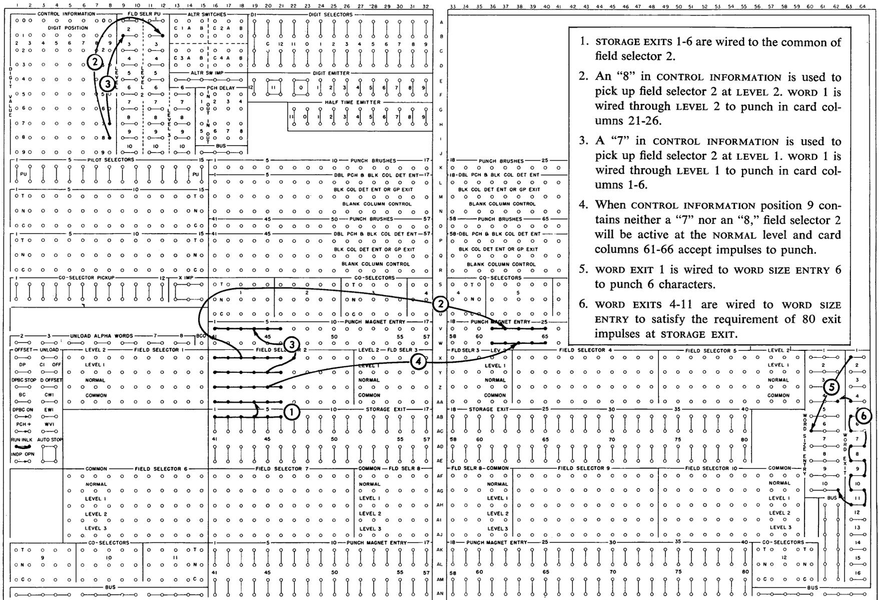
1. STORAGE EXITS 1-6 are wired to the common of field selector 2.
