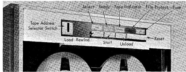
FIGURE 128. IBM 729 TAPE UNIT OPERATING KEYS AND LIGHTS
