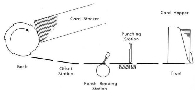
FIGURE 193. 7550 PUNCH SCHEMATIC
