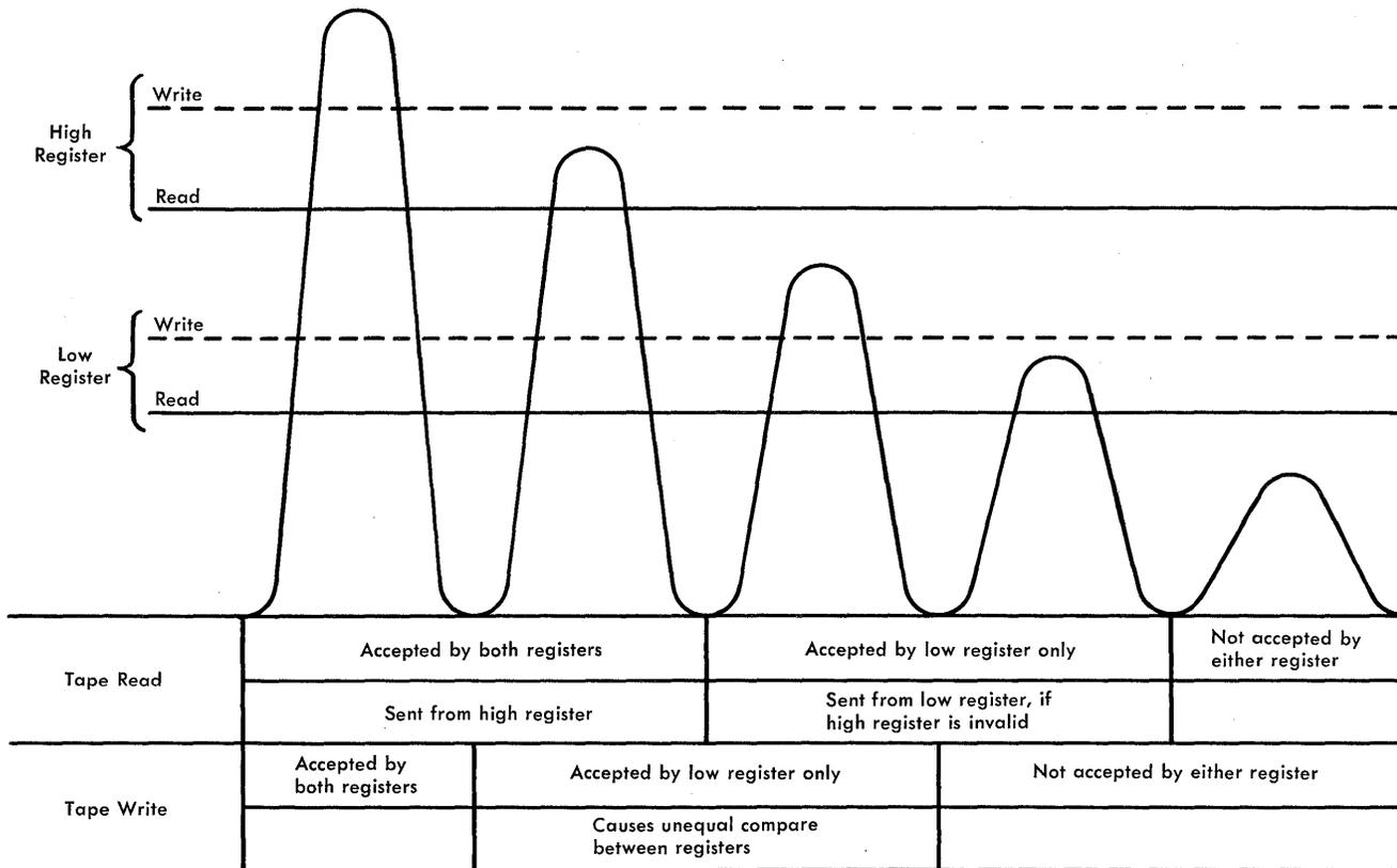
FIGURE 124. DUAL-LEVEL SENSING
