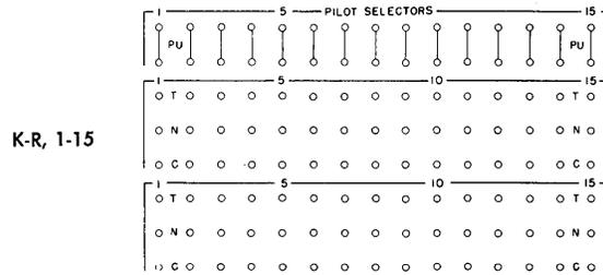
**PILOT SELECTORS:** Fifteen 2-position pilot selectors are provided. Each position has three points, C (Common), N (Normal), and T (Transferred). When a pilot selector is transferred, there is an internal common connection between C and T. When it has not been impulsed to pick up, an internal common connection exists between the C and N hubs.
