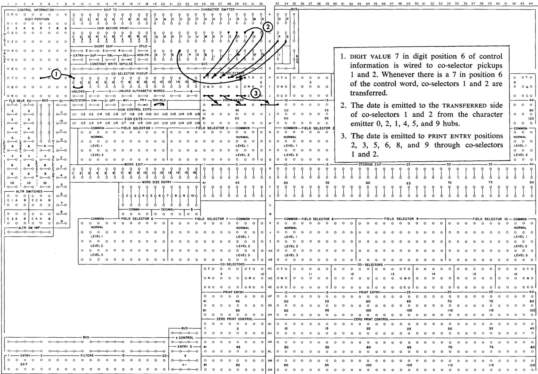
1. DIGIT VALUE 7 in digit position 6 of control information is wired to co-selector pickups 1 and 2. Whenever there is a 7 in position 6 of the control word, co-selectors 1 and 2 are transferred.
