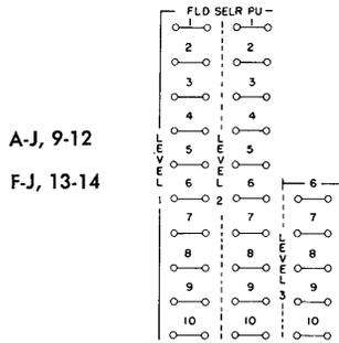
**FIELD SELECTORS PICK UP LEVELS 1, 2, AND 3:** These hubs when impulsed cause the corresponding level of a field selector to transfer on the same punch cycle. They are normally wired from CONTROL INFORMATION. An impulse to these hubs causes the field selectors to transfer immediately and remain transferred for the duration of that punch cycle.
