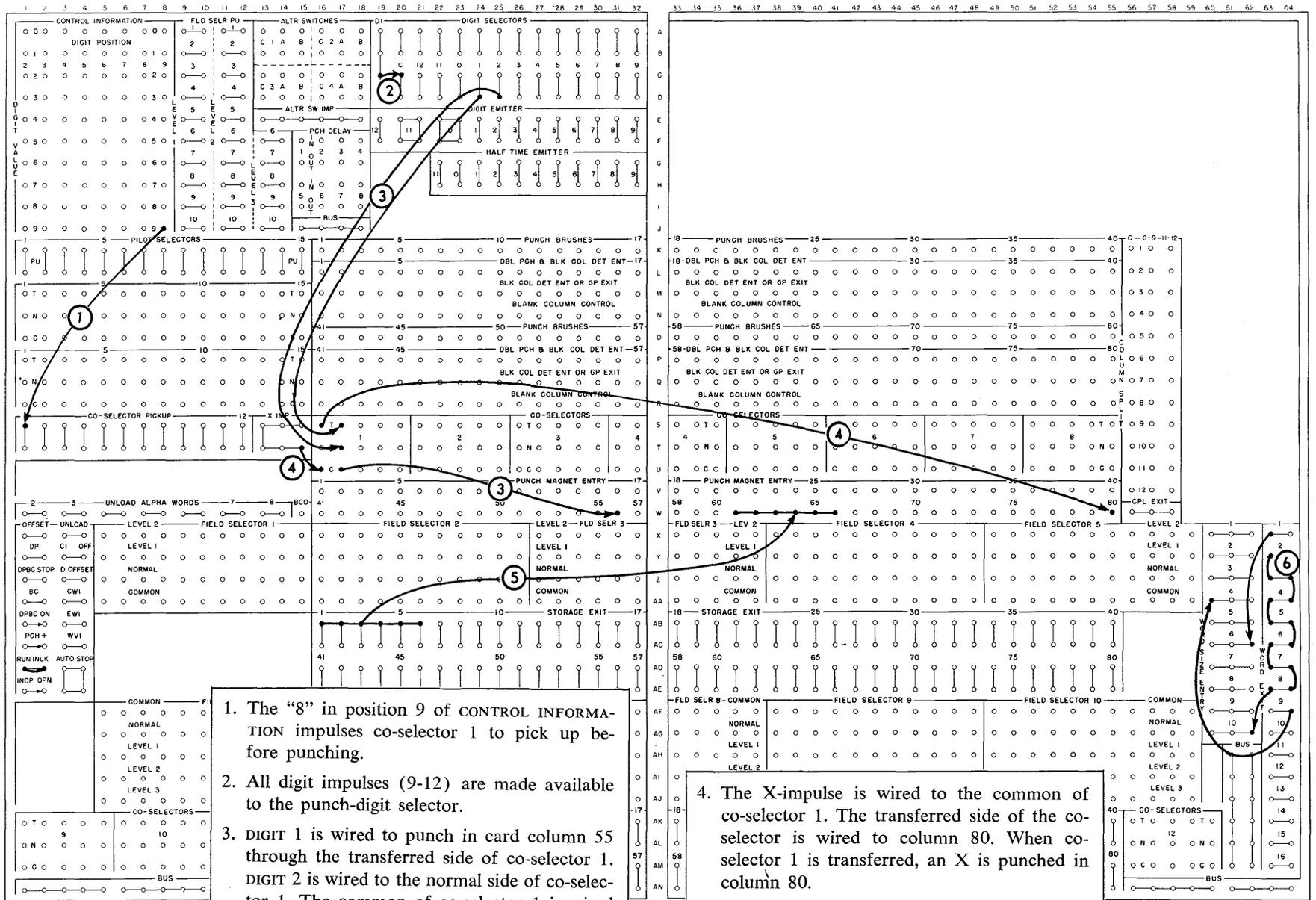
1. The "8" in position 9 of CONTROL INFORMATION impulses co-selector 1 to pick up before punching.
