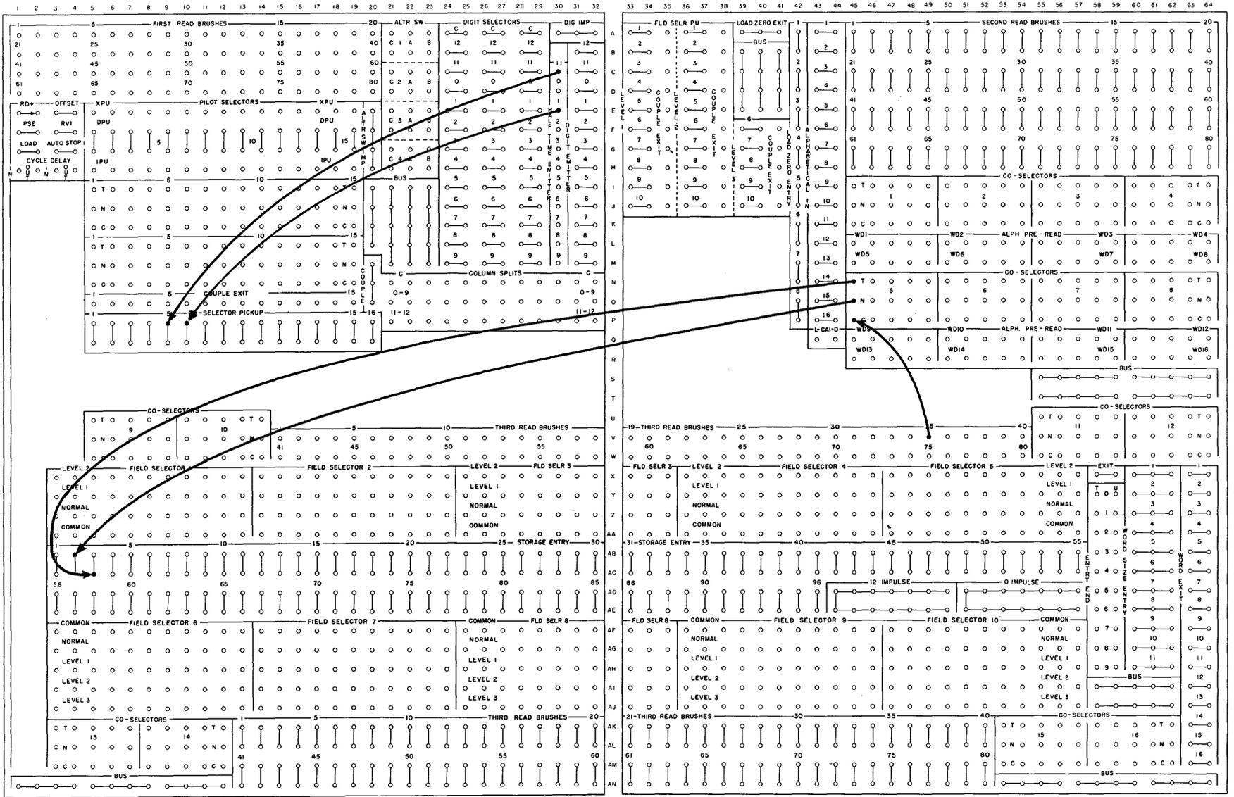
FIGURE 189. ALTERATION SWITCH WIRING
