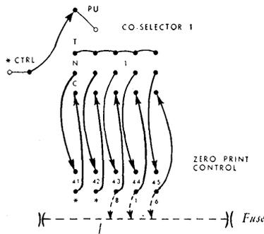
The impulse from position 41 can reach the fuse in a similar manner, by passing over two positions of the transferred side of the selector to zero print control position 43. The selector is picked up from \*CTRL so that the lower zero print control hubs will be connected at no-zone time only; at all other times they are wired to the upper hubs through the normal side of the selector.
