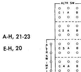
**ALTR SW (ALTERATION SWITCH) 1, 2, 3, 4:** Four alteration switches are located on the left front of the machine. Each alteration switch controls a corresponding two-position alteration switch selector. When the switch is set on A, a common connection exists between C and A; when the switch is set on B, a common connection exists between C and B.
