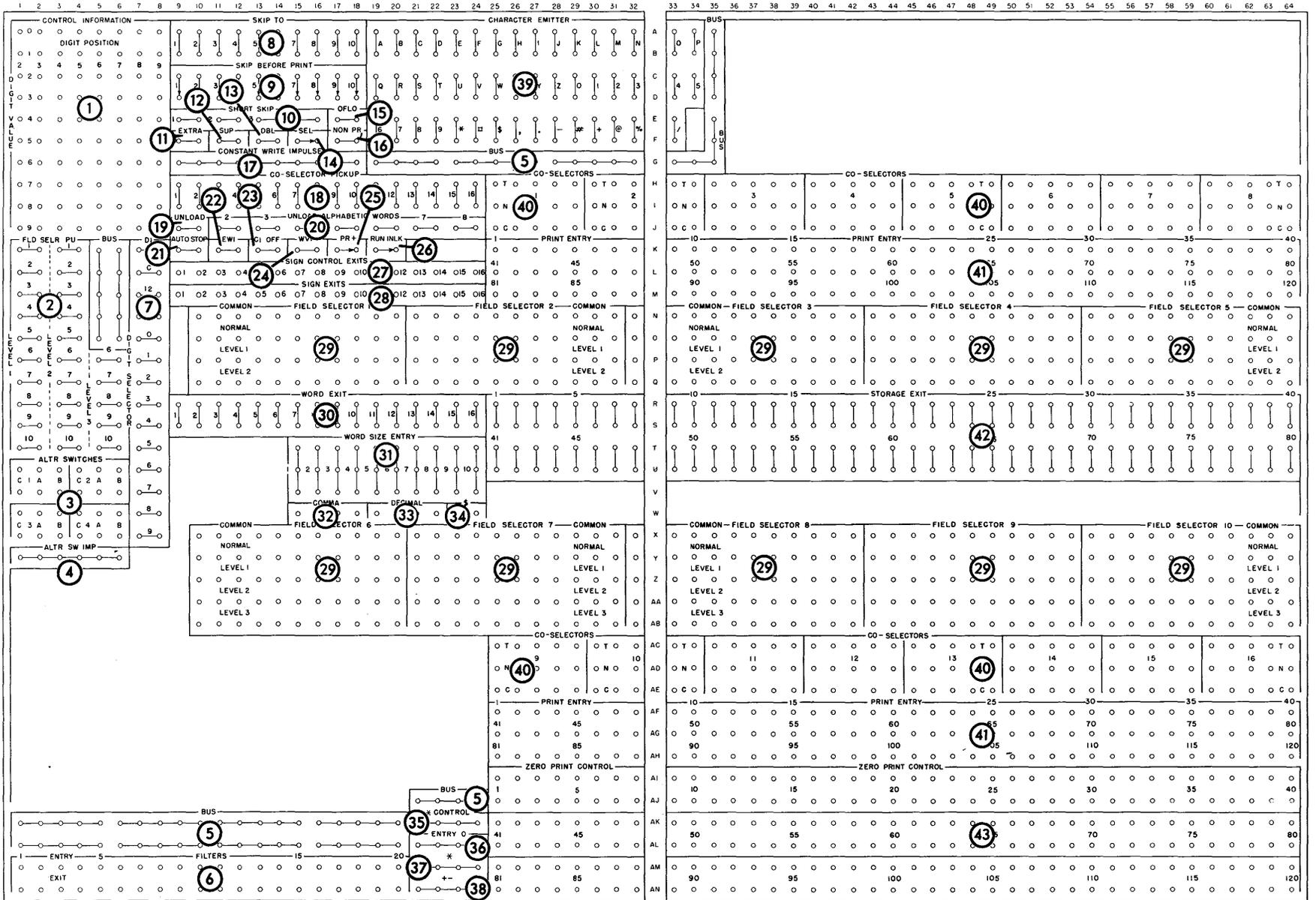
10. *Short Skip*. These are entry hubs normally wired from control information when the skip does not exceed two and a half inches. When these hubs are impulsed, the internal interlock is released and the skip takes place without lost time if skip before print is wired.
