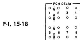
**PUNCH DELAY:** There are eight sets of punch delay hubs on the control panel. Each set of hubs consists of an in hub and out hub. The in hub accepts any impulse. The out hub emits an impulse just prior to punching time on the punch cycle following the one during which the in hub is impulsed. It is possible to delay up to eight cycles by wiring the OUT of one to the IN of another.
