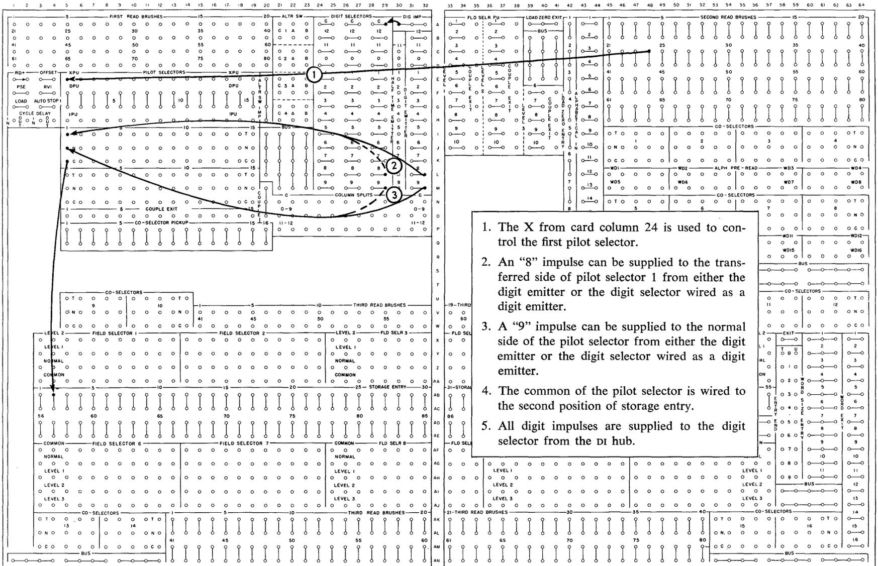
1. The X from card column 24 is used to control the first pilot selector.
