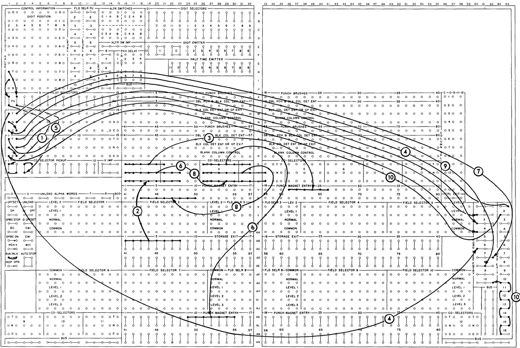
1. Pilot selector 1 and co-selectors 1 and 2 are impulsed by an "8" in CONTROL INFORMATION 2. These selectors transfer at the beginning of the punch cycle and remain transferred for the duration of that cycle.
