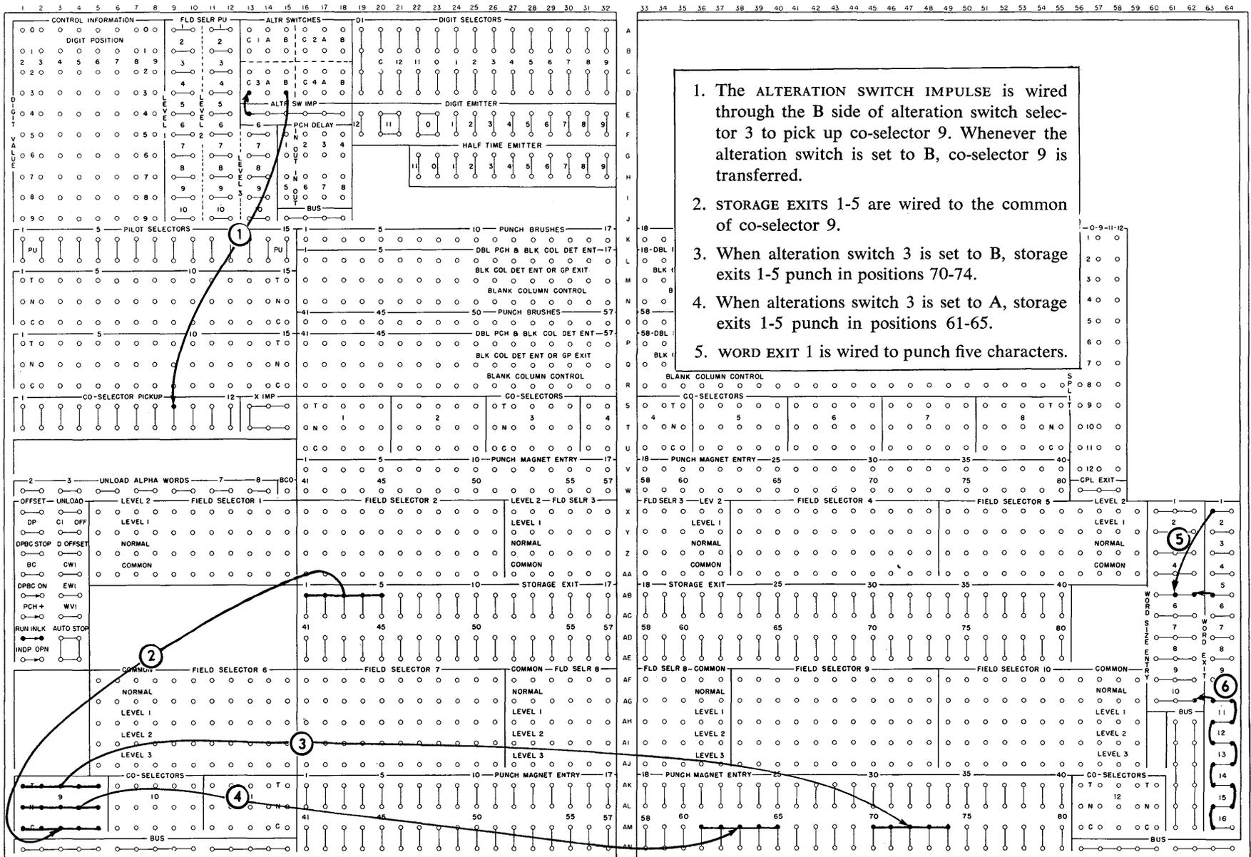
FIGURE 204. DOUBLE-PUNCH AND BLANK-COLUMN DETECTION, AND GANGPUNCHING
