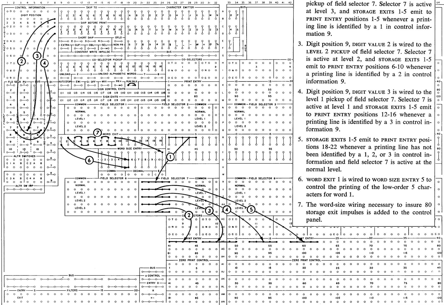
1. STORAGE EXITS 1-5 are wired to the COMMON of field selector 7.
