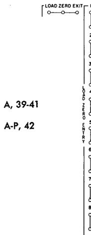
**LOAD ZERO ENTRY:** These hubs are assigned to the eight input words that are active on load cards. If any word in a load card contains invalid data, the LOAD ZERO ENTRY hubs associated with that word must be wired from the LOAD ZERO EXIT hubs.
