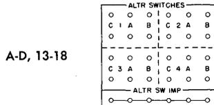
**ALTR SW (ALTERATION SWITCH) 1, 2, 3, 4:** Four alteration switches are located on the front of the machine. Each alteration switch controls a corresponding 2-position alteration switch selector. When the switch is set on A, a common connection exists between C and A; when the switch is set on B, the connection is between C and B. An alteration switch selector remains transferred as long as the corresponding alteration switch is set on B. Any impulse may be wired through C-A or C-B.
