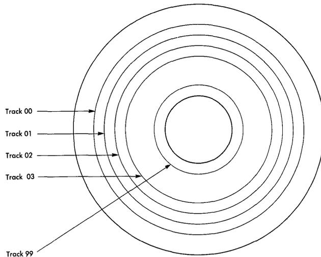
FIGURE 154. TRACK SCHEMATIC OF AN IBM 7300 MODEL 1 DISK
