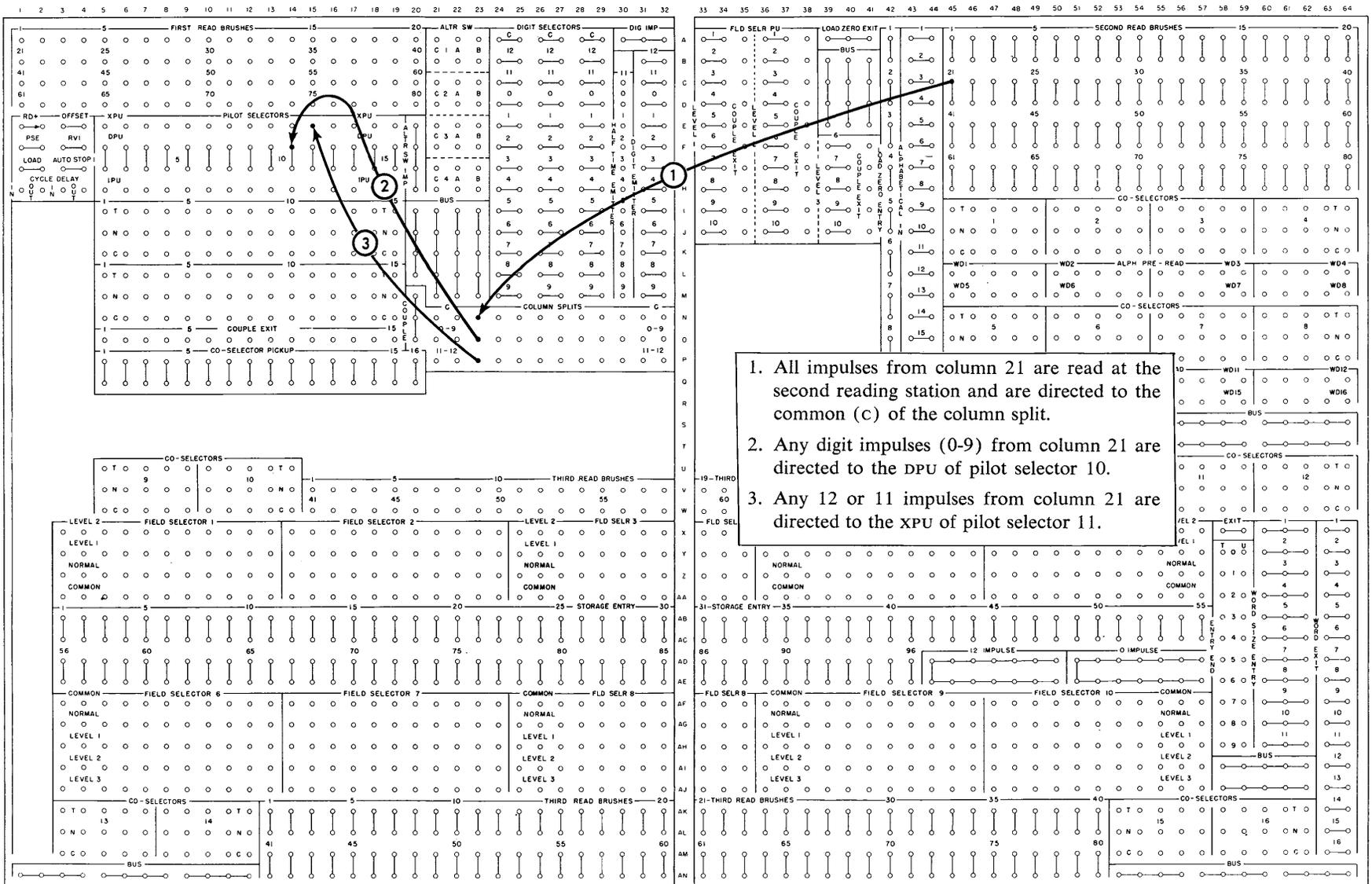
checked. The data read at second reading are stored and compared with the same data when the card advances past the third reading station. Each storage word can contain a maximum of five alphabetic characters. The sign is *not* counted as a character to be read but is automatically entered in the input synchronizer.
