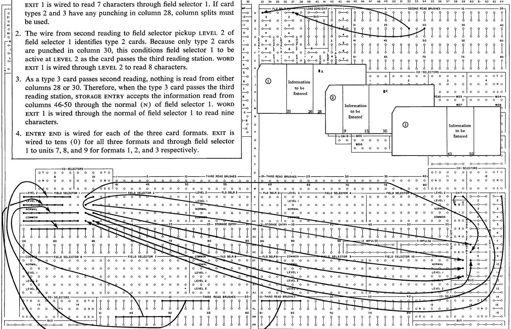
FIELD SELECTOR LEVELS 1, 2, AND 3—NORMAL AND COMMON: There are ten, 11-position field selectors provided. Field selectors 1-5 have 3 levels each (NORMAL, LEVEL 1 AND 2); selectors 6-10 have 4 levels each NORMAL, LEVEL 1, AND 2, AND LEVEL 3).
