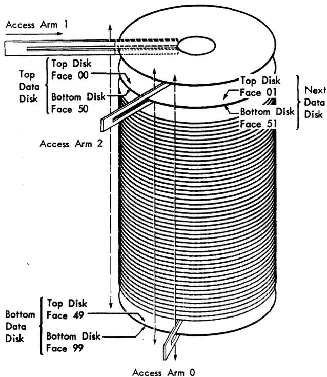
FIGURE 153. SCHEMATIC OF 7300 DISK FACE ARRANGEMENT
