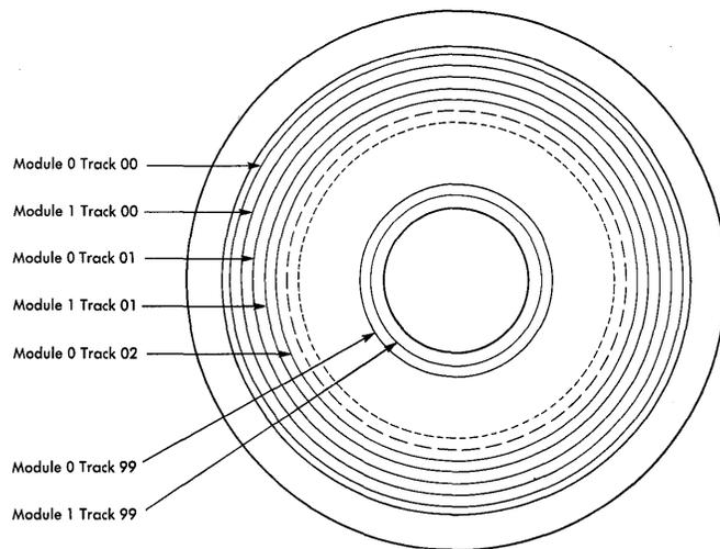
FIGURE 155. TRACK SCHEMATIC OF AN IBM 7300 MODEL 2 DISK
