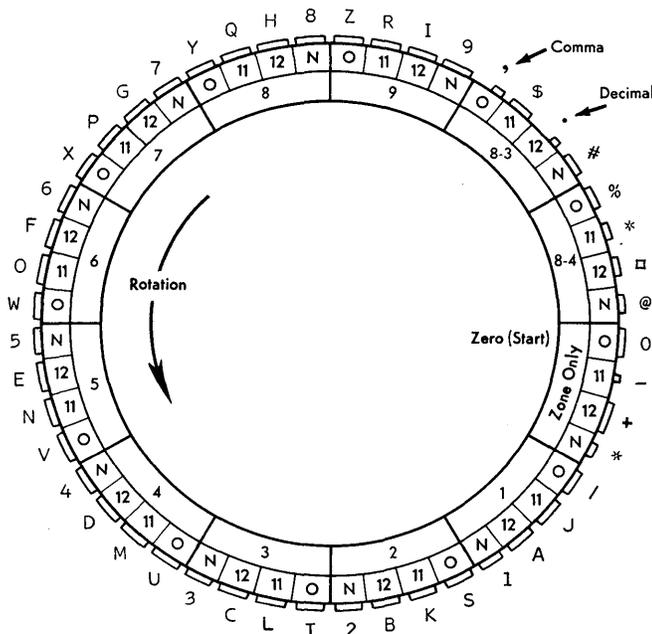
FIGURE 210. 7400 PRINTWHEEL SCHEMATIC
