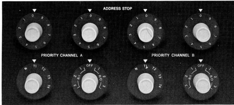
FIGURE 279. ADDRESS STOP AND UNIT-RECORD PRIORITY CONTROLS
