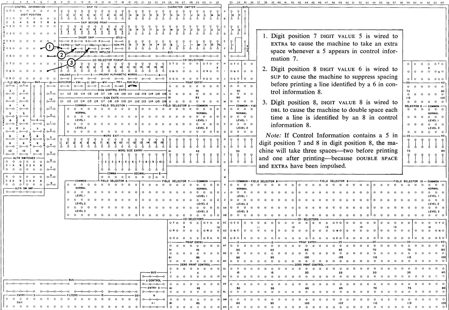
1. Digit position 7 DIGIT VALUE 5 is wired to EXTRA to cause the machine to take an extra space whenever a 5 appears in control information 7.
