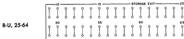
**STORAGE EXITS:** As many as 80 characters from the sixteen words contained in the output-synchronizer can be controlled to exit through these 80 hubs. STORAGE EXIT impulses are normally wired to the PRINT ENTRY hubs. Sign control is explained in a later section.
