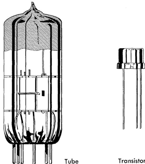
FIGURE 1. RELATIVE SIZES OF VACUUM TUBE AND TRANSISTOR
