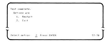
Remove the wrap connector from the back of the machine and replace the cable. You can then choose either to end the test or to run the test again.
