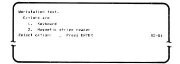
6. Select the option for the test you want, and press the Enter key. If you choose option 1, keyboard, continue in *Part 1 (Keyboard)* of this procedure. If you want to test only the magnetic stripe reader, option 2, go to *Part 2 (Magnetic Stripe Reader)* of this procedure.
