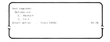
7. You may test other keyboards and any magnetic stripe readers by selecting option 2 which takes you back to the prompt for program name. At the next keyboard, repeat *Part 1 (Keyboard)*. Continue repeating this part until you have completed testing keyboards.
