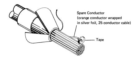
9. Locate the colored conductors listed in the table for the cable you are assembling and cut those conductors  $5\pm1$  millimeter (0.20  $\pm$  0.04 inch) shorter than the other conductors. This will allow a better lay in the covers.
