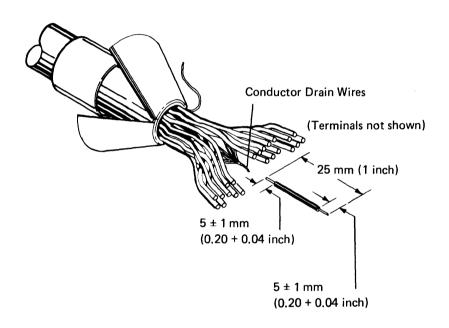
17. Use minimum heat and carefully solder the conductor drain wires and the black wire together. Ensure that the section of the black wire where the insulation has been removed remains exposed.
