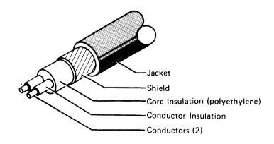
The following table provides bulk cable specifications for twinaxial cable
