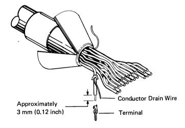
$\underline{\text{Note}}$ : Do not solder the terminal or insert it into its assigned connector hole.
