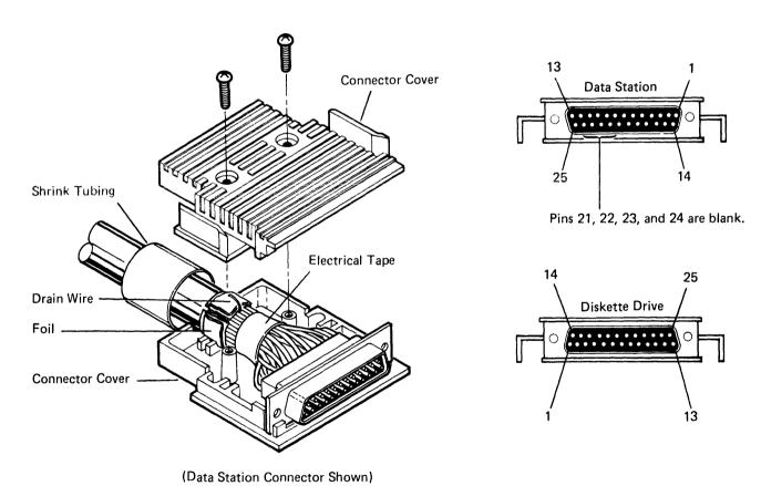
31. Attach the sticky label (provided with connector kit) in the postion shown. A yellow label should be attached to a diskette drive cable connector; a green label to the data station cable connector.
