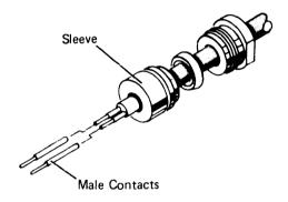
6. Bend the conductors and the contacts out at right angles to the cable axis; then bend the conductors back to parallel (approximately 6.4 millimeters (0.25 inch) between conductors).
