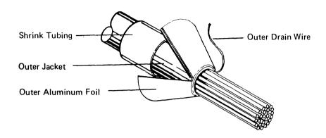
8. The exposed conductors are individually wrapped in aluminum foil and are color coded in two ways: the color of the aluminum foil wrapping and the color of the inner insulation around the conductor. The orange conductor wrapped in silver colored foil (in the 25 conductor cable) is a spare conductor; place a piece of electical tape over the end of this conductor.
