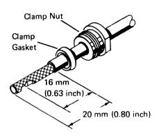
3. Slide a braid clamp over the braid so that its inner shoulder butts against the cable jacket. Then, fold the shield back over the braid clamp and trim below the shoulder.
