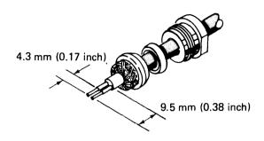
5. Slide the sleeve over the cable core and press the sleeve against the braid wires.
