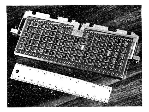
Figure 7. Pluggable Electronic Subassembly
