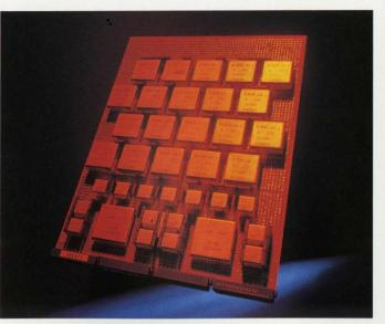
One million bytes of main storage are packaged on this single card. 16 million bytes of storage can be provided on IBM 4381 models with 16 cards.
