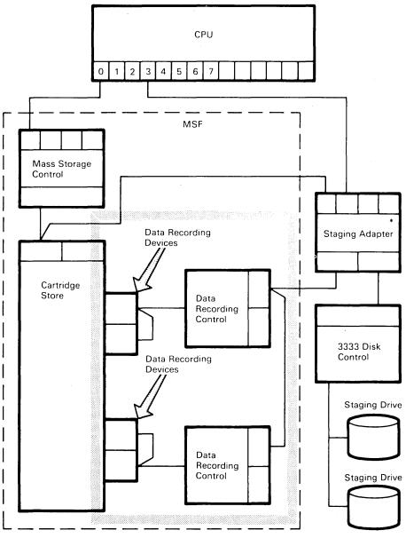
\*The Staging Adapter can be a 3830 Model 3 or the Staging Adapter feature on the Integrated Storage Control feature.
