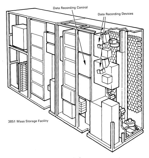
Figure 5. Data Recording Control and Devices
