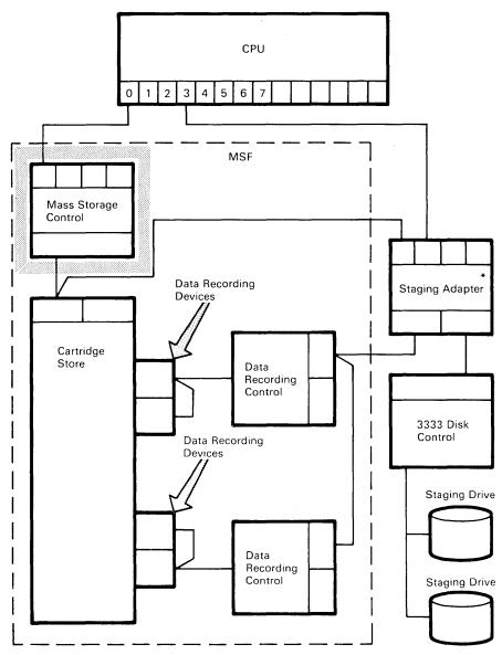
\*The Staging Adapter can be a 3830 Model 3 or the Staging Adapter feature on the Integrated Storage Control feature.
