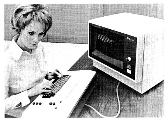
Figure 8-20. IBM 2265 Display Station with Alphameric Keyboard
