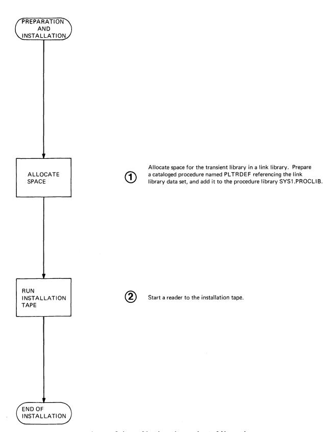
Figure 4. Preparation and installation (transient library)
