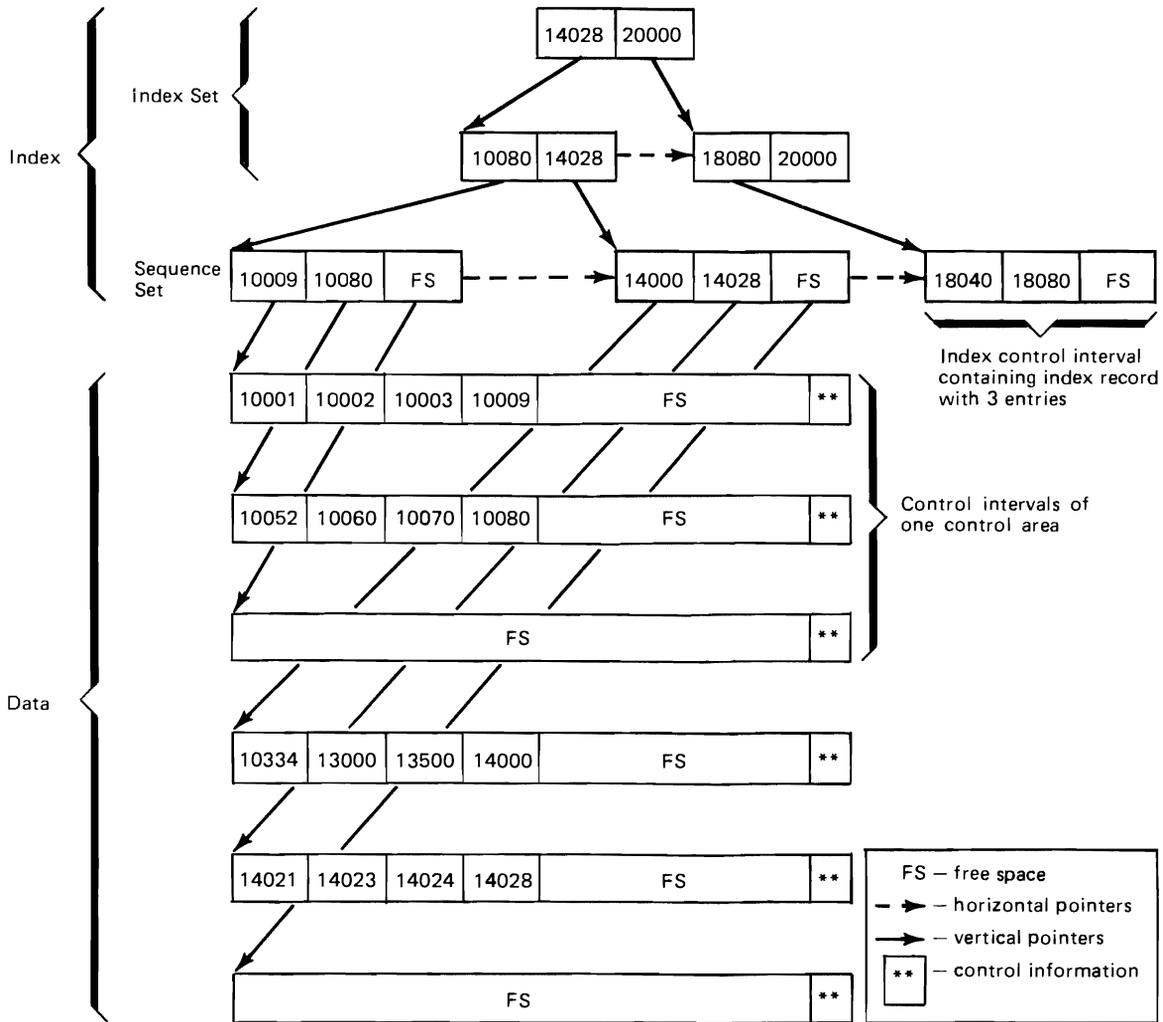
Figure 14. VSAM's Index Structure for a Key-Sequenced File
