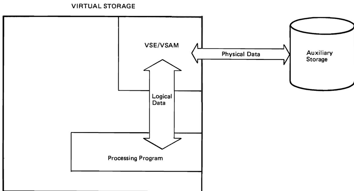
Figure 1. Position of VSE/VSAM between a Processing Program and Auxiliary Storage
