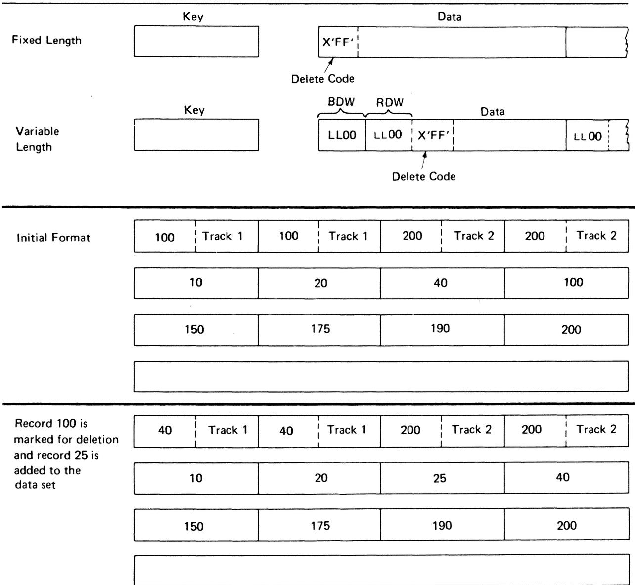
Figure 64. Deleting Records from an Indexed Sequential Data Set
