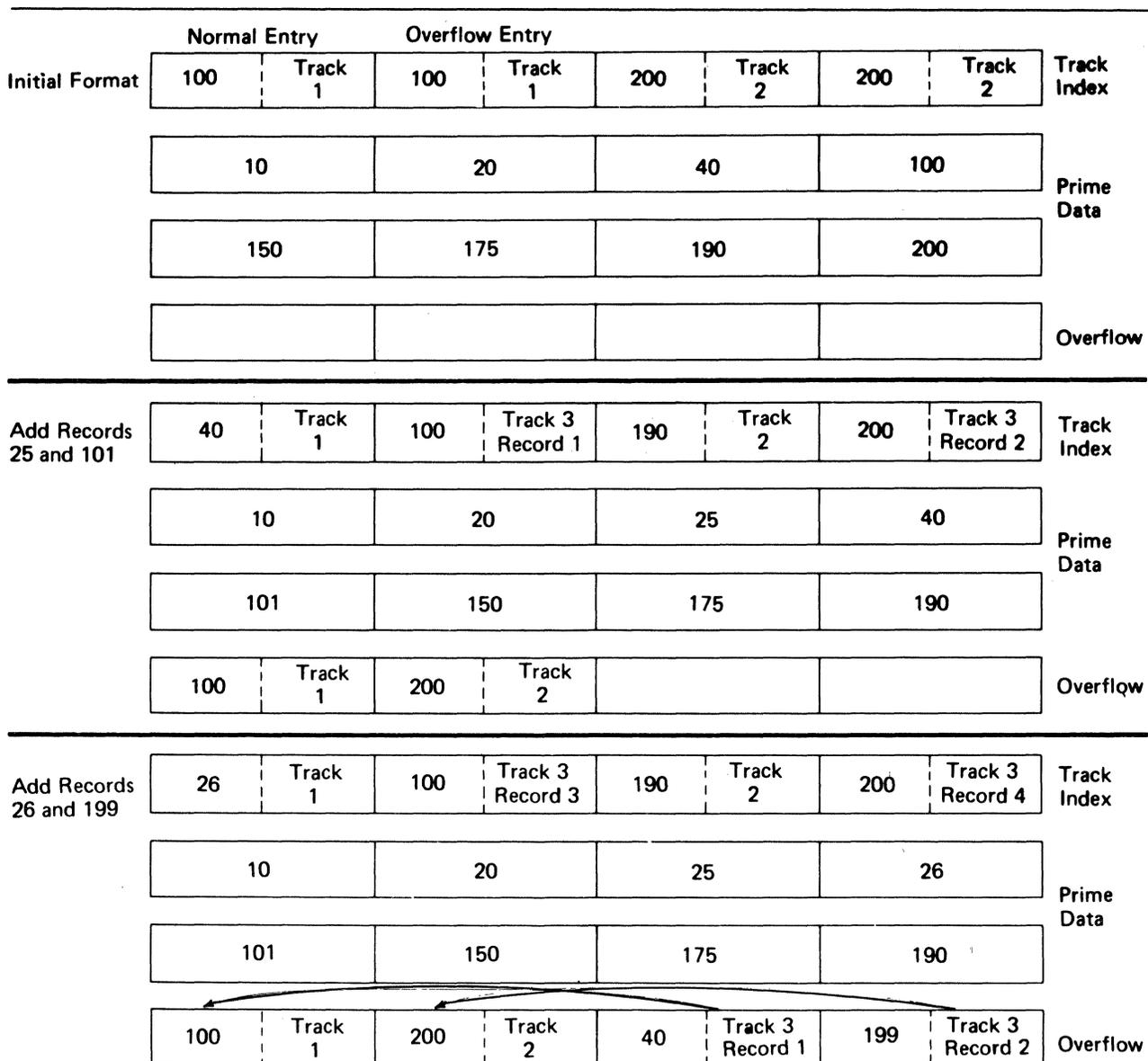
Figure 63. Adding Records to an Indexed Sequential Data Set
