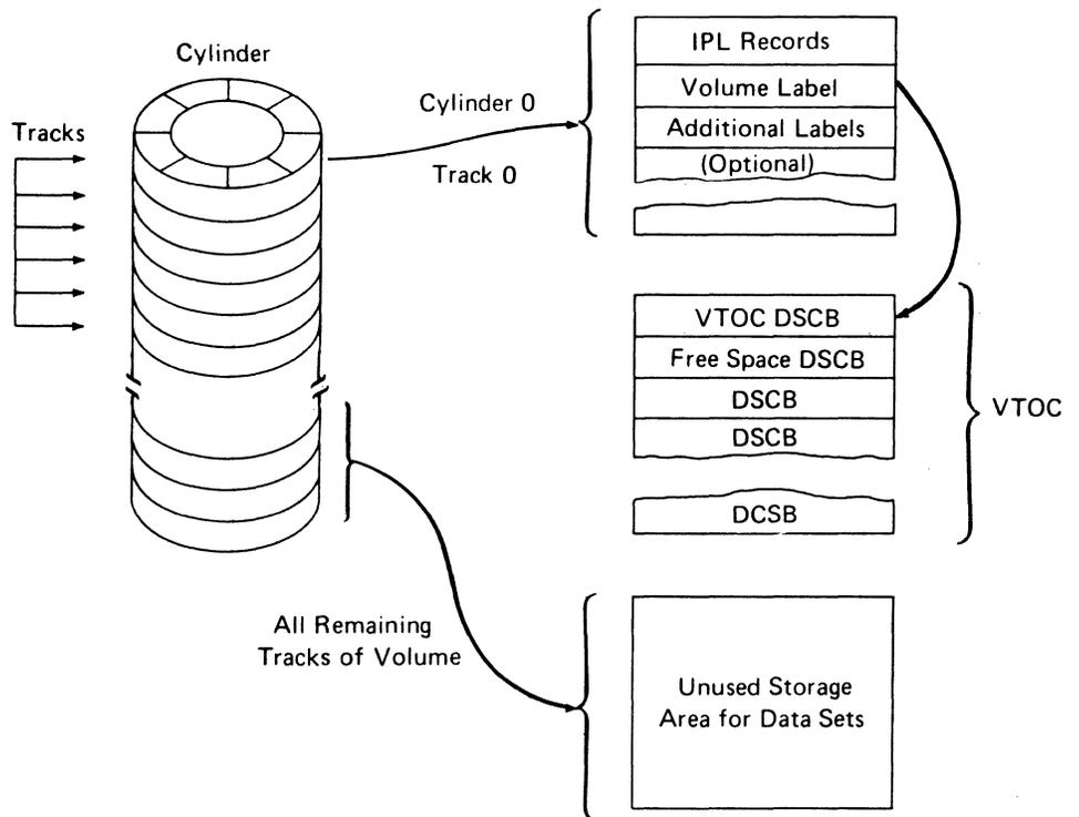
Figure 65. Direct Access Labeling
