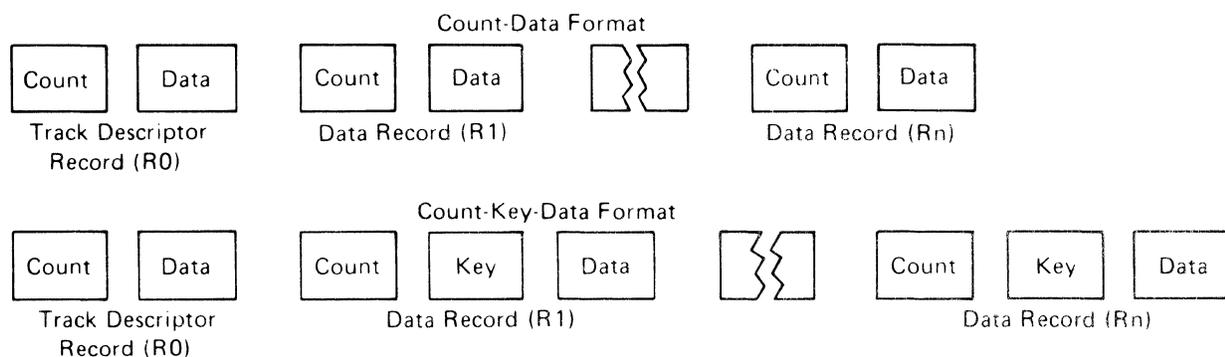
**Figure 1. Direct Access Volume Track Formats**
