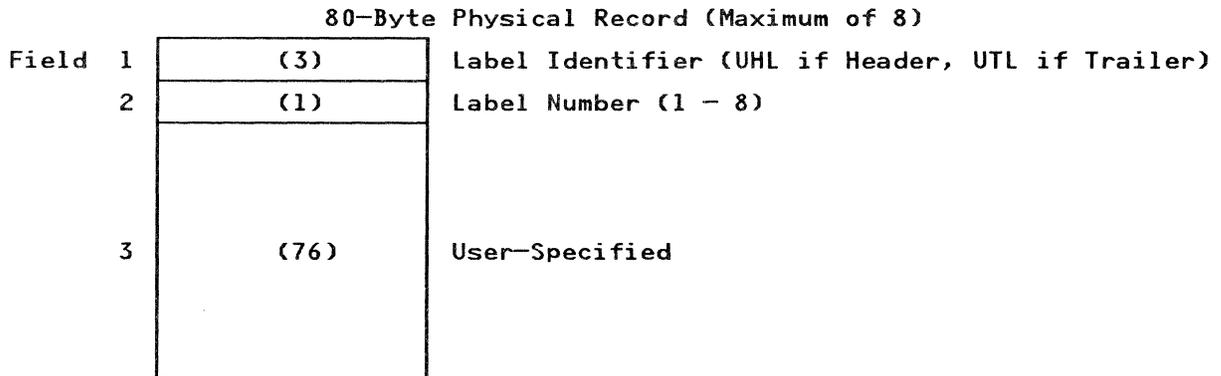
Figure 67. User Header and Trailer Labels
