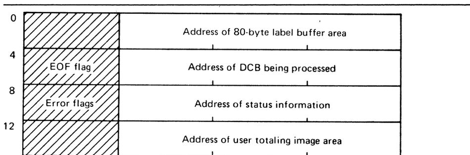
Figure 24. Parameter List Passed to User Label Exit Routine
