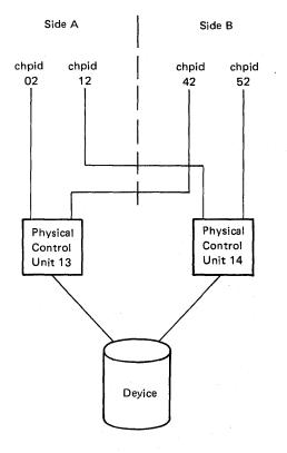
Figure 1-5. Channel Path Selection on a 3084 Processor Complex
