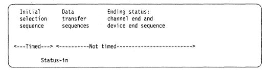
Example B. Command chaining control unit initiated reconnection sequence
