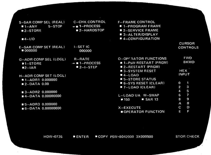
After recognizing the failure an operator is able to 'scan' the display frames and thus obtain detailed information about the condition of the hardware. This information may enable the IBM CE to diagnose the failure immediately and advise on continued system operation. He may also advise that the SEREP is executed and request 'hard copies' of the display frame on which the failure is indicated to enable an offline diagnosis of the failure.
