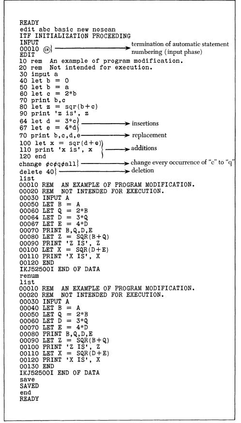
Figure 12. Example of Modifying a Program As It Is Being Created
