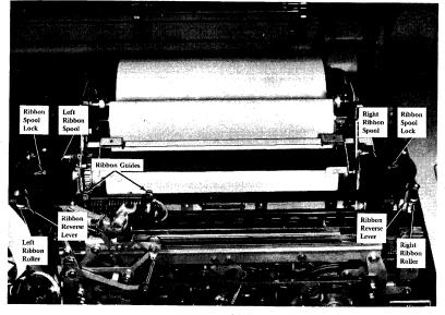
Figure 18. Type 35 ASR ribbon controls
