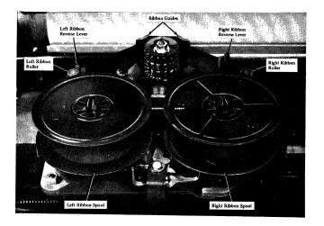
Figure 14. Type 33 ASR ribbon controls
