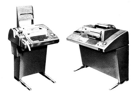
Figure 2. Teletype units, Type 33 ASR (left) and Type 35 ASR
