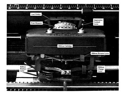
Figure 6. 2741 ribbon/print element carrier
