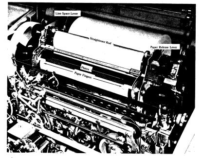
Figure 17. Type 35 ASR paper insertion and movement controls
