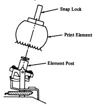
Figure 8. Position of print element while being removed or replaced
