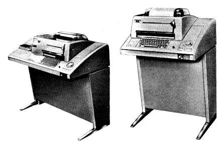
Figure 15. Teletype units, Type 35 ASR (left) and KSR
