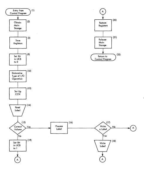
Figure 15. General Flow of a Nonstandard Label Processing Routine After Receiving Control From the EOV Routine
