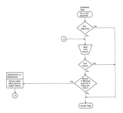
Figure 20. Verification of First Record When Unlabeled Tape Is Specified
