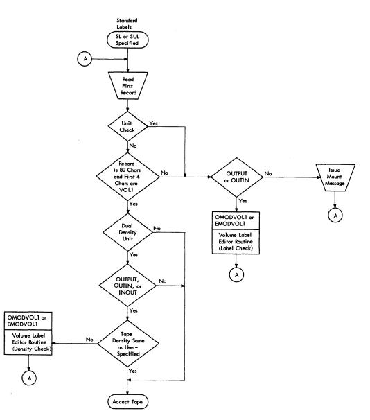
Figure 18. Verification of First Record When Standard Labels Are Specified
