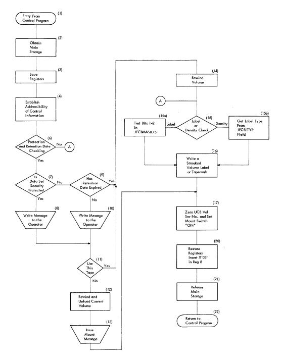
Figure 22. General Flow of an Editor Routine After Receiving Control From the EOV Routine
