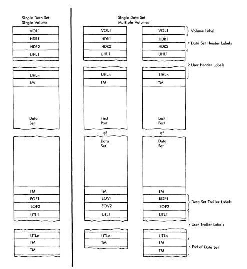
Single Data Set/Single Volume: The volume label is followed by the data set header labels and optional user header labels. The data set is preceded and followed by a tapemark. The data set trailer labels are identified as EOF and followed by optional user trailer labels. Two tapemarks follow the trailer label group to indicate that the data set is the last data set on the volume and is not continued on another volume.
