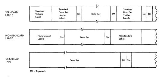
Figure 1. Basic Tape Layouts
