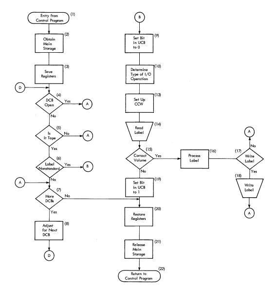
Figure 13. General Flow of a Nonstandard Label Processing Routine After Receiving Control From the Open Routine
