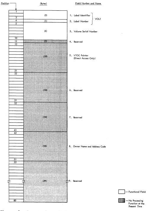
Figure 5. Format of Standard Volume Label
