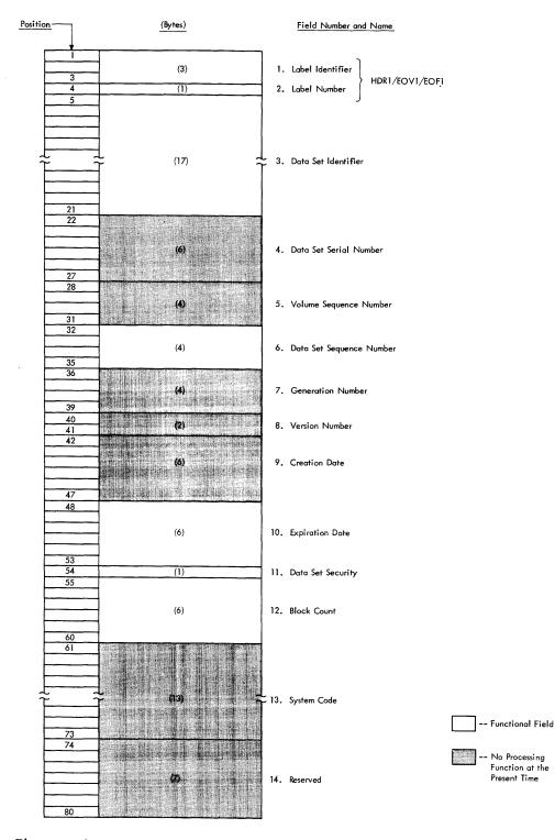
Figure 6. Format of Standard Data Set Label 1
