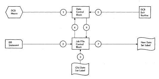
Figure 2. Sources and Sequence for Completing the Data Control Block
