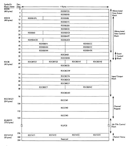
Figure 26. Restart Work and Control Block Area
