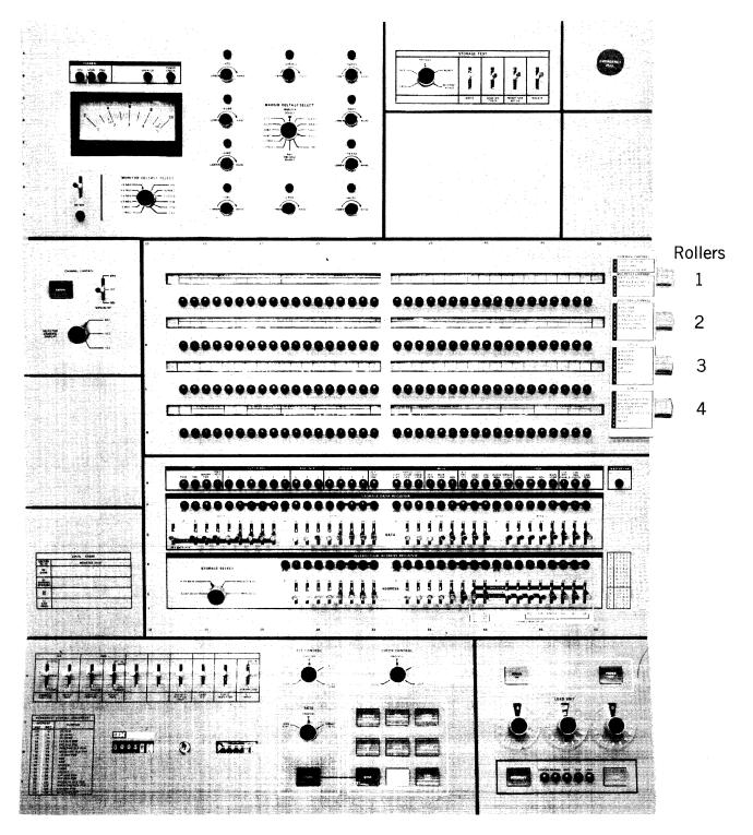
Figure 18. Model 50 System Control Panel
