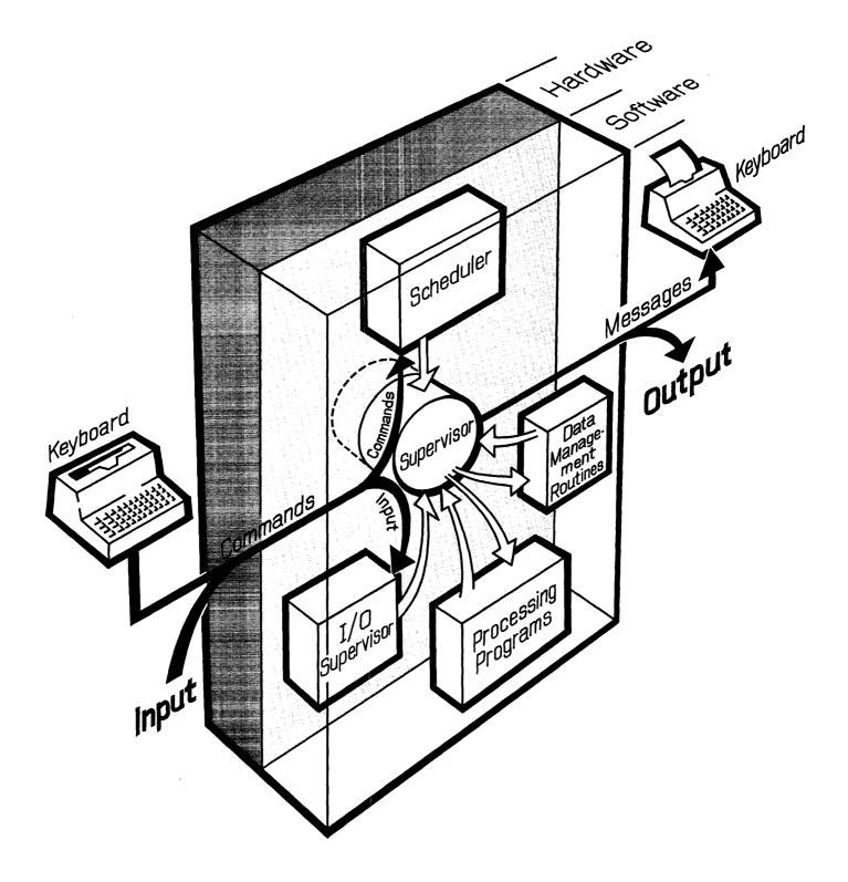
Figure 1. How the System Works
