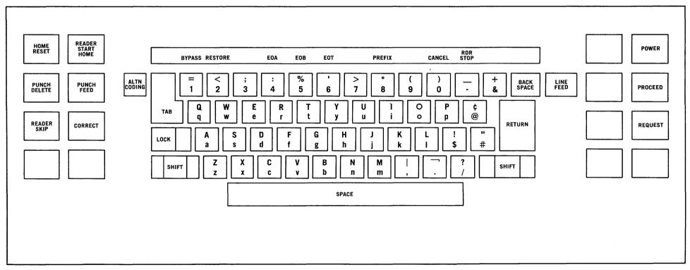
Figure 7. Model 5 Keyboard and Switch Panel
