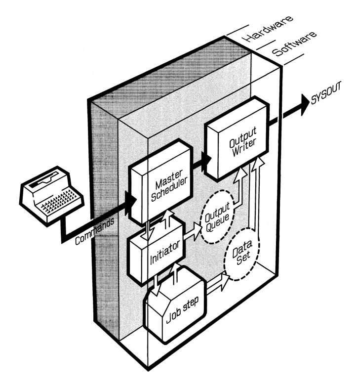
Figure 5. Output Process in Systems With MVT
