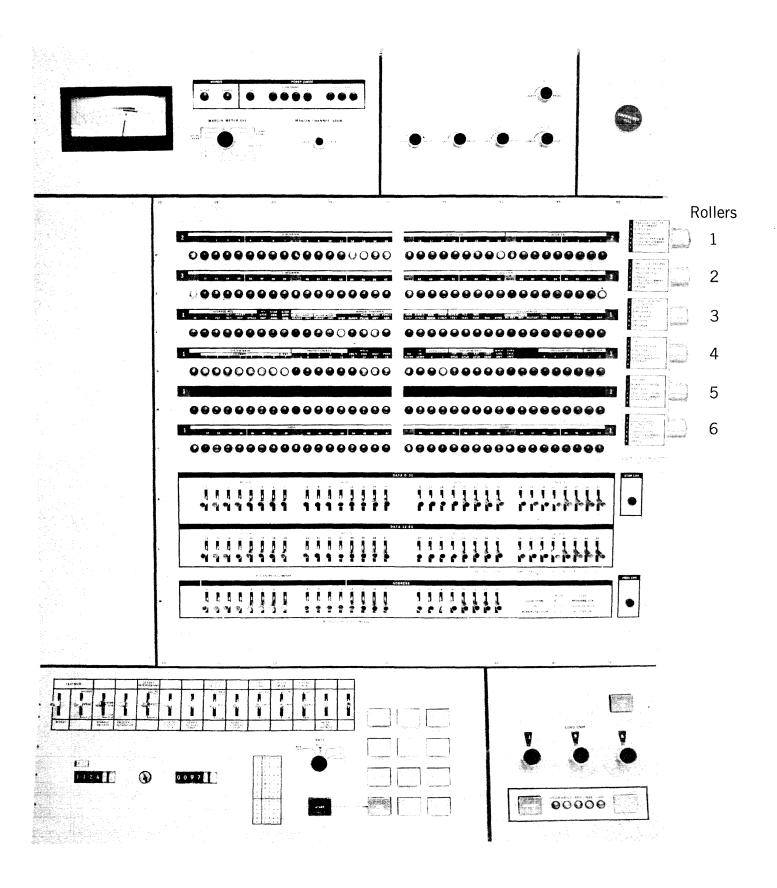
Figure 14. Model 65 System Control Panel
