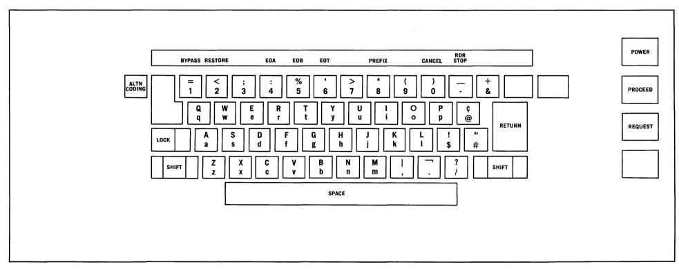
Figure 10. Model 8 Keyboard and SWITCH Panel
