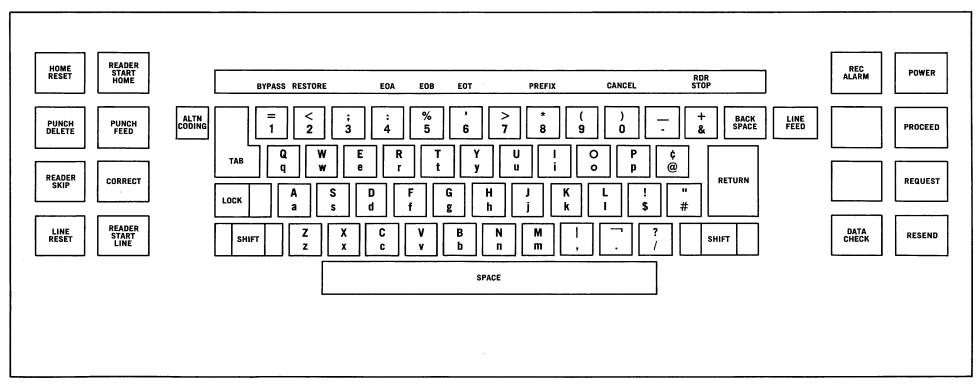
Figure 6. Model 3 Keyboard and Switch Panel
