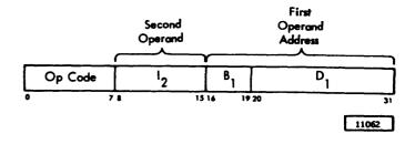
In the SI format, the address which specifies the core storage location of the first operand field is derived from the contents of the B1-D1 fields of the instruction. The address may be taken directly from the B1-D1 Fields (direct addressing) or an effective address may be formed by adding the contents of the general register specified by the B1 field to the contents of the D1 field (effective addressing).
