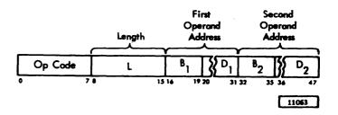
The address which specifies the core-storage location of the first operand field is derived from the B1-D1 fields of the instruction. The B2-D2 fields specify the leftmost byte of the second operand field. The first and second operand fields are the same length. The number of bytes extending to the right of the first byte is specified by the L field of the instruction.
