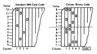
Figure 10. IBM Punched Card Codes
