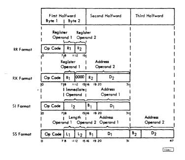
In each format, the first instruction halfword consists of two parts. The first byte contains the operation code (op code). The length and format of an instruction are specified by the first two bits of the operation code. The second byte may be used to contain data, specify operand lengths, or specify registers to be used by the operation.
