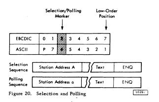
polling and selection, bit position 2 (in EBCDIC) and bit position 6 (in ASCII) are treated as "do not care" bit positions by the address decoding circuits. These bit positions are used to mark polling or selection. The BSCA is equipped with an address decoder for the station address. The station address is set up by the customer engineer when the feature is installed.
