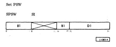
The 32-bit word (four eight-bit bytes), located in main storage with the leftmost byte at the first operand address, replaces the program Status Word (PSW).
