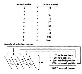
As shown above, the decimal number system allows counting to ten in each position-from units to tens to hundreds to thousands etc. The binary system allows counting to two in each position. Register displays in the System/360 are in binary form: a bit light on is a "one" a bit light off is a "zero".
