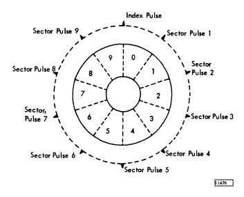
One of the sector pulses is called the index pulse and is used as a physical beginning point for the data on the track. For the purpose of description, a track is treated as a ten-sector group of data, beginning and ending with an index pulse. The data, as it is written on disk storage, is actually in the form of discrete, concentric circular tracks stacked ten high in the form of cylinders. Each sector is divided into two parts, the count area and the data area.
