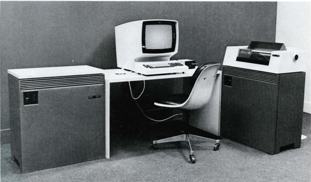
B. 3271/3272 Control Unit, and Attached 3277 Display Station and 3284/3286 Printer
