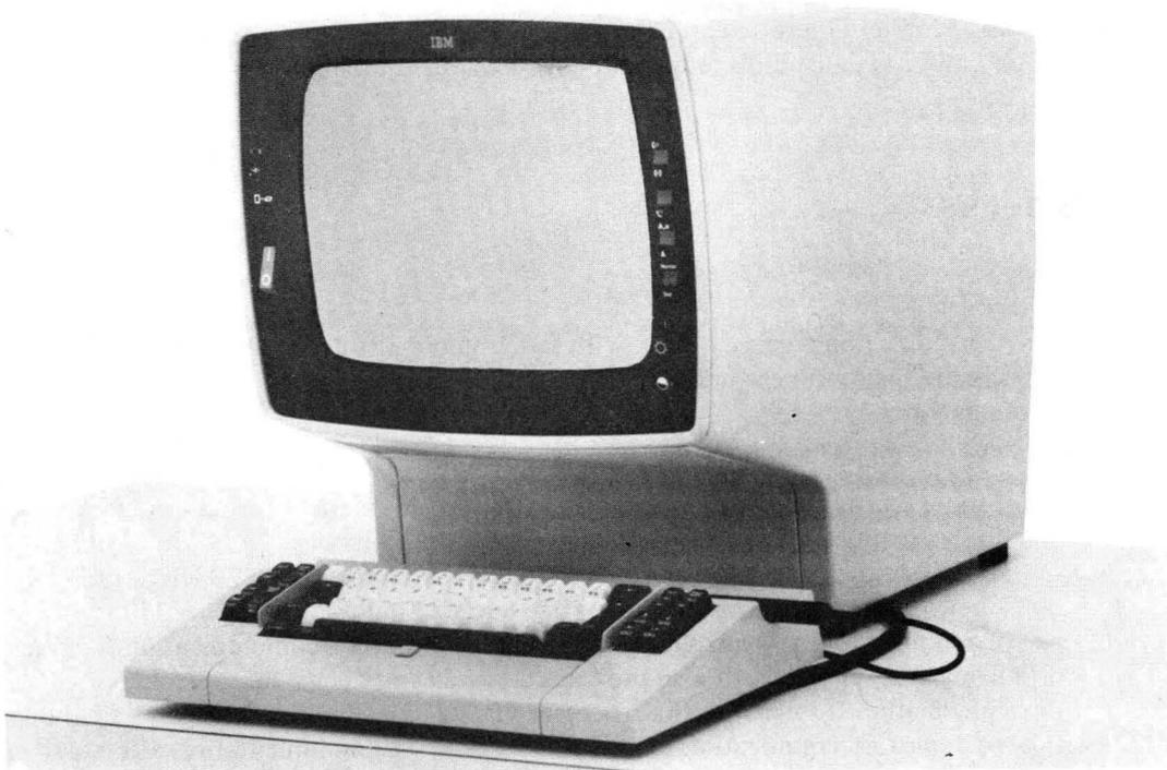
Figure 2-3. IBM 3276 Control Unit Display Station
