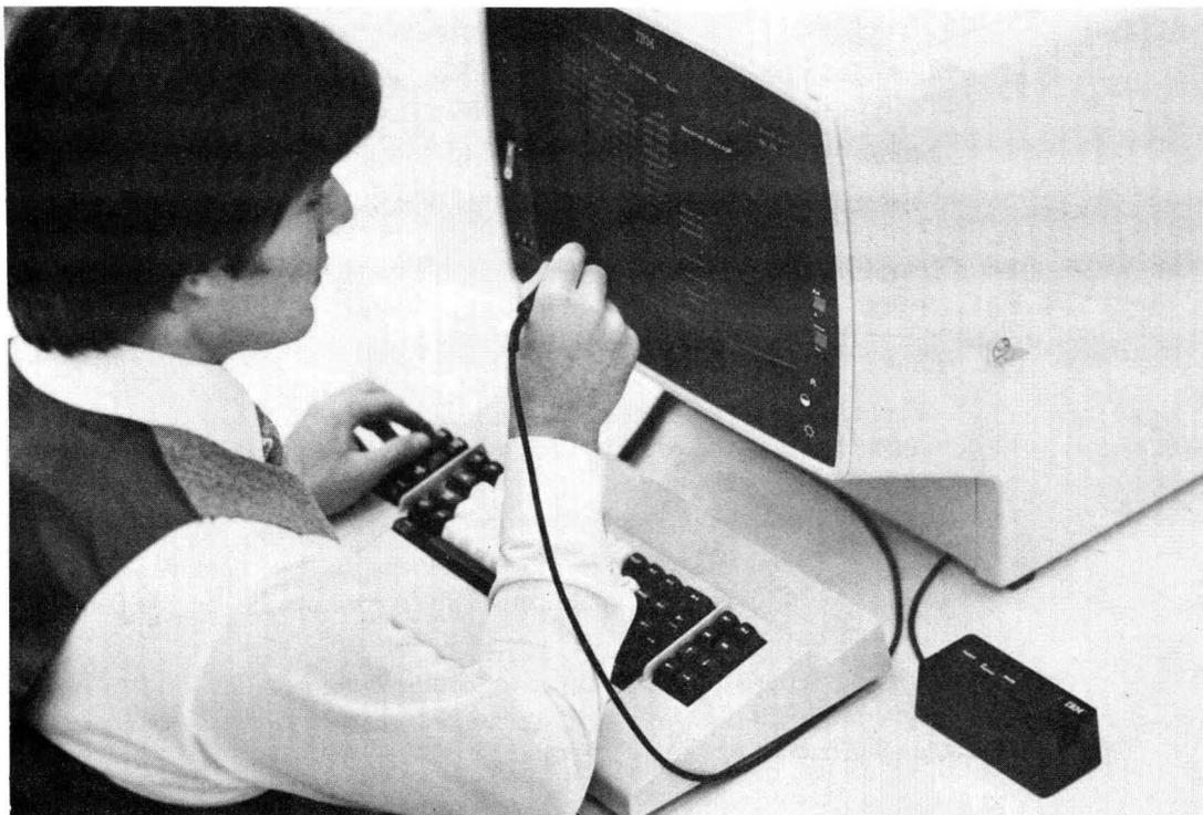
Figure 2-6. IBM 3278 Display Station with Keyboard, Selector Light Pen, Magnetic Slot Reader, and Security Keylock
