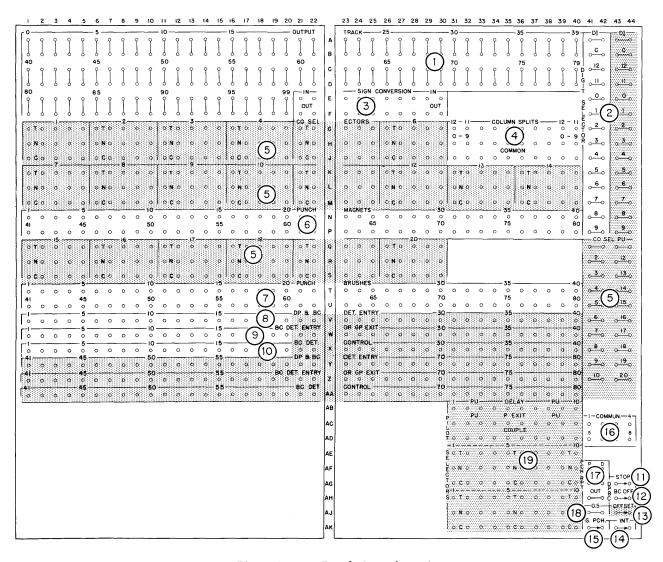
Figure 4. 323 Punch Control Panel
