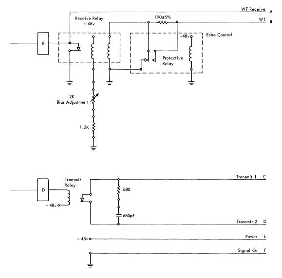
Figure 9. Telegraph Line Adapter WTC Connection to 3945
