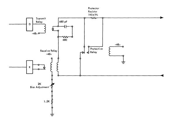
Figure 7. Telegraph Adapter Interface
