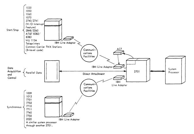
Figure 1. 2701 in a System Environment
