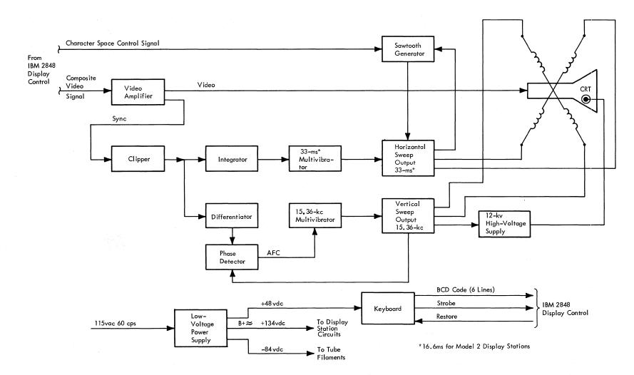
Figure 2-1. Display Station Block Diagram
