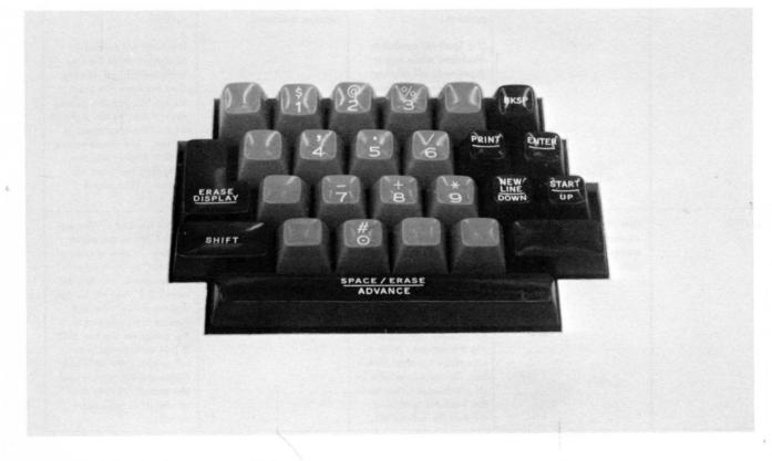
Figure 6-6. 2260 Display Station Numeric Keyboard
