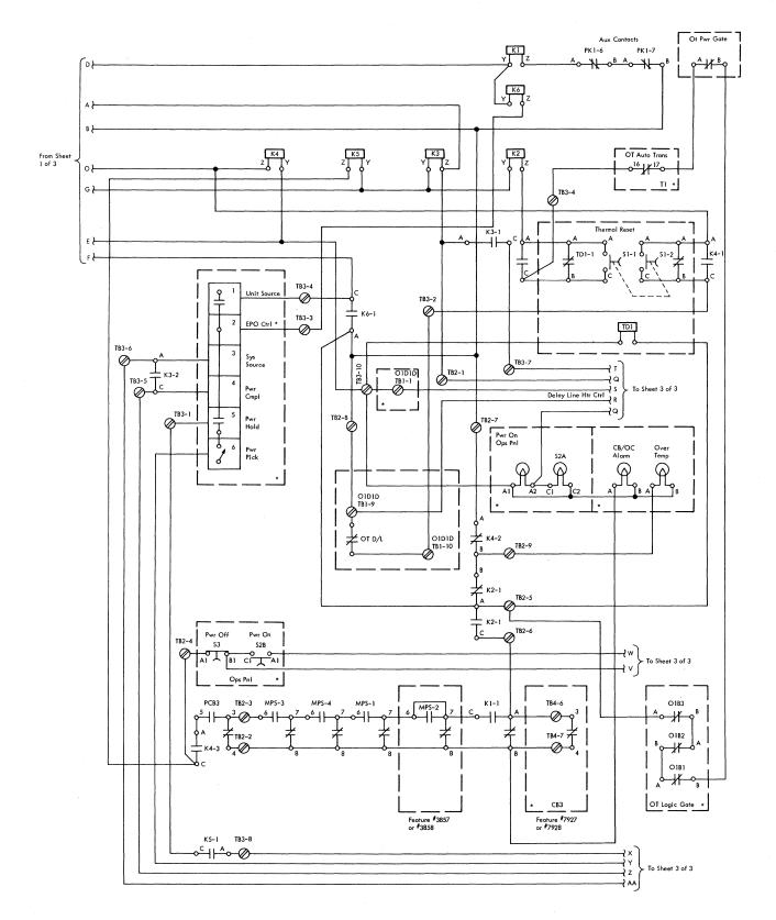
Figure 5-2. 50-Cycle Power Distribution and Control (Sheet 2 of 3)
