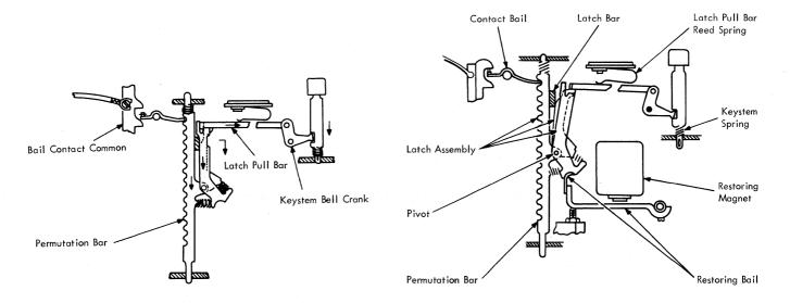
Figure 2-12. Permutation Bar and Keyboard Latch (Normal)
