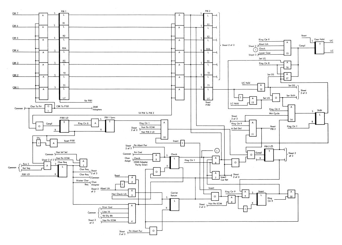
Figure 2-117. Printer Adapter, Logic Diagram (Sheet 1 of 3)
