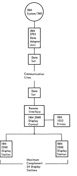
Figure 4-1. Remote Display Complex Configuration
