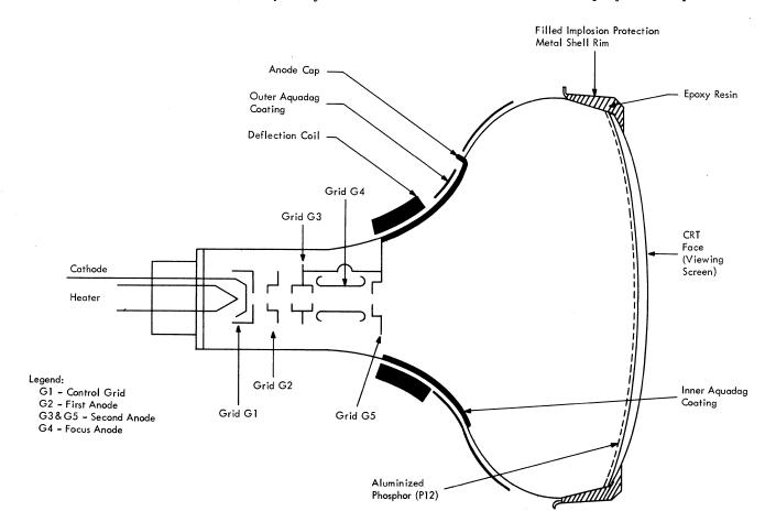
Figure 2-3. Cathode-Ray Tube
