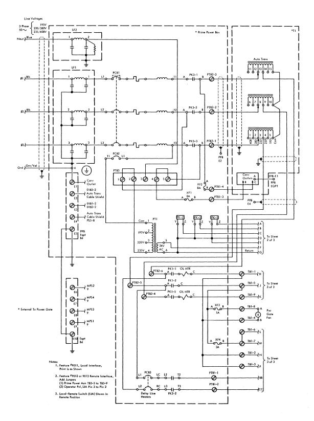
Figure 5-2. 50-Cycle Power Distribution and Control (Sheet 1 of 3)
