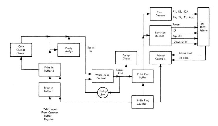
Figure 2-116. Printer Adapter, Simplified Block Diagram
