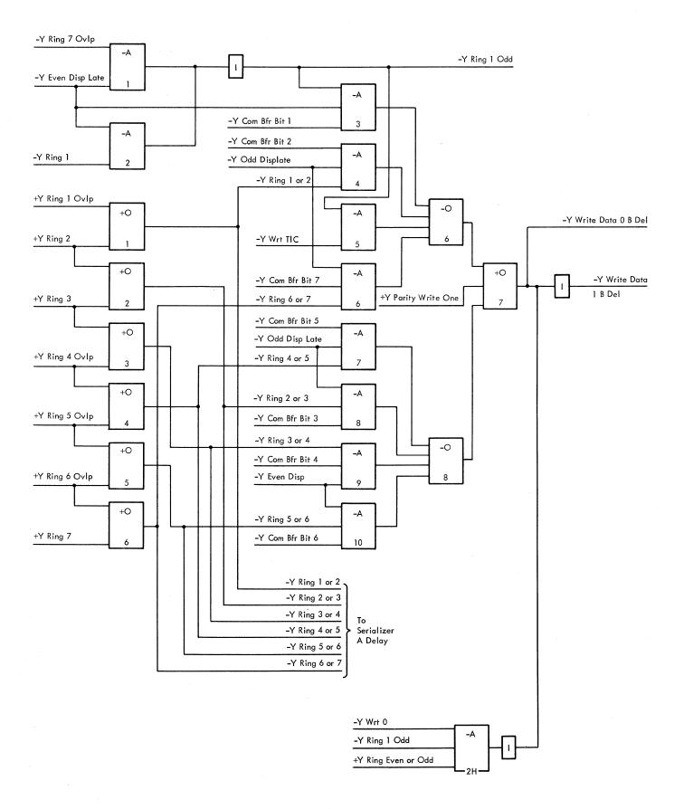
Figure 2-56. Serializer, B Delay
