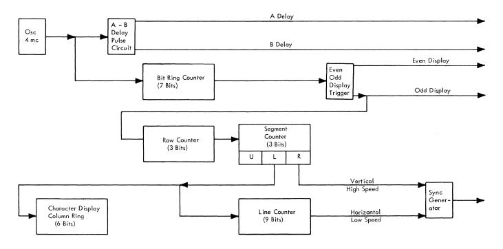
Figure 1-7. Timing and Clock Circuits, Simplified Block Diagram
