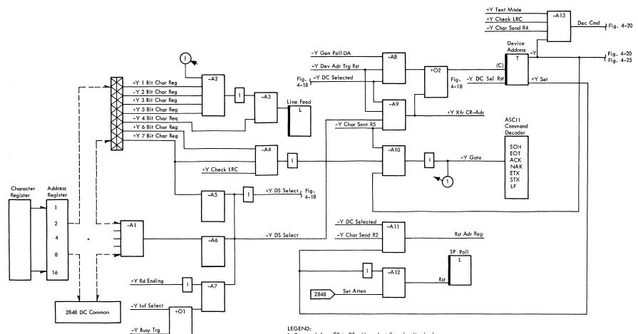
\* Data path from CR to DS address decoding circuitry is via back-panel jumpers wired by the CE according to the highest 2260/1053 address used by the customer.
