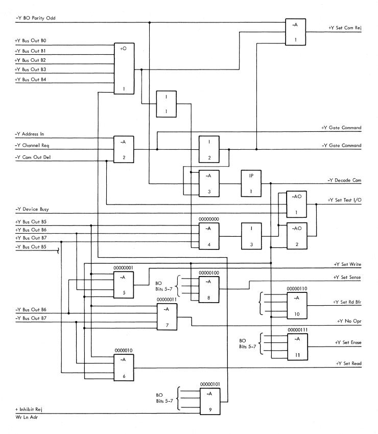
Figure 2-99. Command Decode
