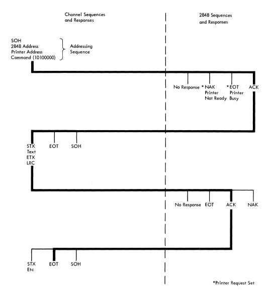
Figure 4-12. Sequence/Response Diagram - Write Printer
