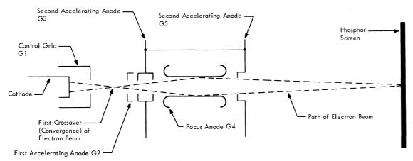
Figure 2-4. CRT Electron Gun
