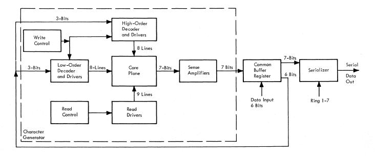
Figure 2-64. Character Generator, Block Diagram
