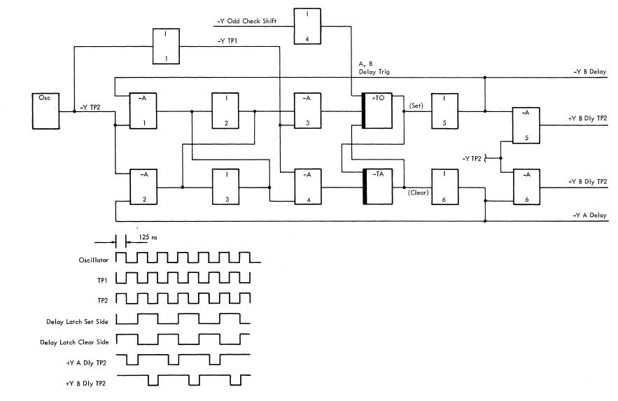
Figure 2-34. Oscillator and A-B Delay Pulse Circuit
