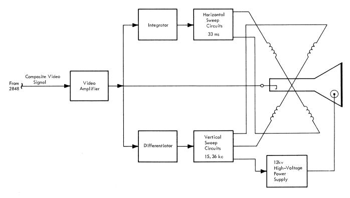
Figure 1-9. 2260 Display Station, Block Diagram
