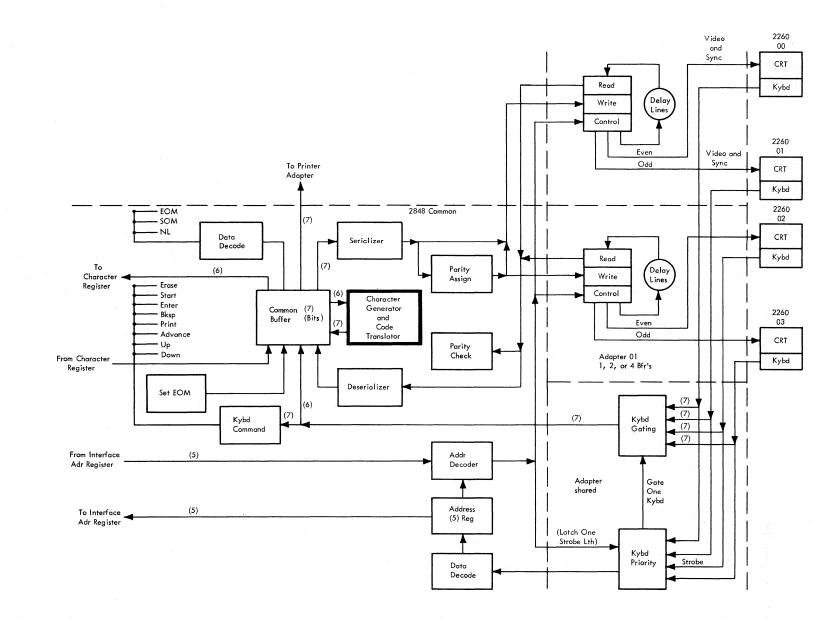
Figure 2-22. Display Control, Simplified Block Diagram
