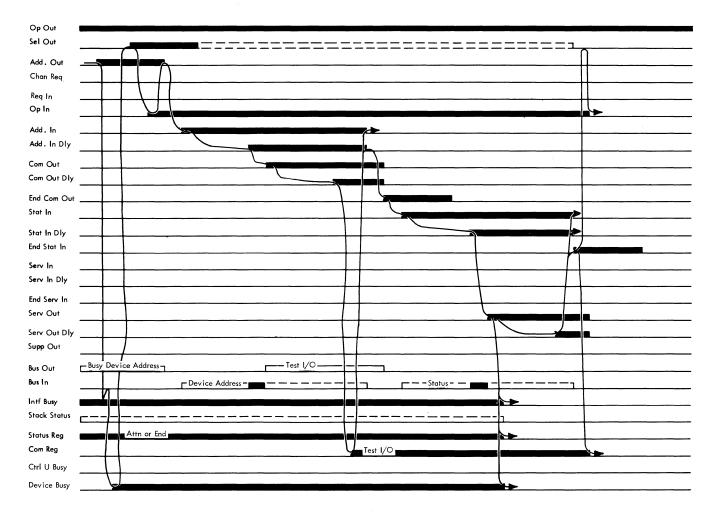
Figure 2-109. Test I/O To Busy Device
