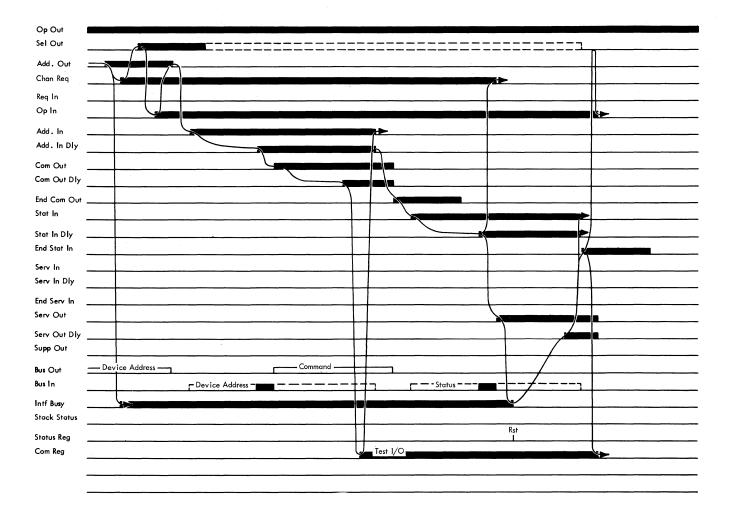
Figure 2-108. Test I/O Operation
