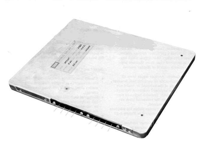
Figure 2-23. Delay Line Module
