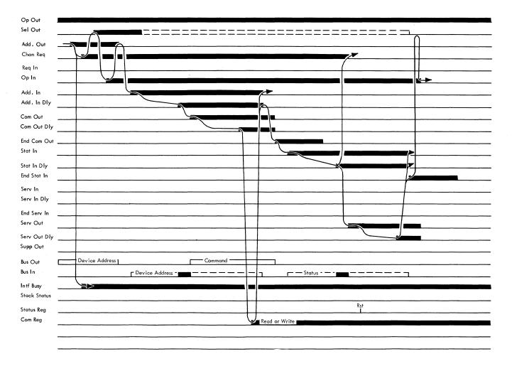
Figure 2-104. Channel-Initiated Selection (Read or Write)
