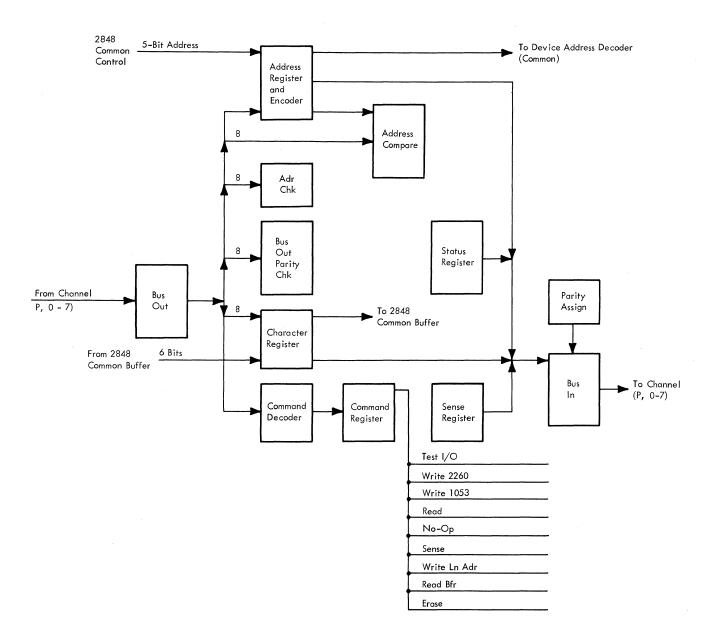
Figure 2-89. Channel Interface Controls
