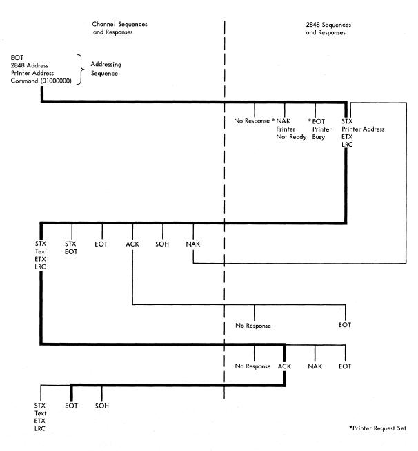
Figure 4-7. Sequence/Response Diagram - Specific Poll to Printer
