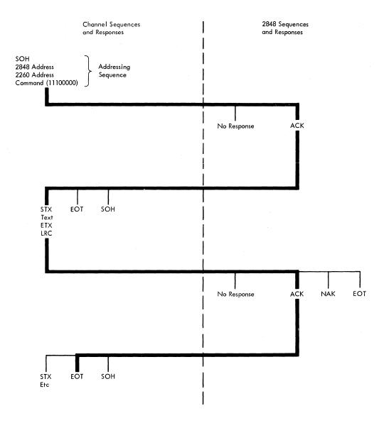
Figure 4-11. Sequence/Response Diagram - Erase/Write
