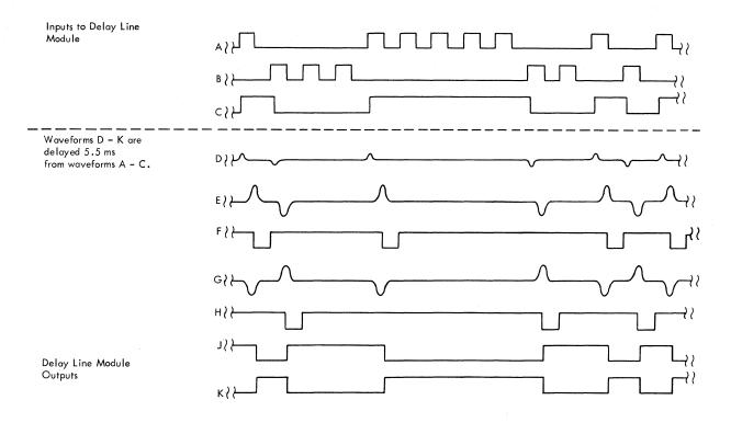
Figure 2-25. Delay Line Timing
