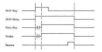
Figure 2-21. Keyboard Data Transfer Timing
