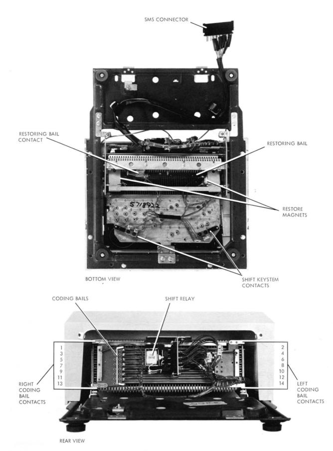
Figure 2-10. Alphanumeric Keyboard, Bottom and Rear Views
