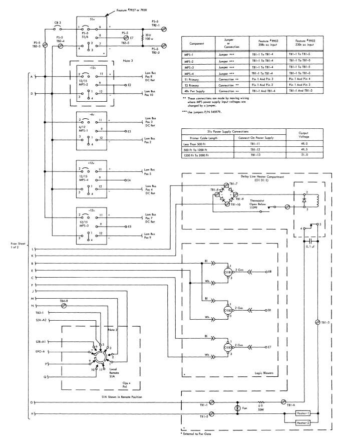
Figure 5-1. 60-Cycle Power Distribution and Control (Sheet 2 of 2)
