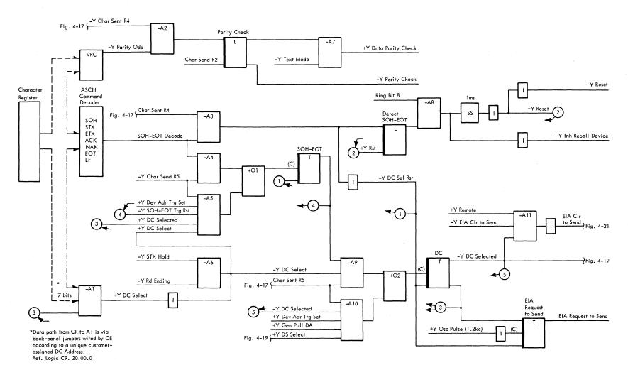
Figure 4-18. Channel Response, SOH-EOT and DC Address Characters
