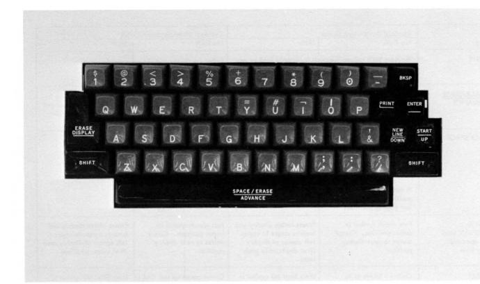
Figure 6-5. 2260 Display Station Alphanumeric Keyboard
