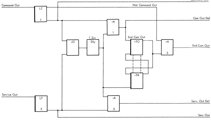
Figure 2-90. Out Tag Delays
