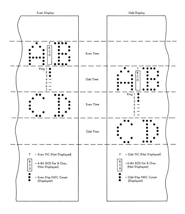
Figure 2-82. Display of NDC Cursor - Even and Odd
