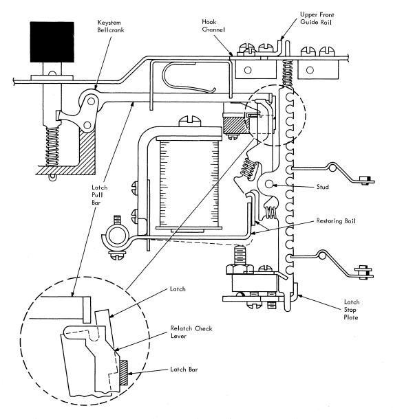
Figure 2-17. Key Position (Latched and Tripped)
