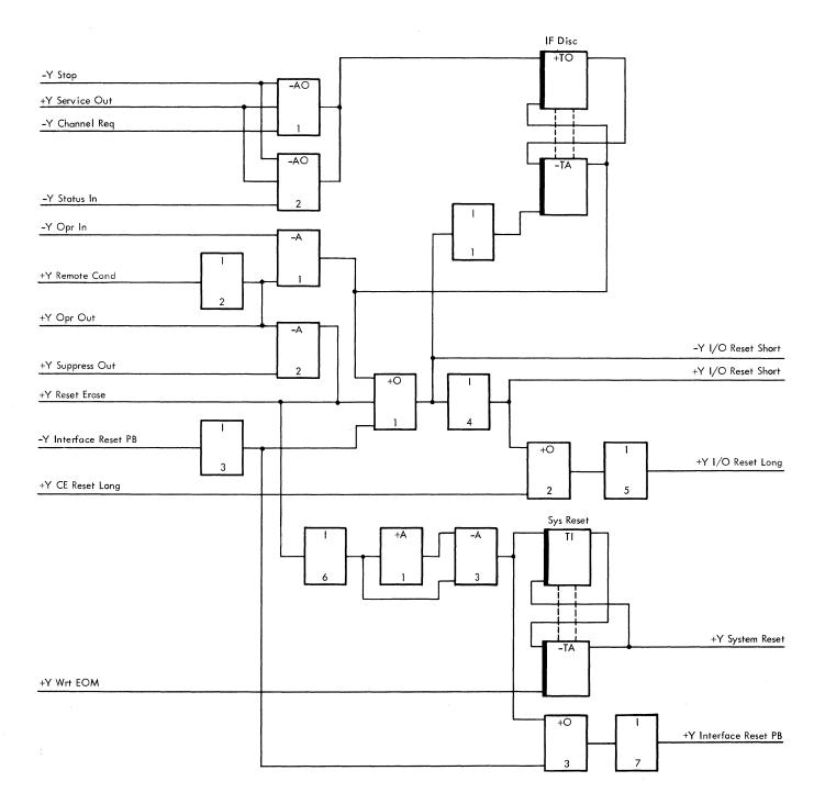
Figure 2-95. Disconnect and Reset
