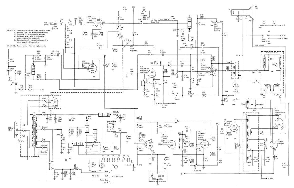
• Figure 2-7A. Display Station Electrical Schematic Diagram for DS Using Tube Adapters
