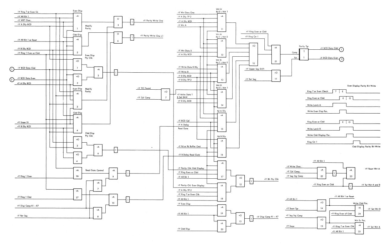
Figure 2-86. Parity Circuits
