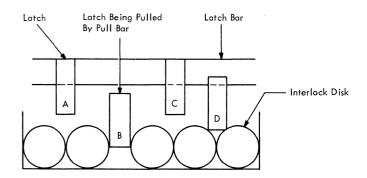
Figure 2-19. Interlock Disks (Partial)
