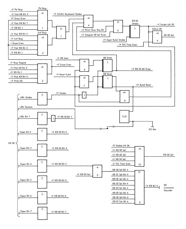
Figure 2-32. Keyboard Controls and Keyboard Data Bit Conversion and Gating
