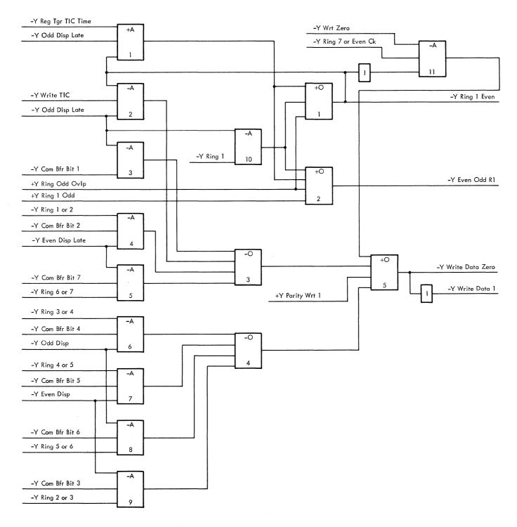
Figure 2-55. Serializer, A Delay
