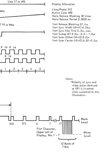
•Figure 2-9. Display Station Timing
