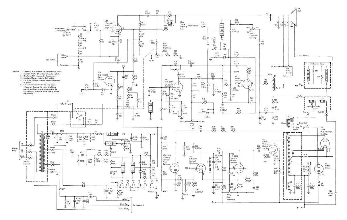
• Figure 2-7B. Display Station Electrical Schematic Diagram for DS Using Newer Level Circuit Boards.
