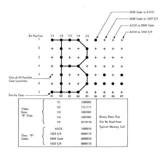
Figure 2-68. Generation of Binary Data from Memory Cell
