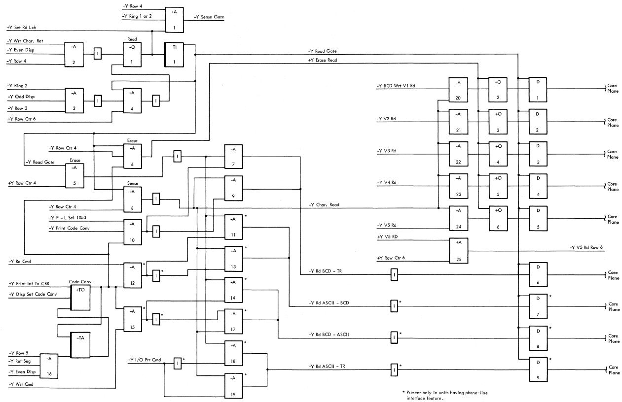
Figure 2-71. Character Generator Read Control Circuits
