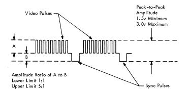
•Figure 2-2. Composite Video Signal (One Vertical Scan)
