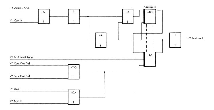
Figure 2-91. Address In Latch
