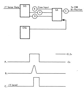
Figure B-4. Output Sense Level, and Sense Gate, Type FYZ
