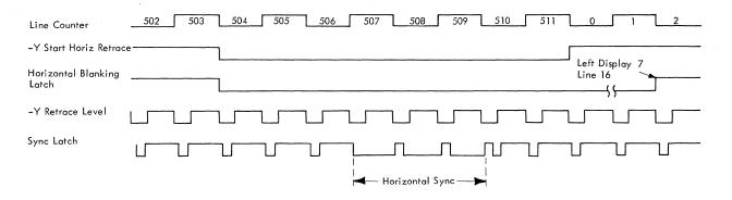
Figure 2-43. Sync Generator Timing
