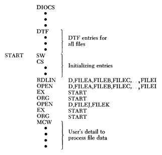
When this DIOCS entry is used, all OPEN instructions for *disk* files must be issued before the *Autocoder* loader is cleared. The *first* disk-file OPEN instruction must be issued before any *Autocoder* LTORG, EX, or XFR is issued.
