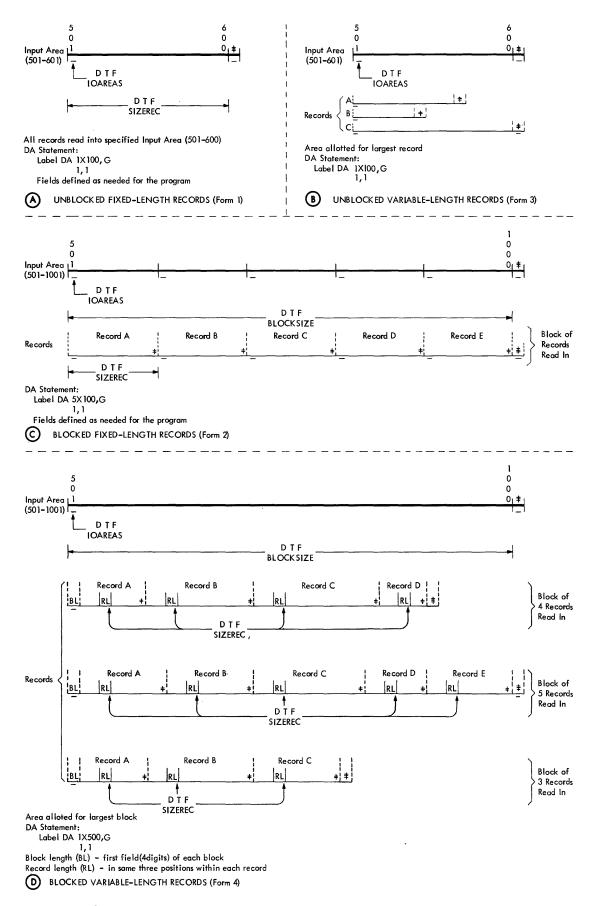
Figure 7. Schematic of Tape Records and Input Areas
