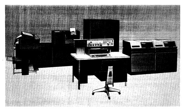
Figure 1. IBM 1440 Data Processing System
