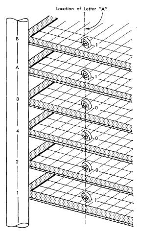
Figure 7. The Letter A Represented in Binary-Coded-Decimal Form in Core Storage
