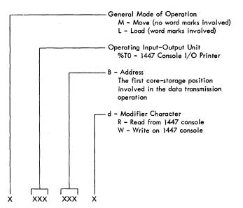
Figure 61. 1447 Console I/O Printer Instruction Format
