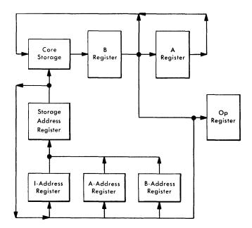
Figure 11. Processing Unit Registers
