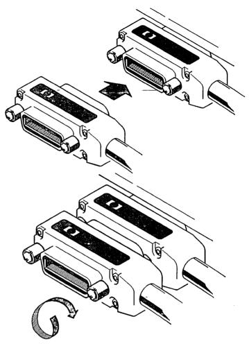
Figure 2-7. Stacking the Connectors.
