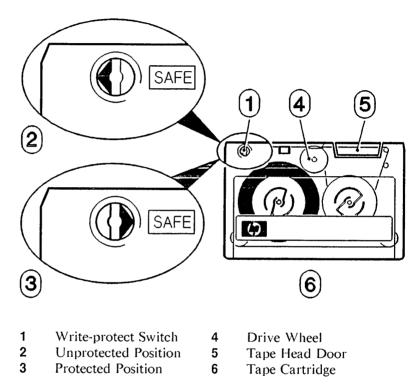
Figure 3-2. Write-protecting a Cartridge
