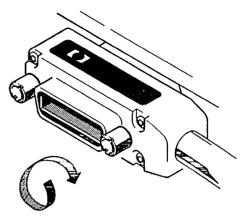
Figure 2-6. Tightening the Retaining Knobs.
