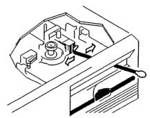
Figure 4-2. Cleaning the Tape Head.
