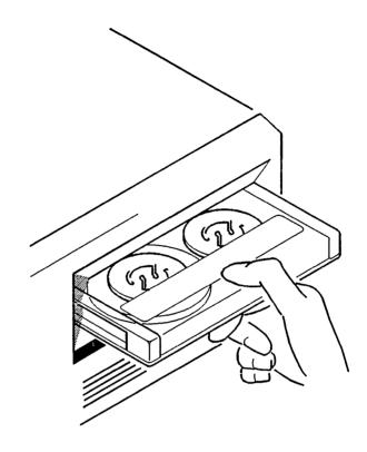
Figure 3-1. Inserting the cartridge
