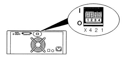
Figure 2-4. The Device Address Switches
