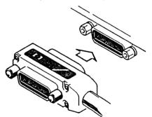
Figure 2-5. Fitting the HP-IB Cable.
