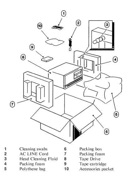
Figure 2-1. The Tape Drive, its Accessories and Packaging
