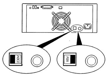
Figure 2-9. Voltage Select Switch.
