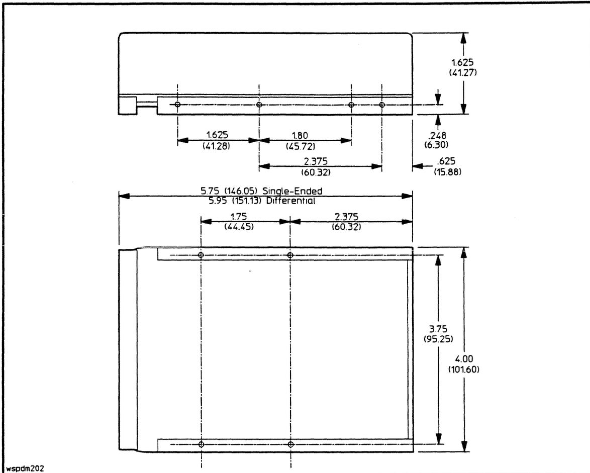
**Figure 2-3. Chassis Dimensions and Mounting Locations**
