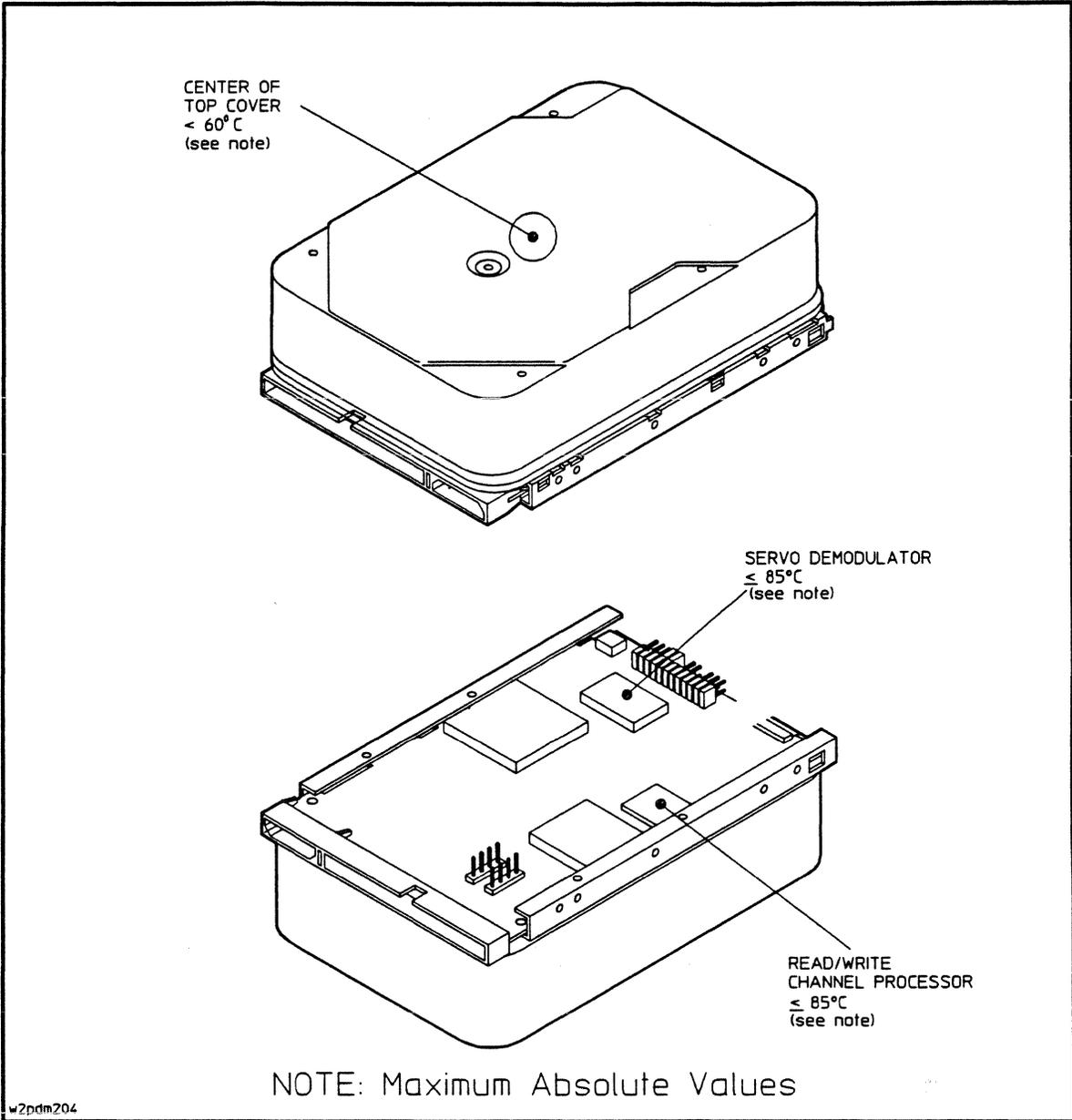
**Figure 2-4. HDA Temperature Measuring Points**
