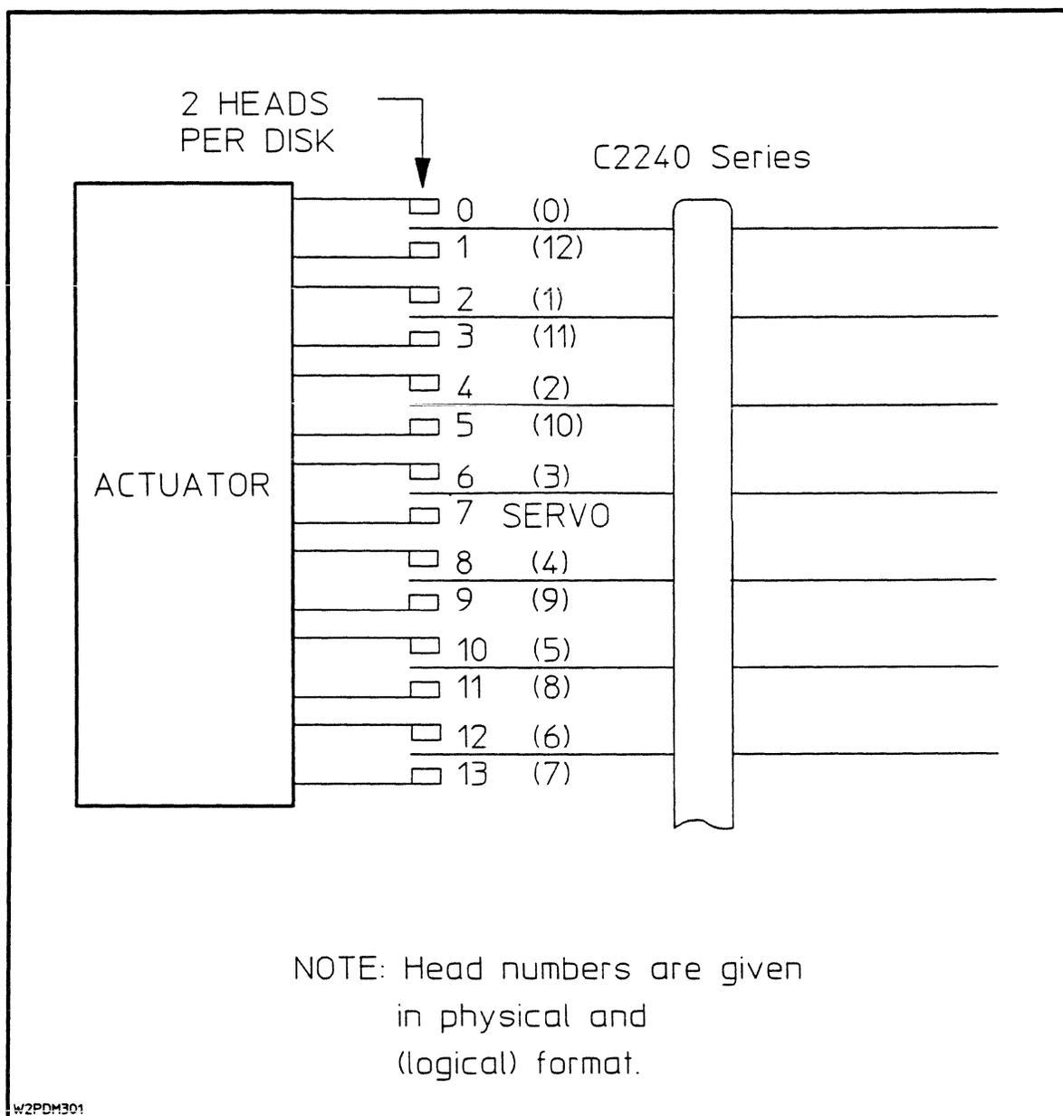
**Figure 3-1. Disk Drive Addressing Structure**
