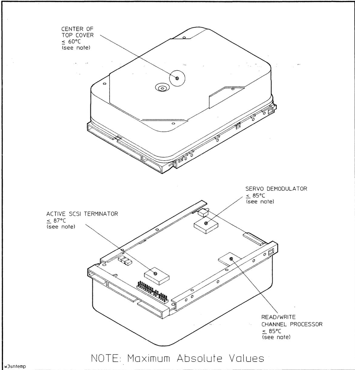
**Figure E-4. Narrow, Single-Ended: Temperature Measuring Points**
