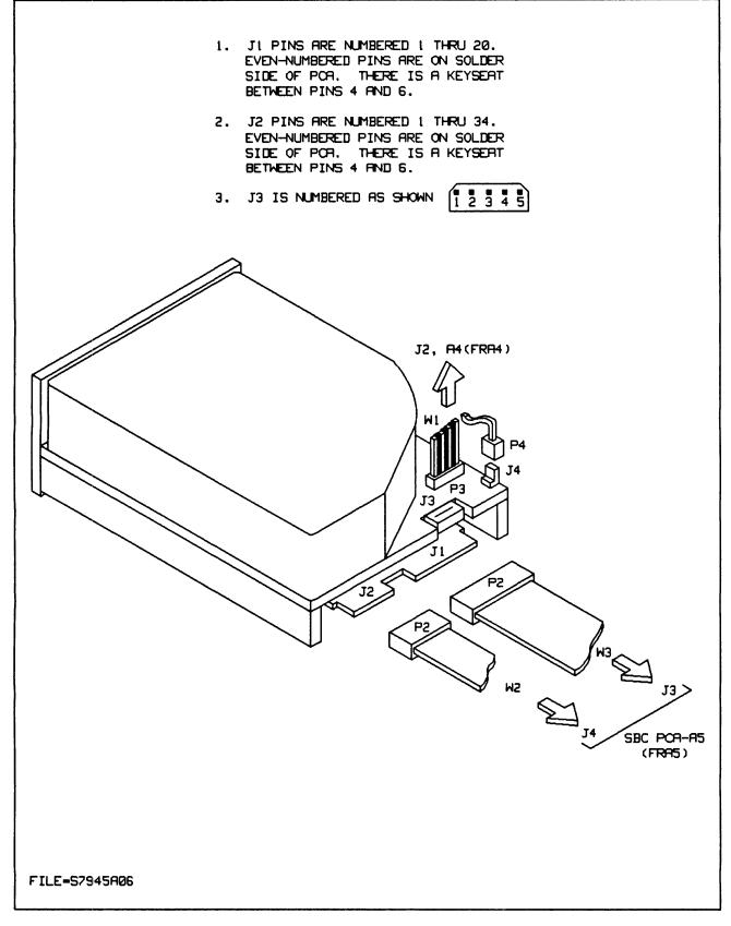
Figure 4-4. FRA1 (Disc Drive A1), Layout and Cable Connections
