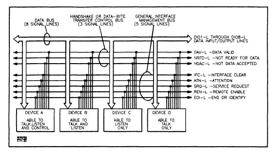
Figure 2-2. Hewlett-Packard Interface Bus Signal Lines
