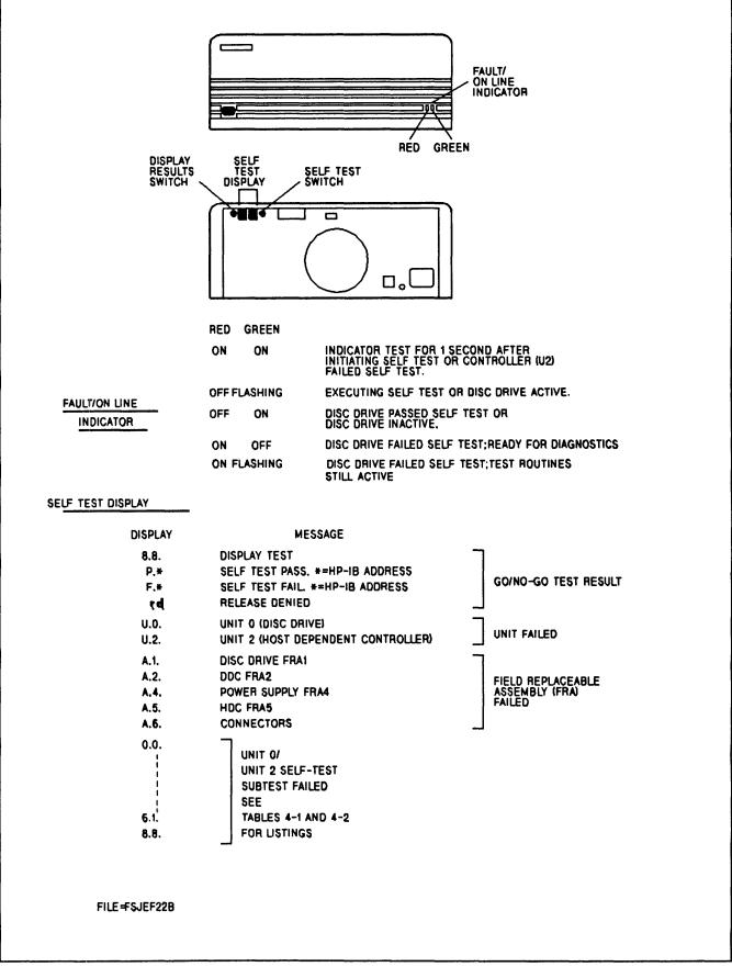
Figure 4-1. Self-Test Controls and Readout
