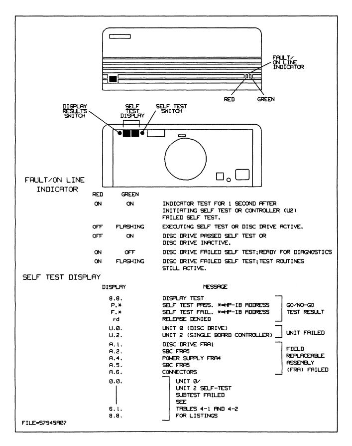
Figure 4-1. Self-Test Controls and Readout
