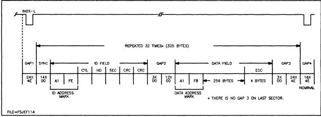
Figure 3-2. Track Recording Format
