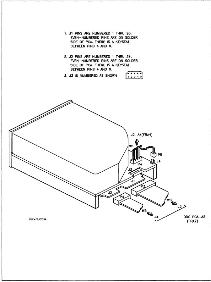
Figure 4-4. FRA1 (Disc Drive A1), Layout and Cable Connections
