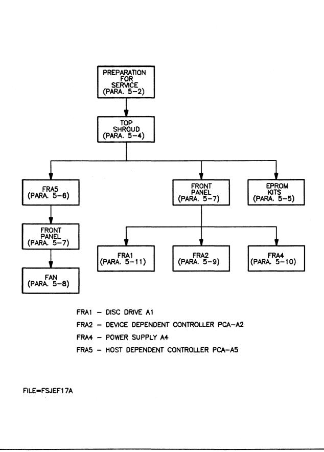
Figure 5-1. Order of Disassembly
