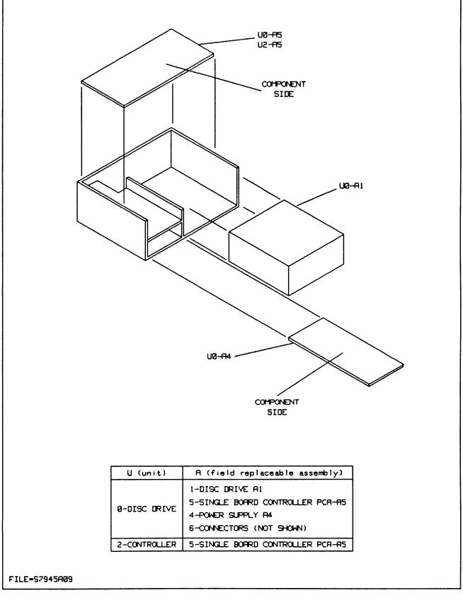
Figure 4-3. Field Replaceable Assembly (FRA) Locations
