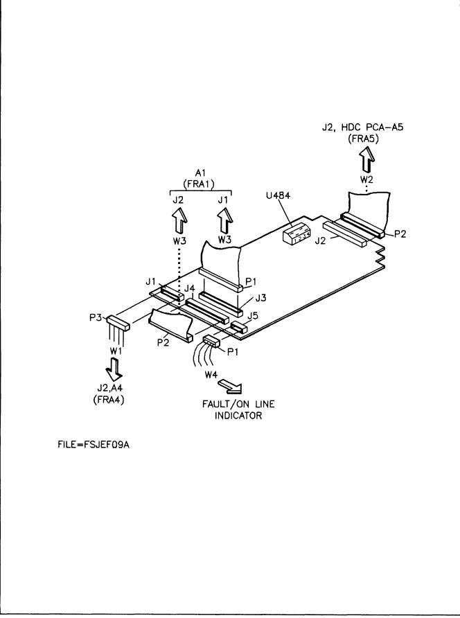
Figure 4-5. FRA2 (DDC PCA-A2), Layout and Cable Connections
