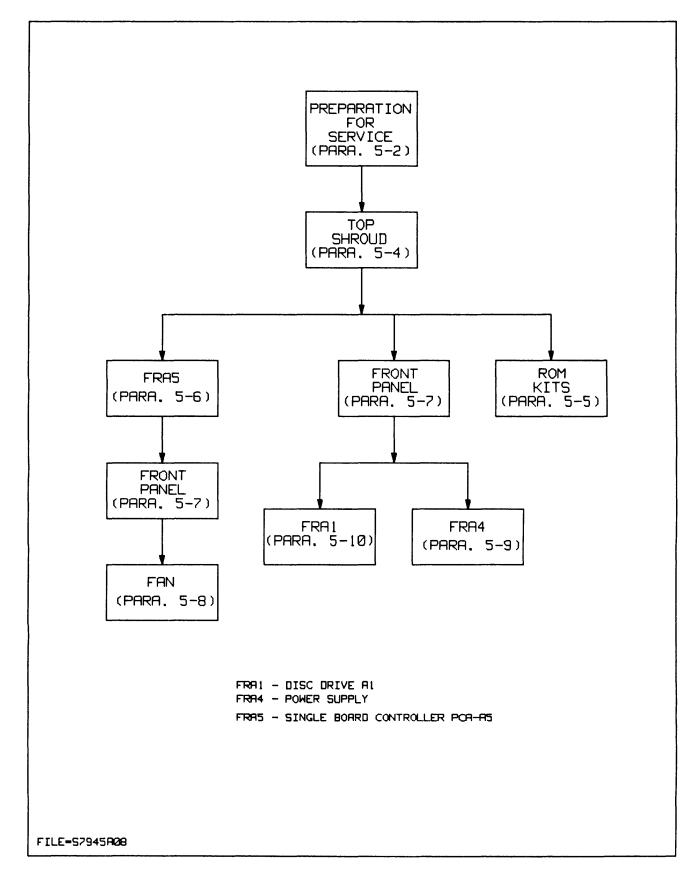
Figure 5-1. Order of Disassembly
