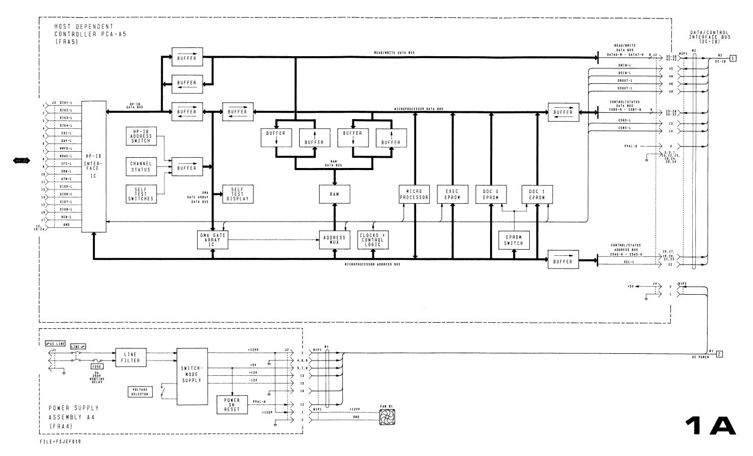
Figure 3-4. Disc Drive, Functional Block Diagram, (Sheet 1 of 3) B3-31/B3-32
