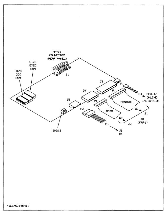
Figure 4-6. FRA5 (SBC PCA-A5), Layout and Cable Connections
