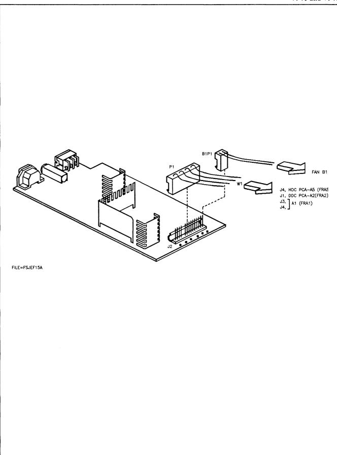
Figure 4-6. FRA4 (Power Supply A4), Layout and Cable Connections
