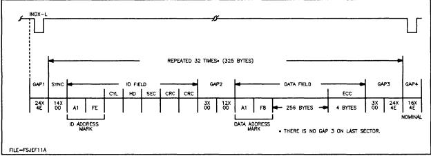
Figure 3-2. Track Recording Format
