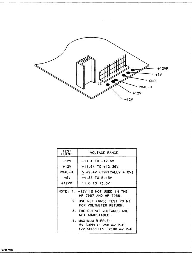
Figure 4-4. Power Supply (PCA-A3) Test Points and Voltages
