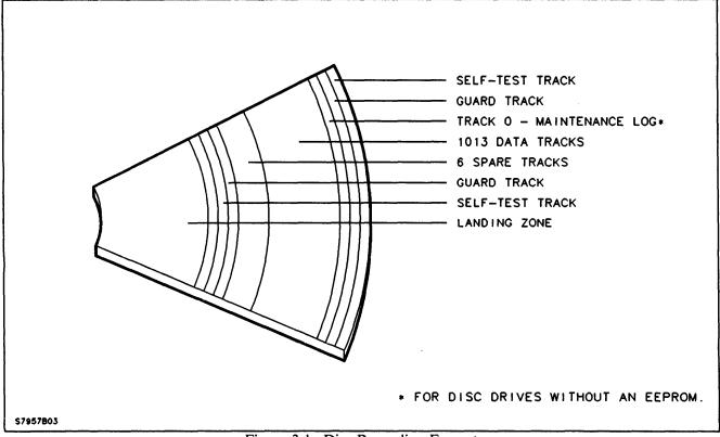
Figure 3-1. Disc Recording Format
