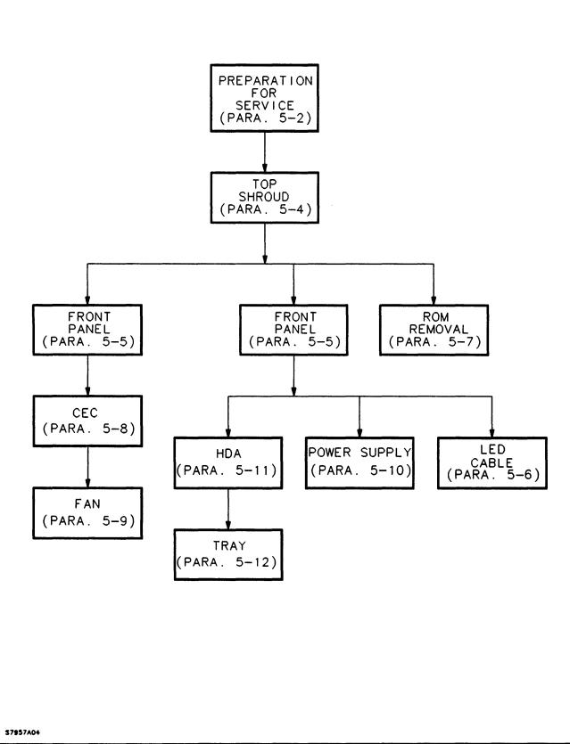
Figure 5-1. Order of Disassembly
