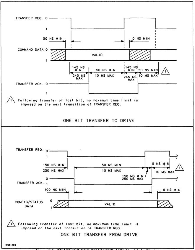
Figure 2-5. TRANSFER REQ/TRANSFER ACK Handshake Timing
