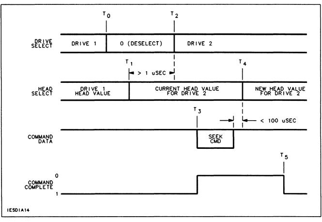
Figure 2-8. Recommended Drive/Head Selection Sequence
