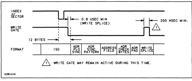
Figure 2-2. Write Gate Timing During Format
